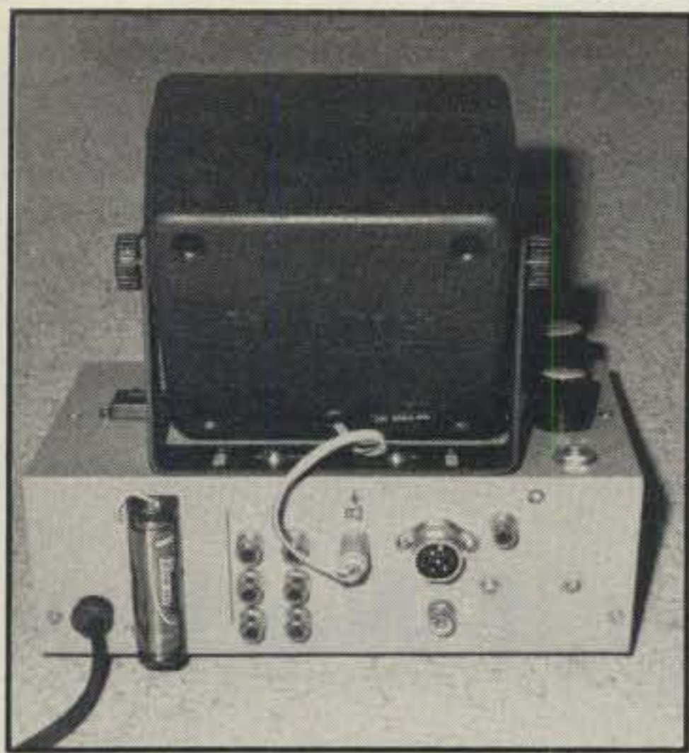
A rear view of the larger "CCC." Liberal use is made of phono jacks for external connections. The battery to the left is a holder for the LCD clock only.
