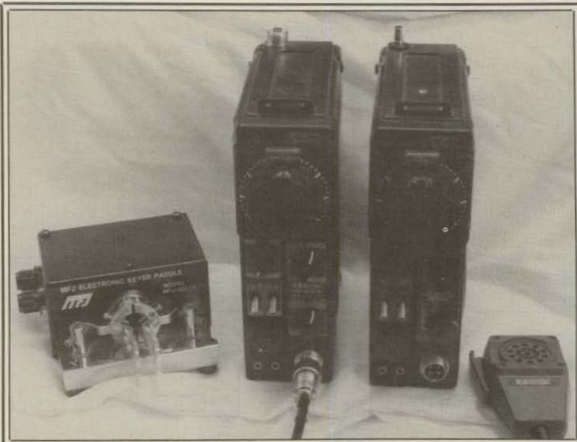
Fig. 4— Here's an authentic example of OSCAR 10 on a budget. Older style and inexpensive SSB/CW transceivers for 2 meters and 70 cm form a basis upon which an RF amplifier and preamplifier is added. Matching 2 meter and 70 cm antennas complete the setup.
