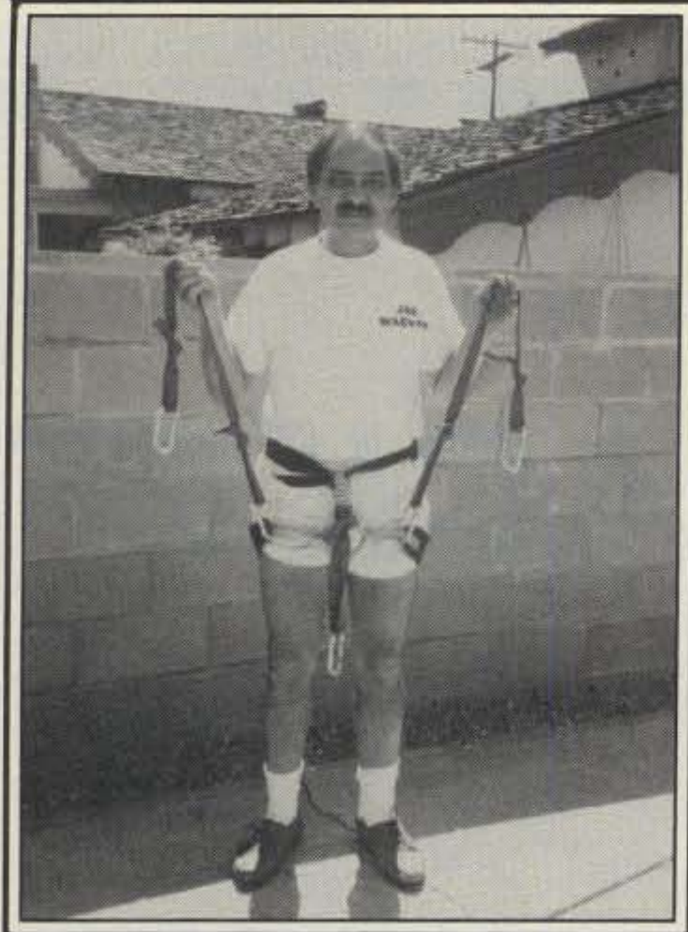
The front view of the harness showing how it is worn. The right and left webbing (with carabiners) attaches to the tower or around the tower.
