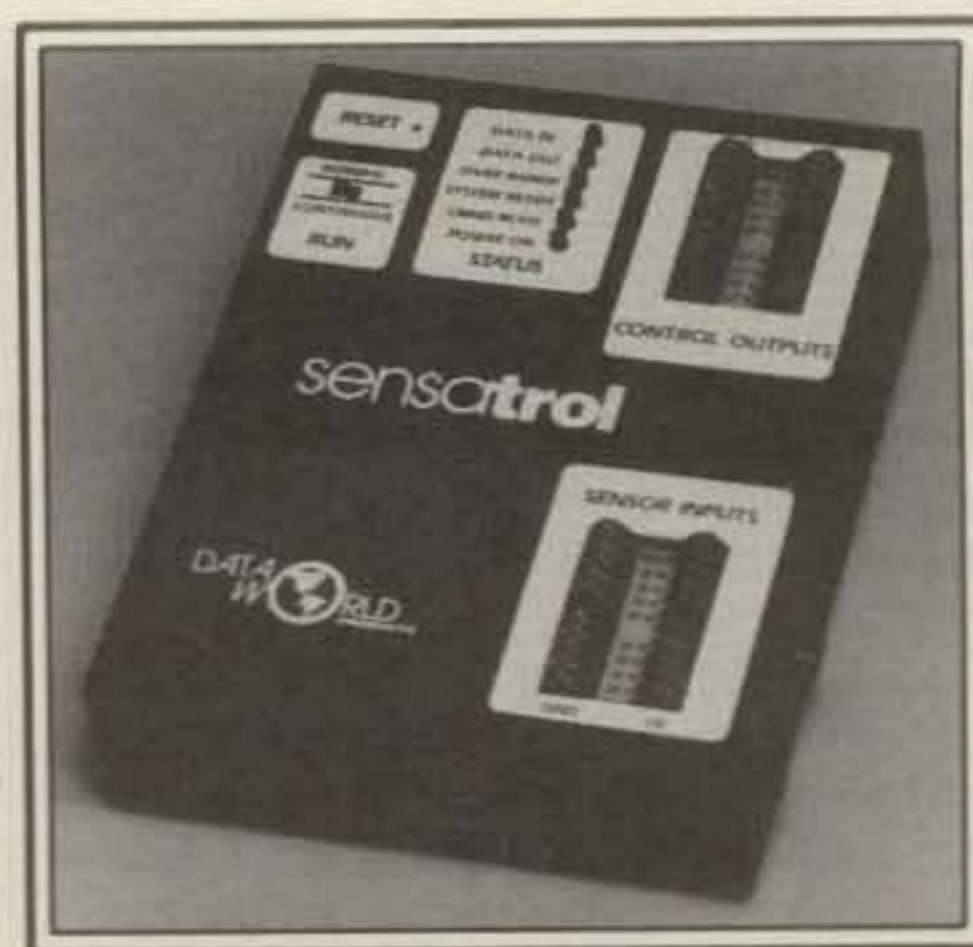
The Sensatrol interface provides a good example of the kind of linking that's possible between your personal computer and the environment. The device is a digital sensor/controller which directly interfaces with any PC that has an RS232C port. A variety of measurement and control applications are possible. (Photo courtesy Data World Products)
