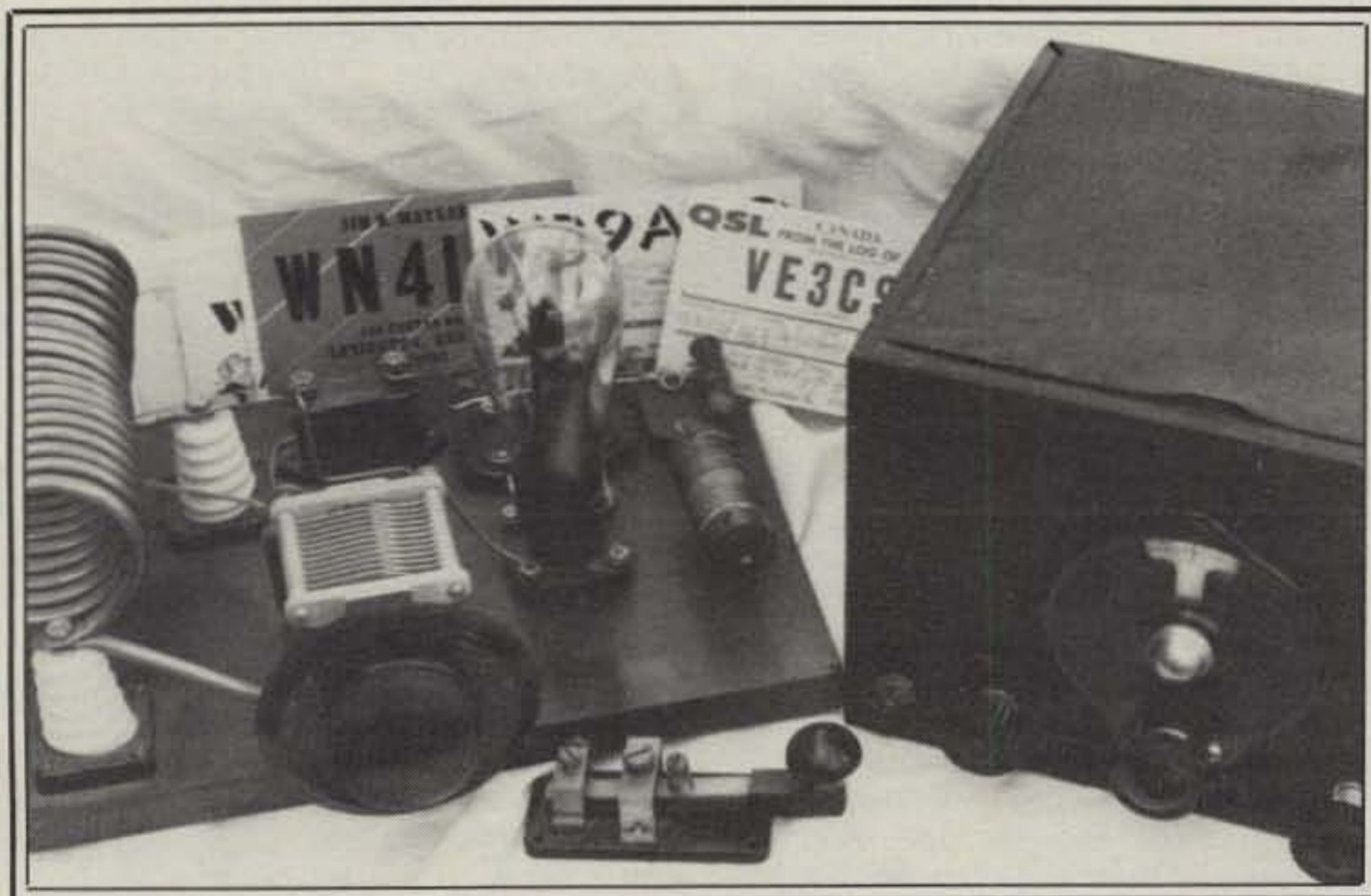
Fig. 10- Full classic setup featuring SW-3 and TNT transmitter. This 10 watt rig has worked over 10 countries on 80 meters since 1984.
