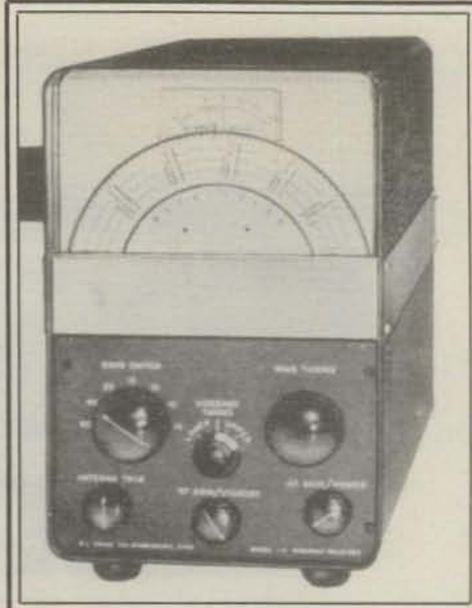
Fig. 6- R.L. Drake's classic 1-A receiver reflected a radical change in cabinet designs, but its performance quickly became an accepted "standard of reference." S-meter is recessed behind main dial, speaker is mounted on cabinet's rear wall, and push/pull, on/off switch is on RF gain control.
