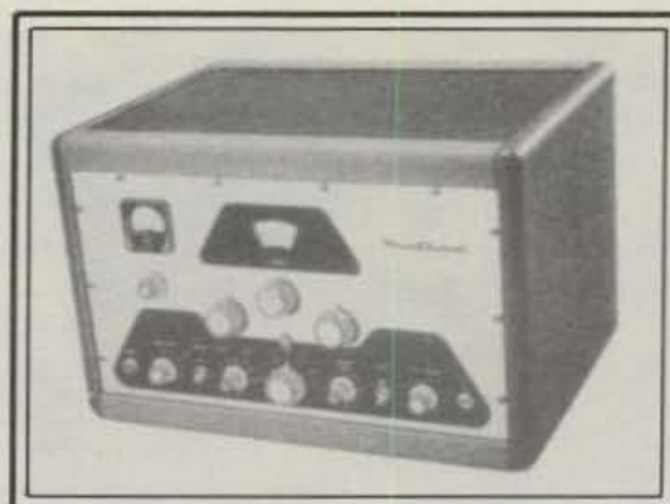
Fig. 4- Heathkit's "Battle Cruiser" of the HF bands: The legendary DX-100. This unit was a DXer's dream come true, and its 125 watts output could literally "work the world"!
