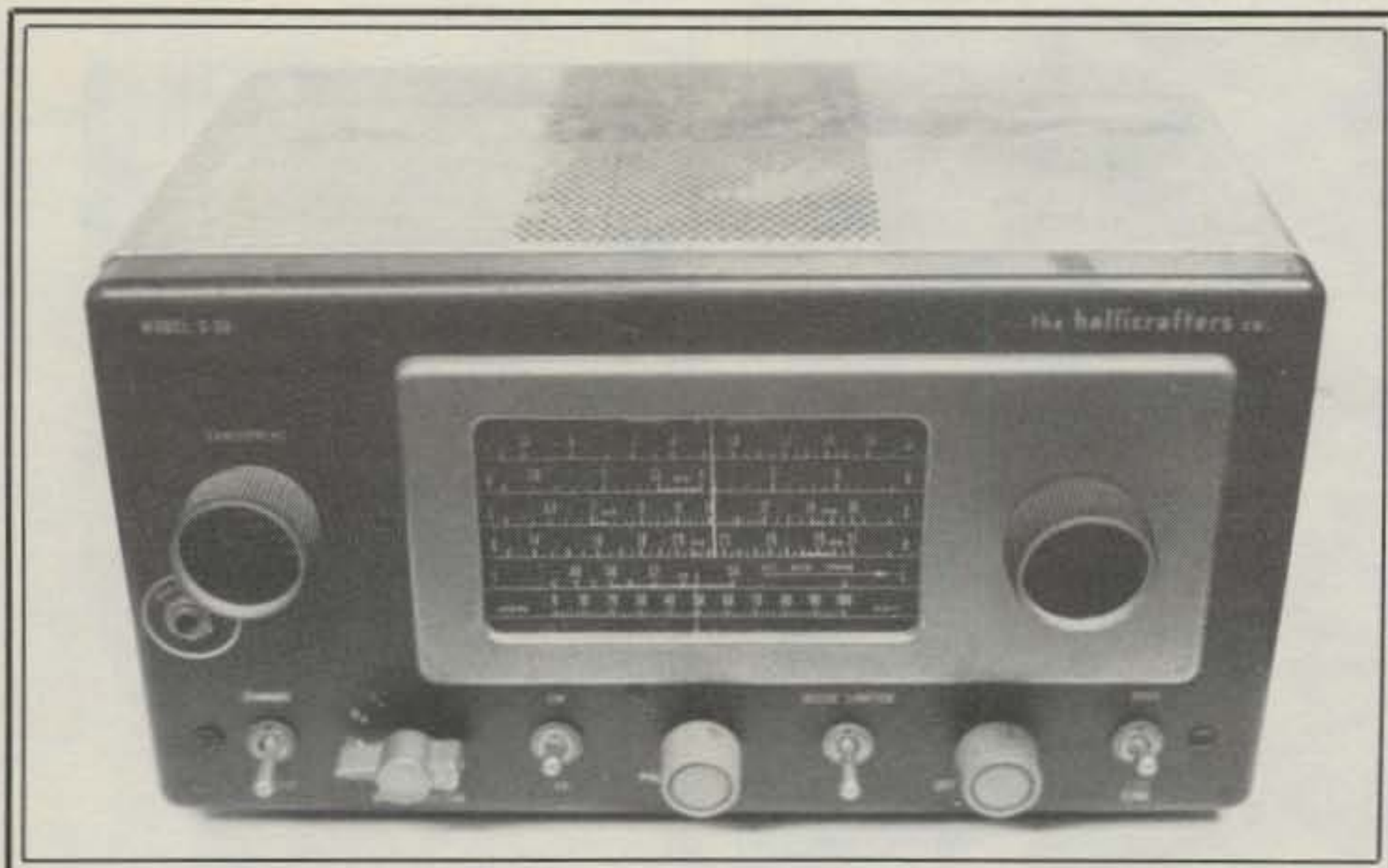
Fig. 3- Another economy champ from Hallicrafters during the 1950s was the S-53. Noteworthy points of this receiver were its ability to actually copy 15 and 10 meter signals, and dial-cord restringing problems that could drive one right up the wall.
