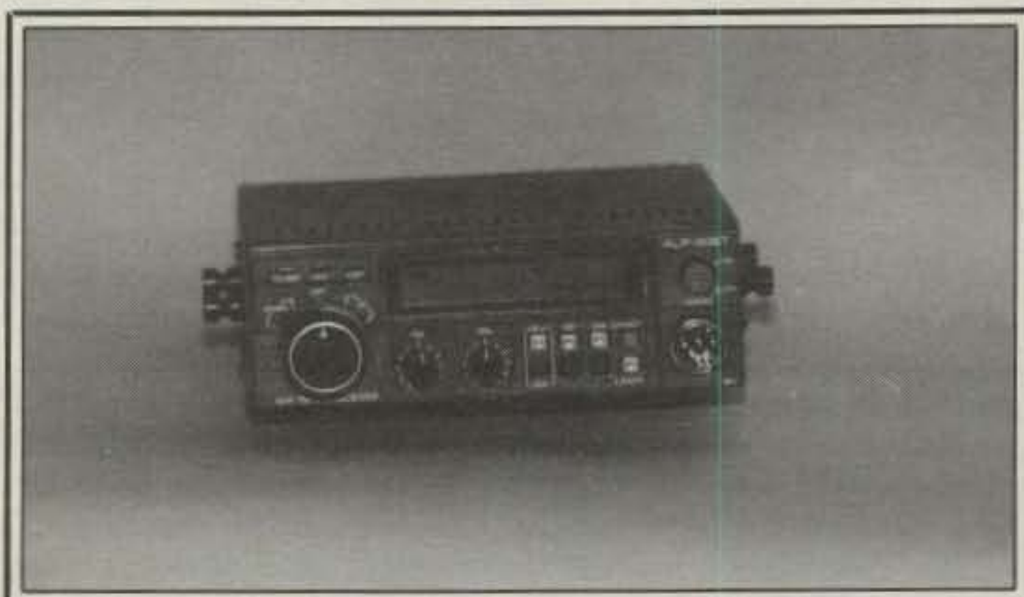
The new Alinco ALR-206T is small but powerful, delivering 25 watts output across the entire band. Uncluttered front panel is the result of a design that puts the majority of the operating controls right into your hand.
