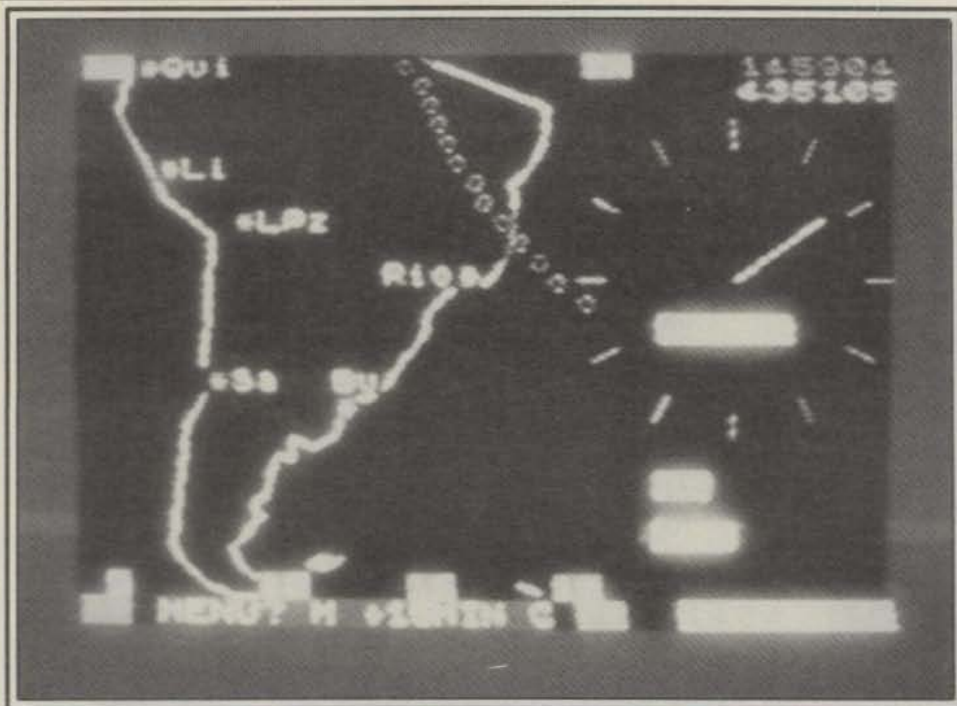
Even the smaller, less-expensive computers such as the Timex-Sinclair Series have good potential for amateur radio applications. Shown here is one of the "mission control panels" from the GM4IHJ satellite tracking program for the Timex 2068 or Sinclair Spectrum computers. (Photo via WA6DLI)
