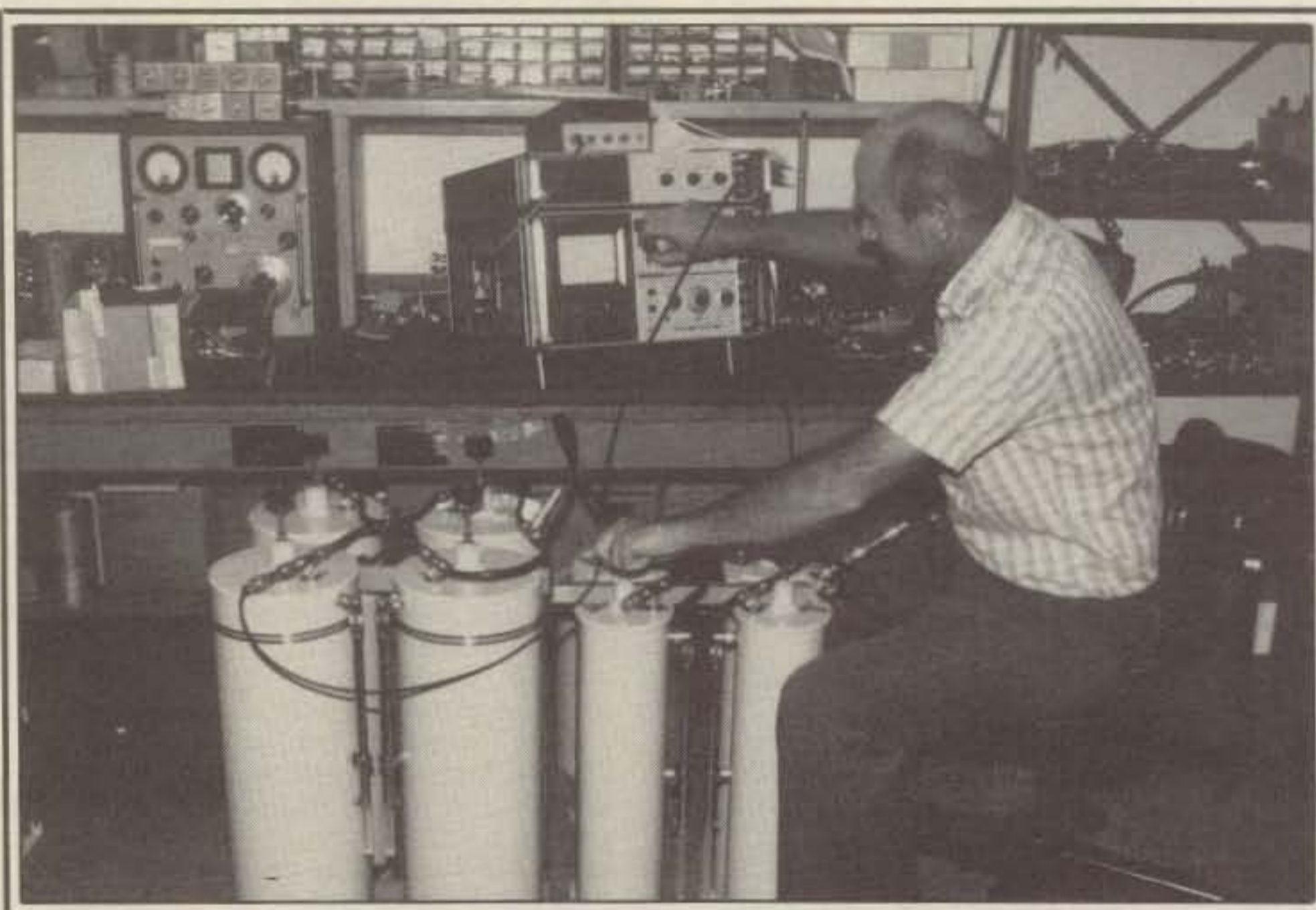
Lloyd Alcorn of WACOM is shown putting the finishing touches on a duplexer.
