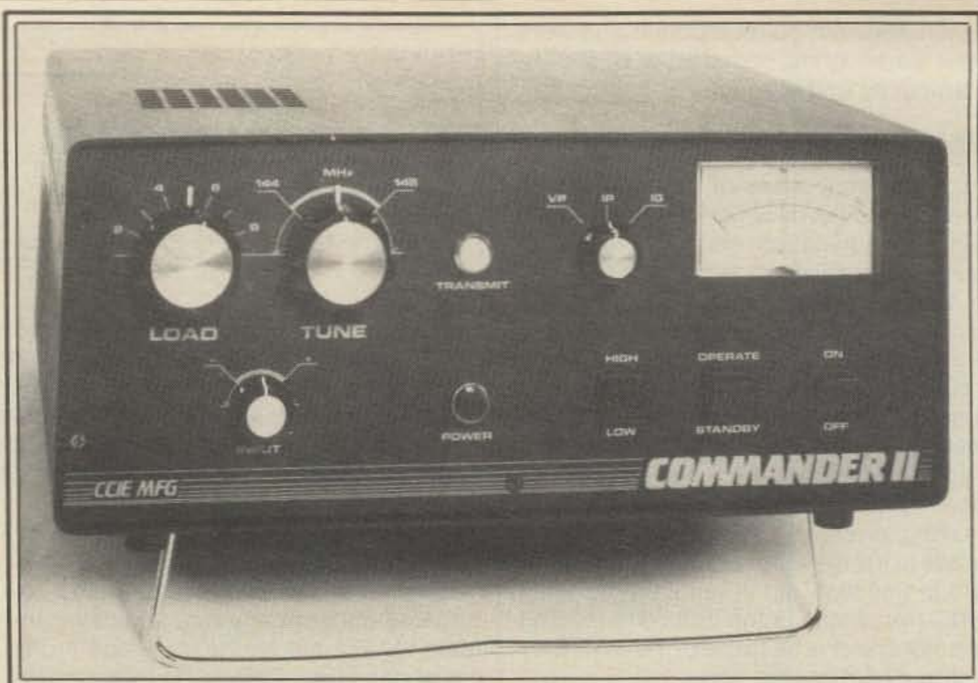
The C.C.I.E. Commander II 144 MHz kilowatt power amplifier is rated at 650 watts RF output with just 15 watts drive.
