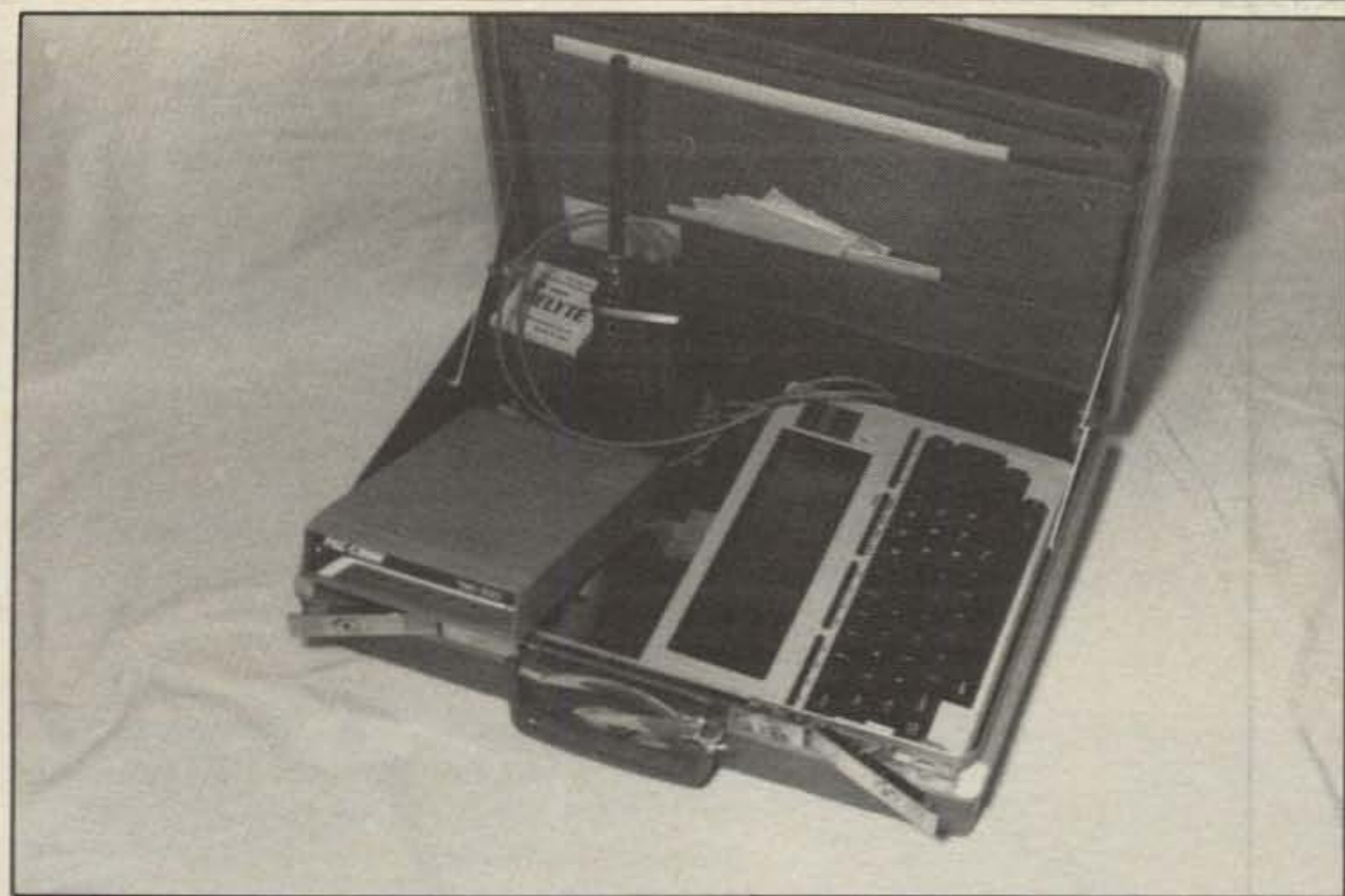
A complete portable packet station in a briefcase consisting of a TRS-80 Model 100 portable computer, a Pac-Comm TNC-200, and IC-02AT, and a gel cell battery.
