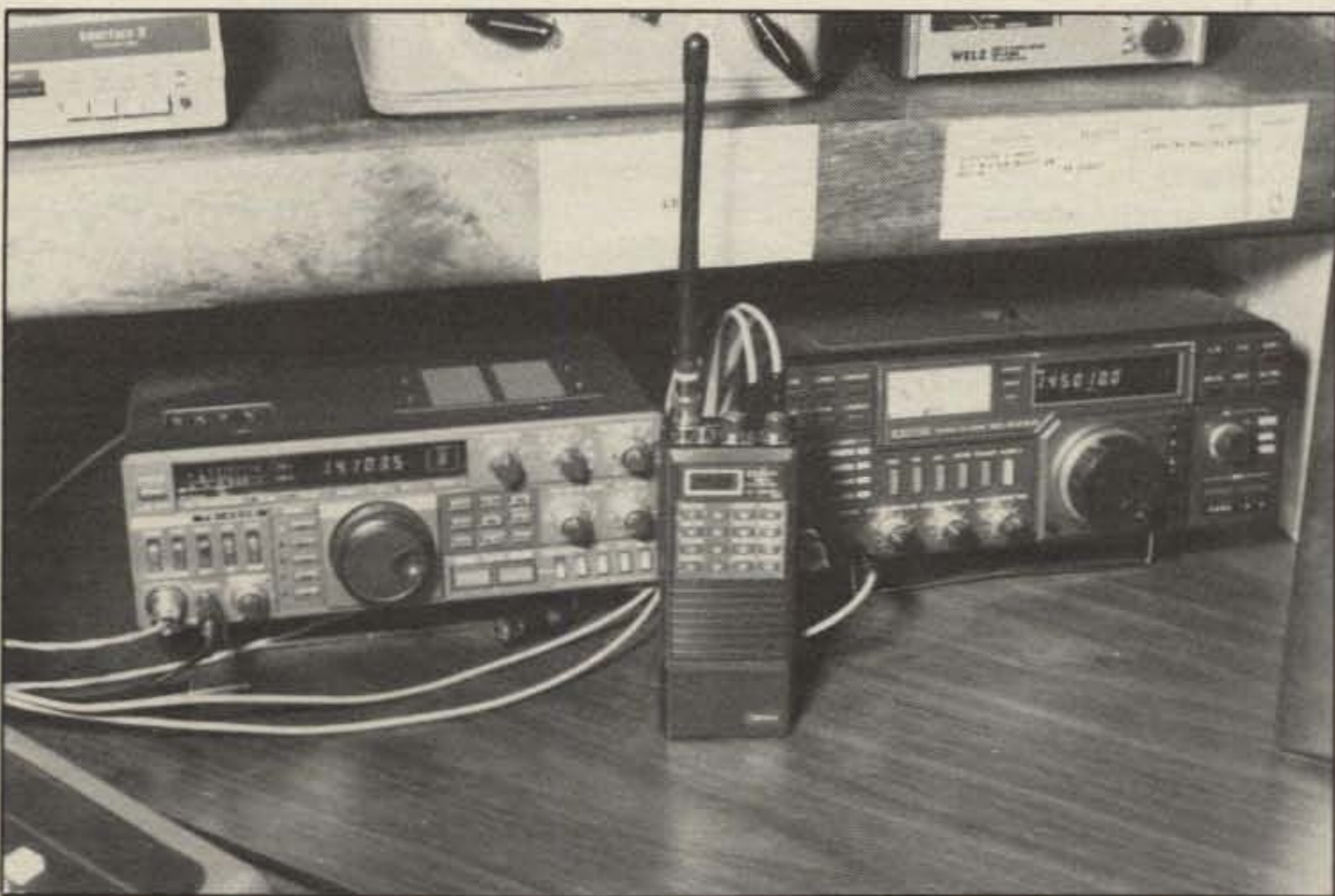
The radio equipment at KR3T. A Kenwood TS-430S is used on HF, an ICOM 271-A is used for 2 meter base operation, and an IC-02AT HT is used for portable operation.
