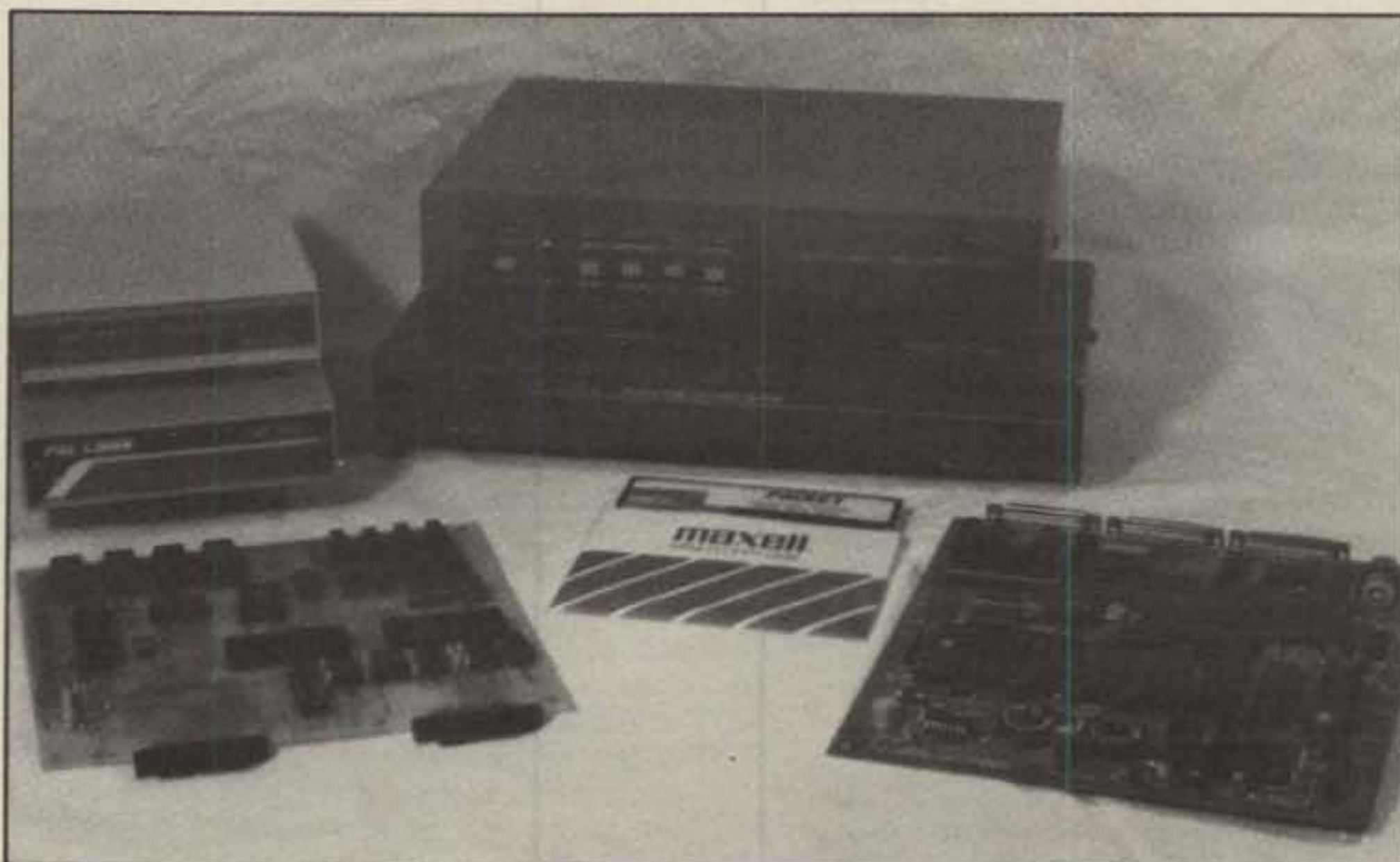
Assorted TNCs. Clockwise from the bottom: the original VADCG TNC, the Pac-Comm TNC-200, the Kantronics KPC-2, the AEA PKT-1, the Heathkit HD-4040, and the VADCG TNC+. The disk contains the Richcraft AX.25 TNC software system.
