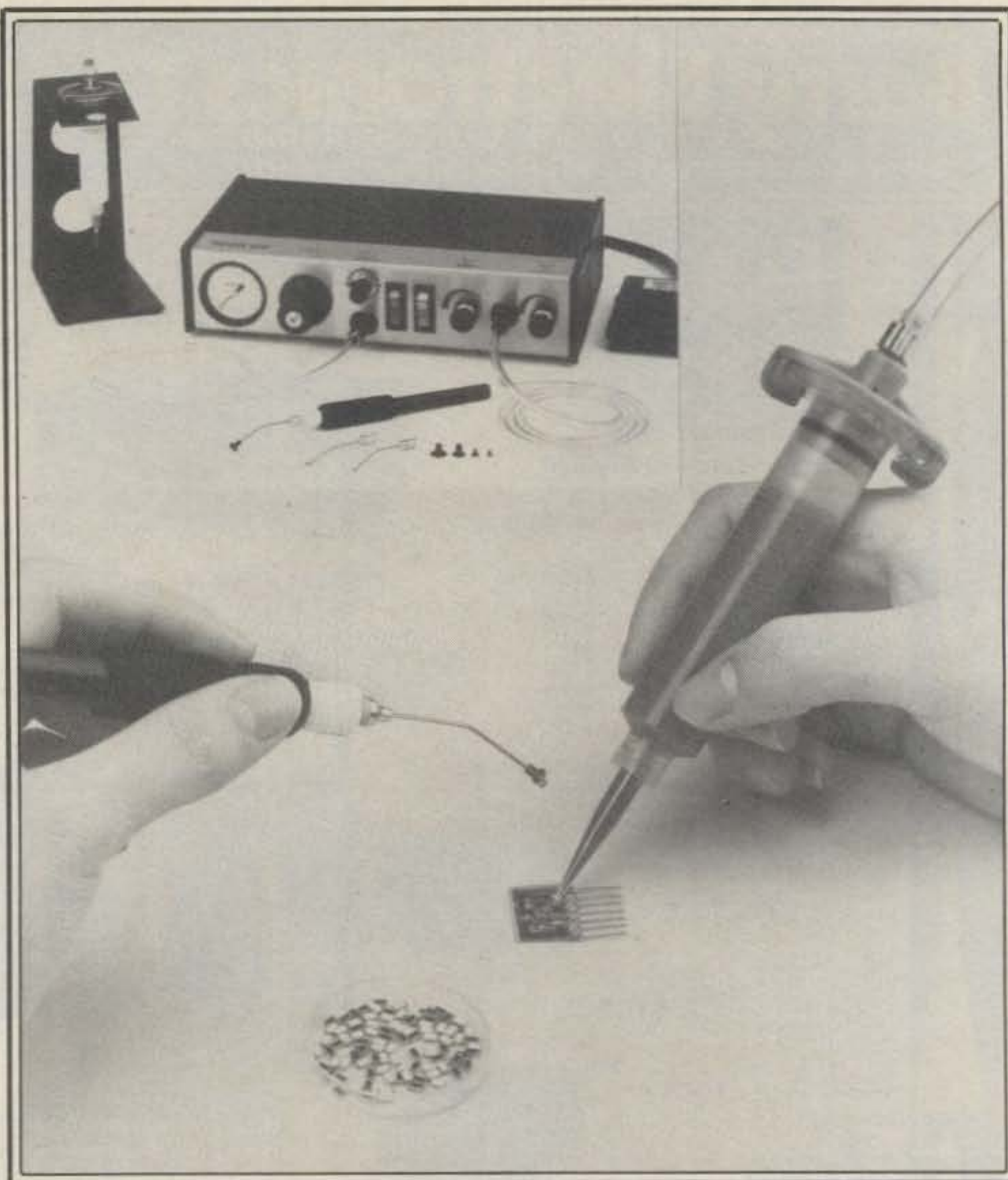
Fig. 13— An instrument that automatically dispenses liquids such as solder creams and holds components as well.
