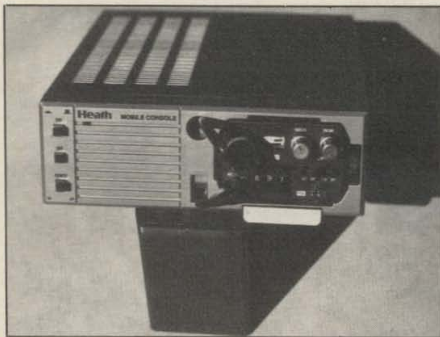
This is the mobile console. The handheld battery pack is removed and the transceiver inserted into the console. Connections are then made for audio and RF.
