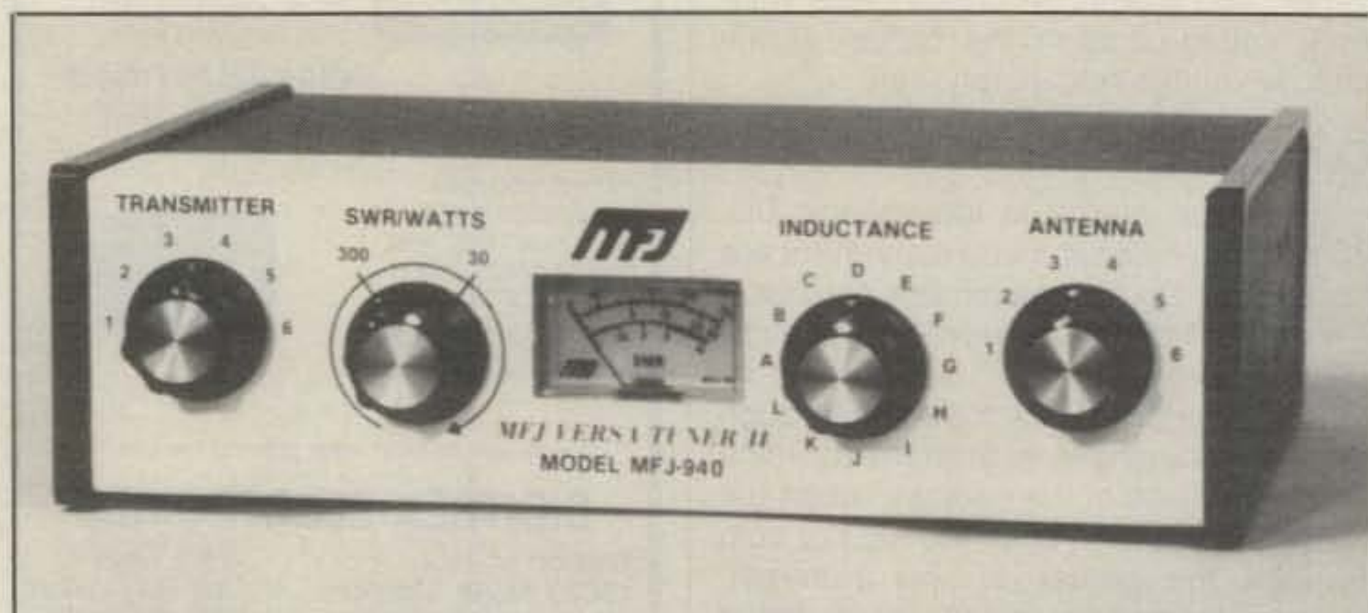
Although Zepps are sometimes fed by coax via an impedance-transforming balun, in most cases openwire is run to the hamshack, where an antenna tuner/transmatch is used to couple to coaxial cable. (Photo courtesy MFJ Enterprises)
