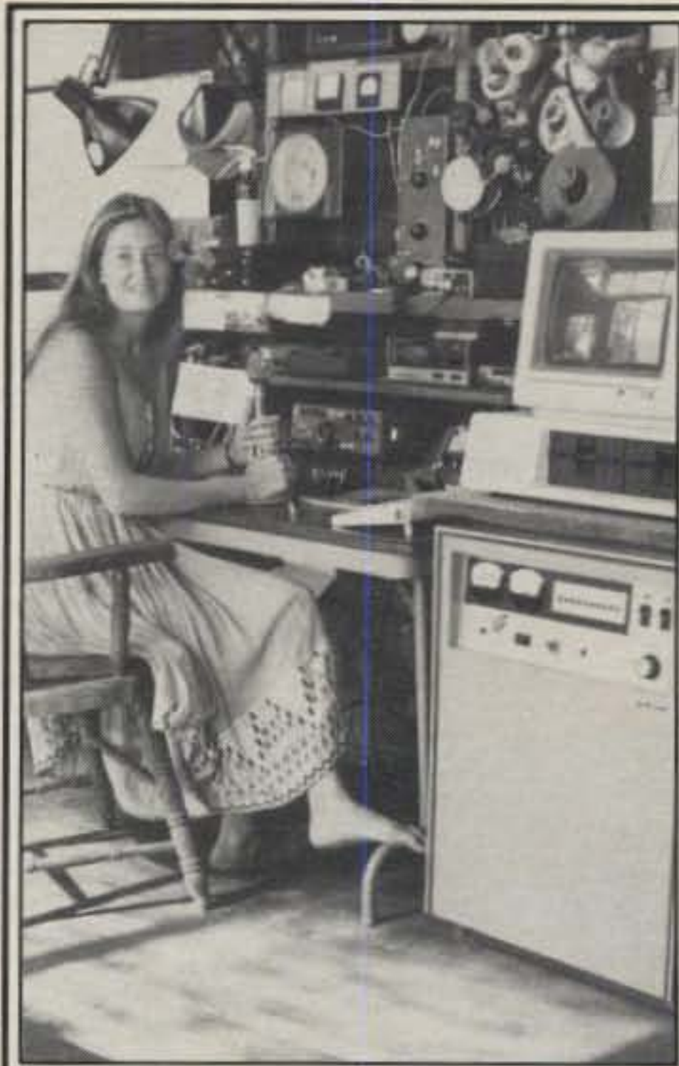
Helen, AH6GQ, at the mike of her unique station. The amp is powered by a 2.5 kw gas generator, and the other equipment is powered by windmills and a hydroplant. No commercial electricity is available at her QTH.
