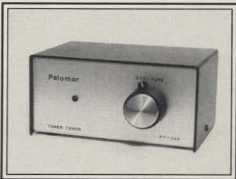
Palomar Engineers Model 340 Tuner Tuner is an unusual accessory that allows you to "tune your antenna tuner" without transmitting. It contains a noise bridge and the necessary switching and protection circuitry to allow its "on the air" insertion between the transceiver or transmitter and antenna tuner. (Photo courtesy Palomar Engineers)
