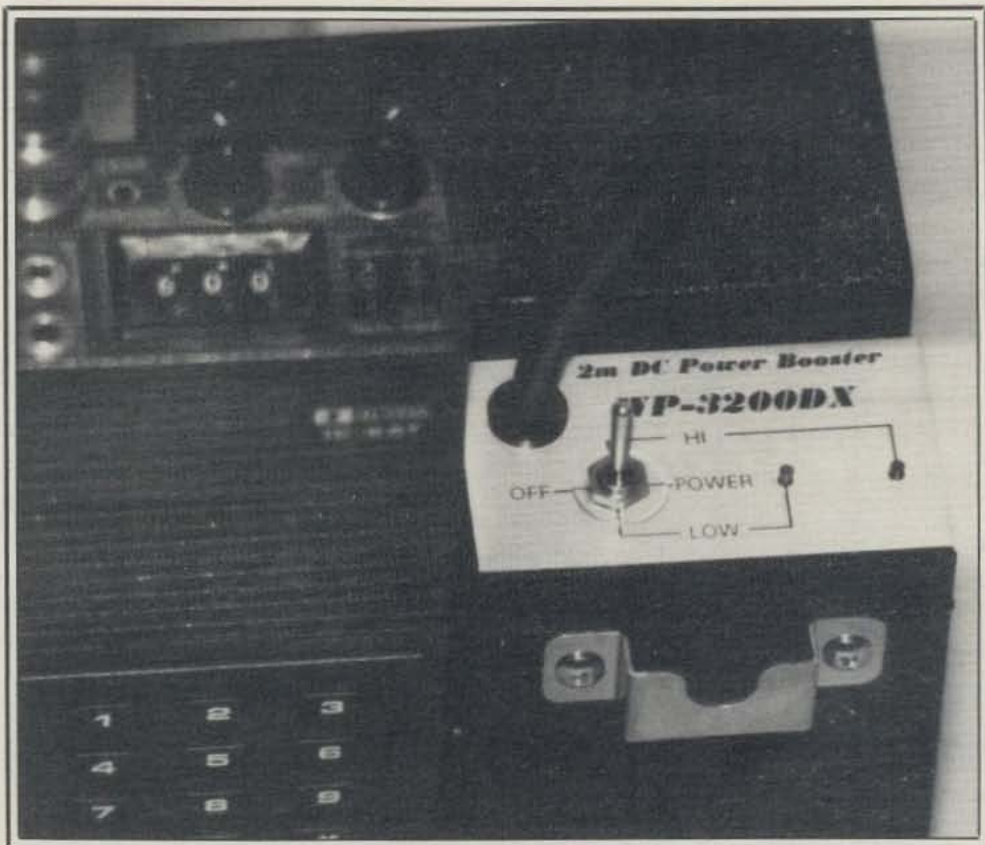
The WSE WP-3200DX "Docking Booster" has a simple control panel, with just a low-off-high switch. The handie-talkie is inoperative when the Docking Booster is switched "off," and the RX preamp is active at all times.
