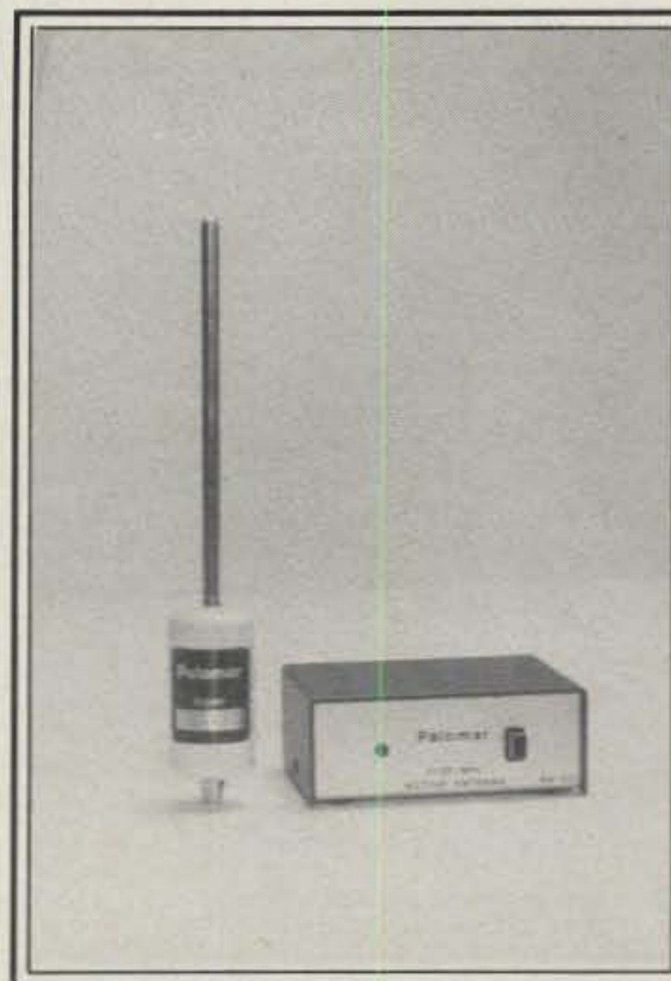
The Palomar PA-351 3-30 MHz Active Antenna should be of interest to CQ readers who are also active SWLs. The unit has a claimed noise figure of 2.5 dB and a gain of 20 dB. The 36 inch probe may be mounted in a high location far from manmade noise, up to 200 feet from the control unit. (Photo courtesy Palomar Engineers)
