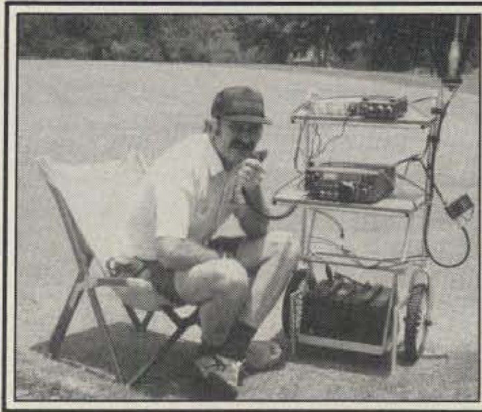
It is true that some DXers never want to wander far from the rig, and even in Lima, Peru, DXers have learned that eternal truth. Here is Carlos Siewczynski, OA4CIT, right at the edge of a sand trap on a golf course, but ready to work a needed one between putts. The gear includes an ICOM 740 with a couple of 12V batteries for power. The antenna is a Hy-Gain mobile.
