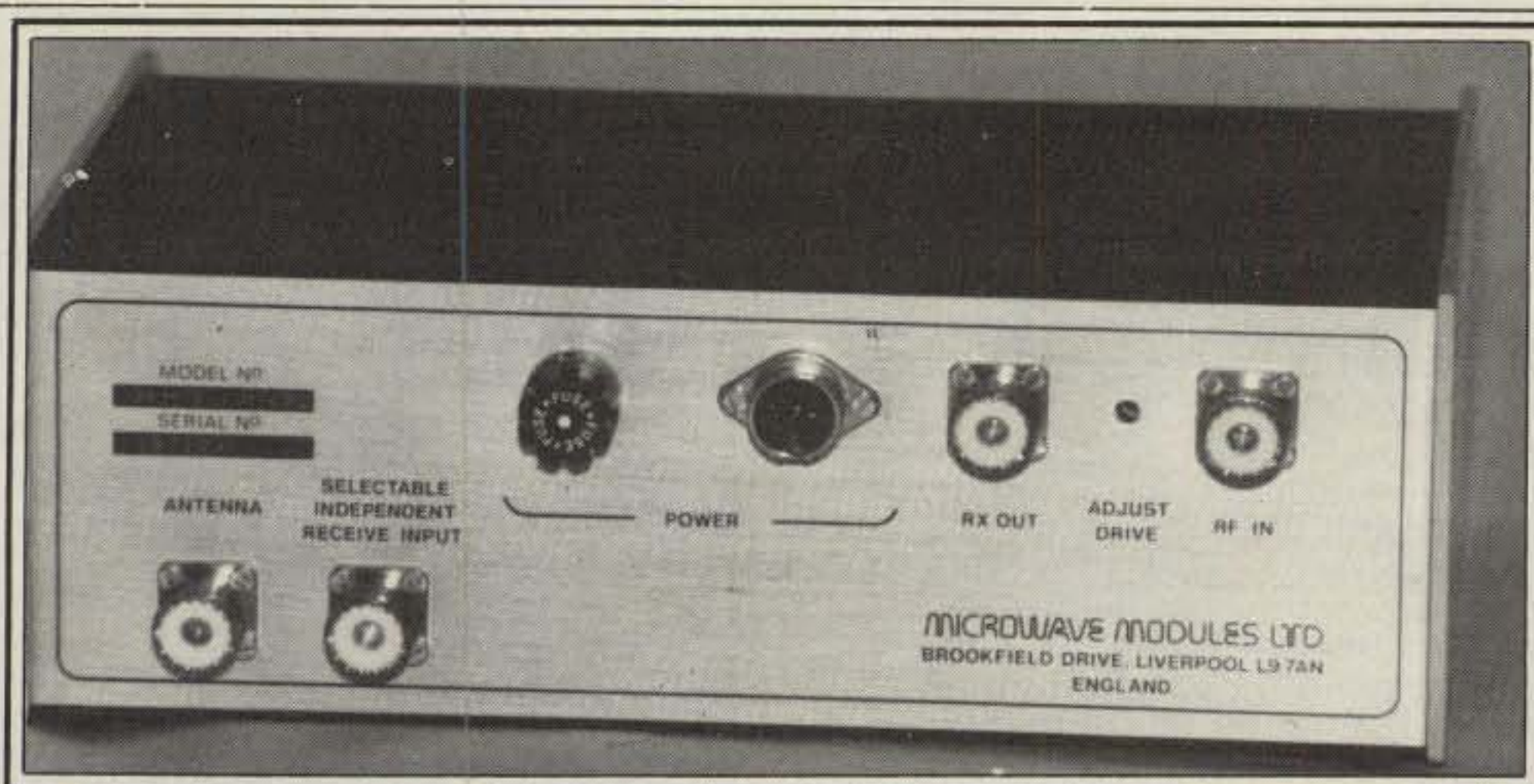
MMT50/28S rear view: fuse holder, power receptacle, all input and output jacks, and RF drive adjust are within easy reach.
