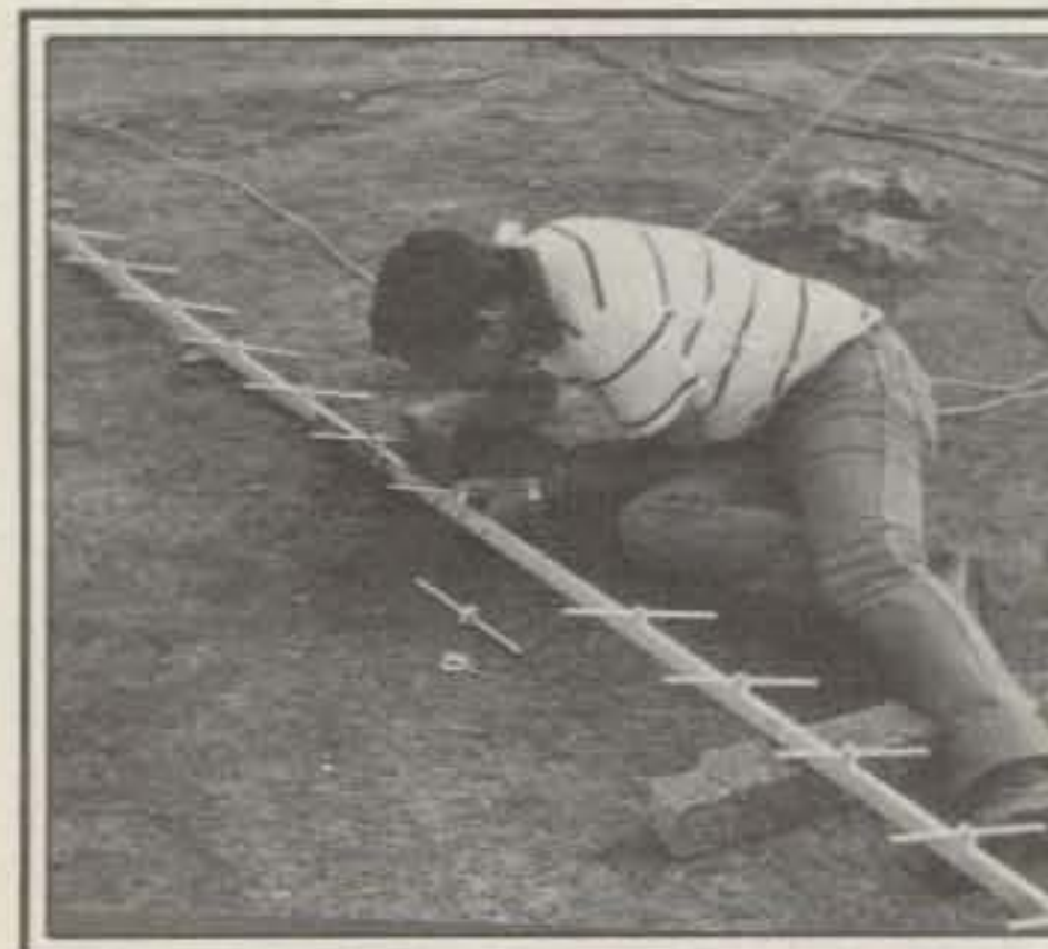
CT3BX and CT3DK operated from a portable site on Madeira Island, running two bands QRP. Hern and Manuel used 100% homebrew antennas. Here Hern, CT3BX, is shown repairing their 25-element 70 cm Yagi, a modification of the 21-element F9FT Tonna design.
