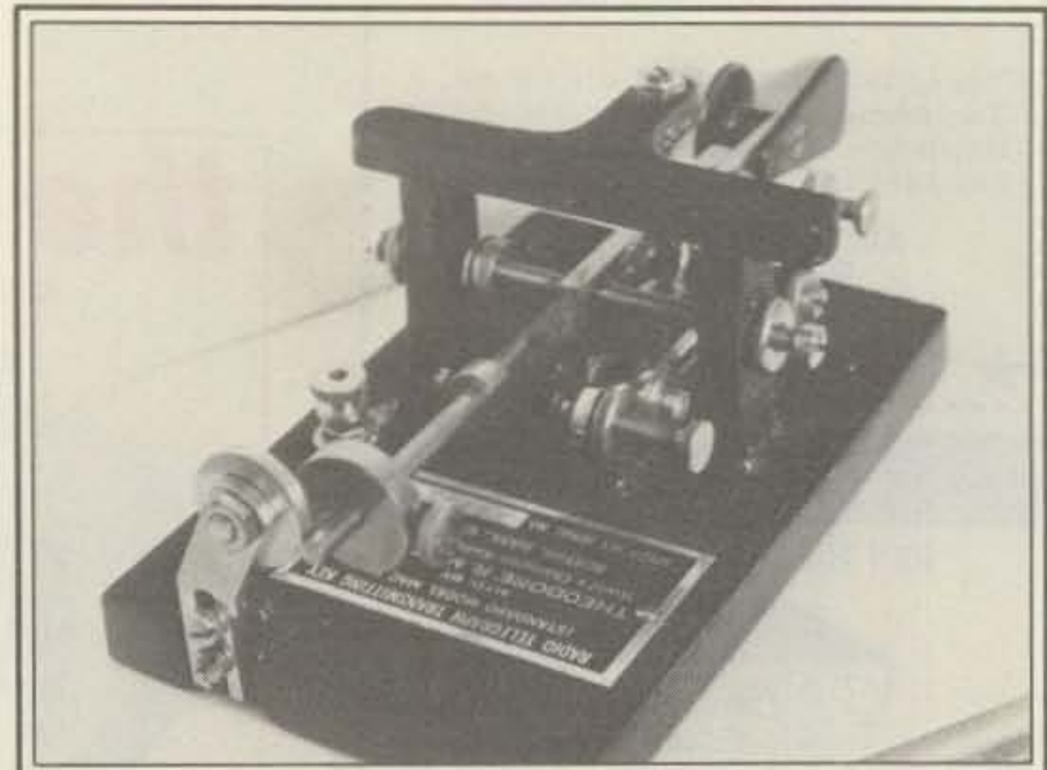
Fig. 3— VE7FOU's beautifully restored Mac Key. This classic gem was a pure "junkie" when Rick found it—no weight, damper, or fingerpieces.
