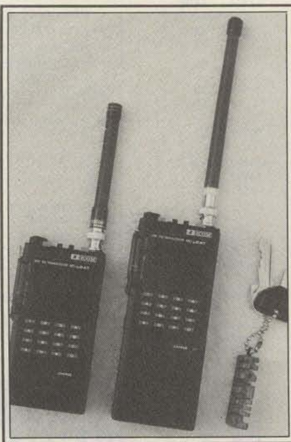
Fig. 1—The two ICOM IC-u2AT hand-held/pocket FM transceivers featured in this review. Left unit is "sized down" with supplied miniduck antenna and optional BP-21 battery pack. Right unit is using supplied BP-22 and optional full-size ducky.
