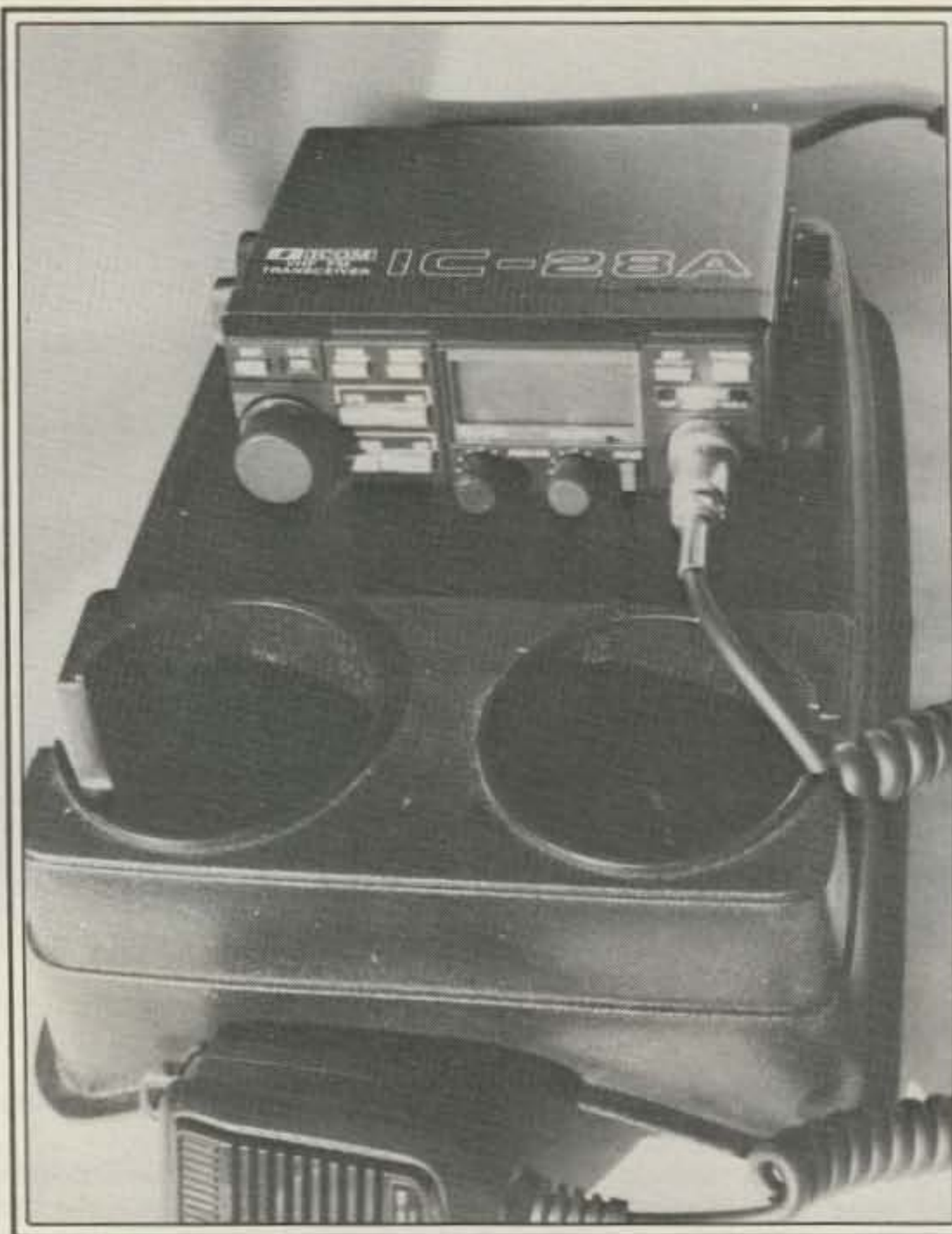
K6ARE's method of dealing with the "where to put the rig?" problem was to mount it to a plastic tray which straddles the transmission hump and can be moved quickly.
