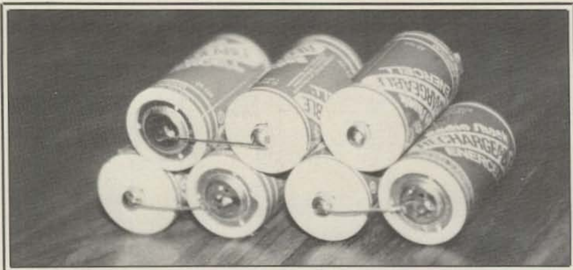
View of the assembled "C" cell pack ready for connection to the project case. Note that the solder connections are shiny, indicating that the solder flowed well at the battery end caps.
