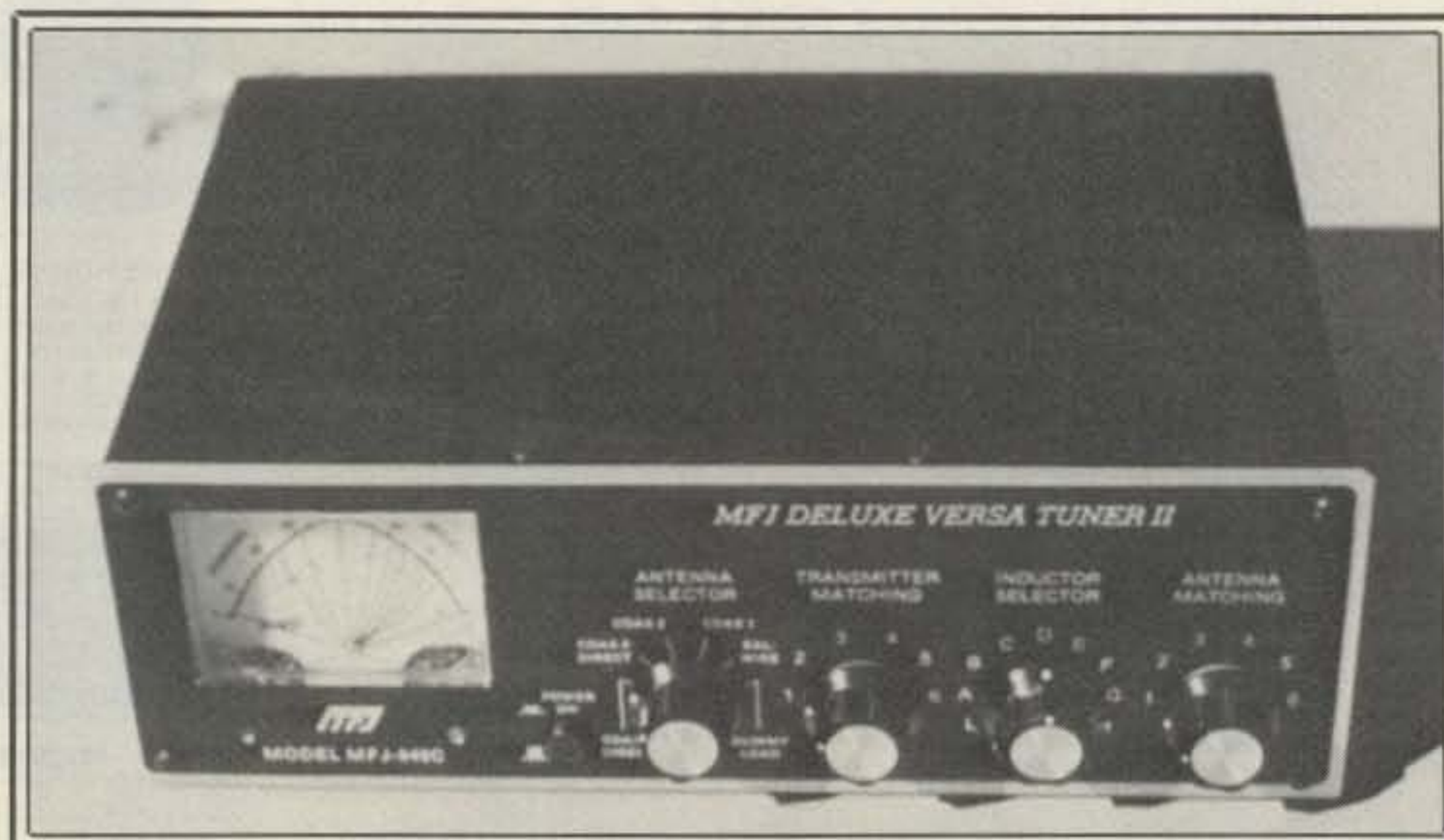
This photo shows the front-panel controls. The SWR/Power meter uses a dual needle type meter, at the left.
