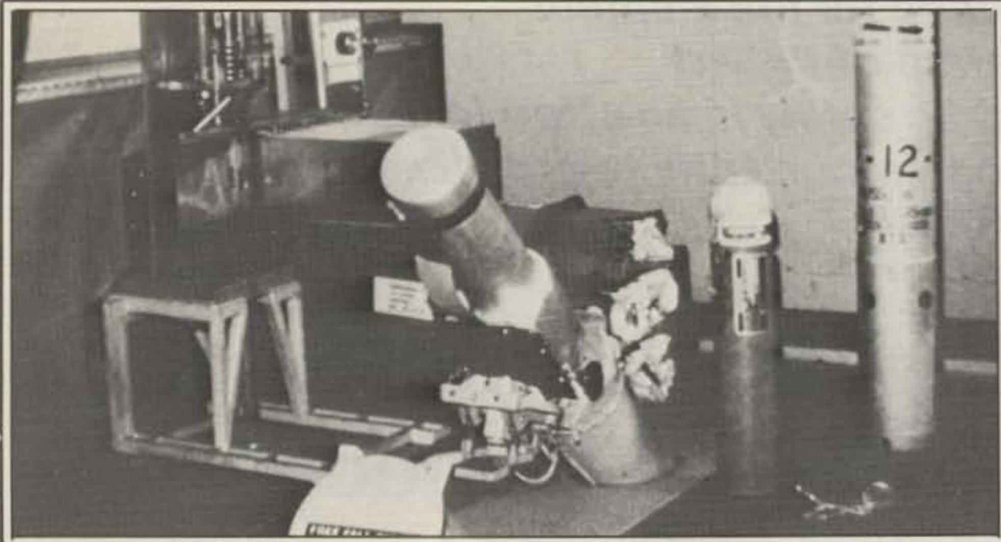
The dropsondes and the launching tube aboard the aircraft. (Photo courtesy of NOAA)
