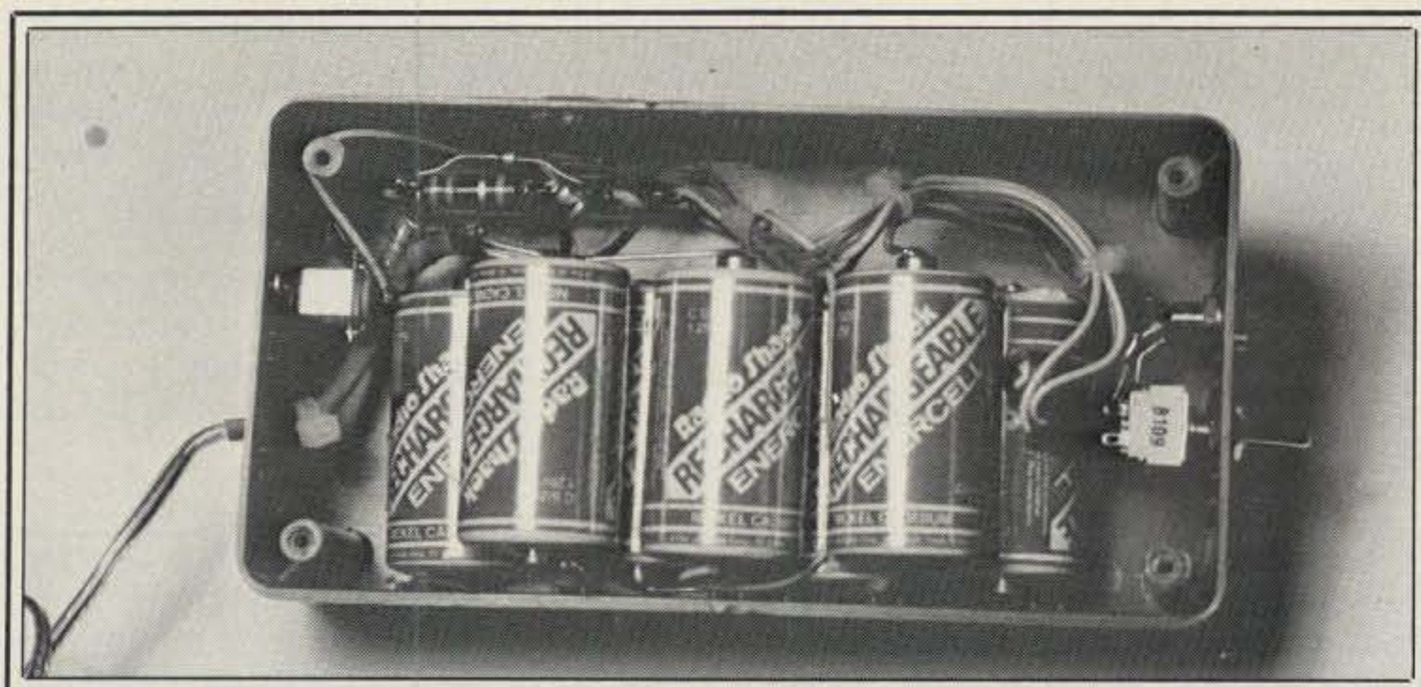
Top view of the completed project showing the relative placement of major components. The lead going from the left-hand side of the case is a 4 foot pair going to the handie-talkie.
