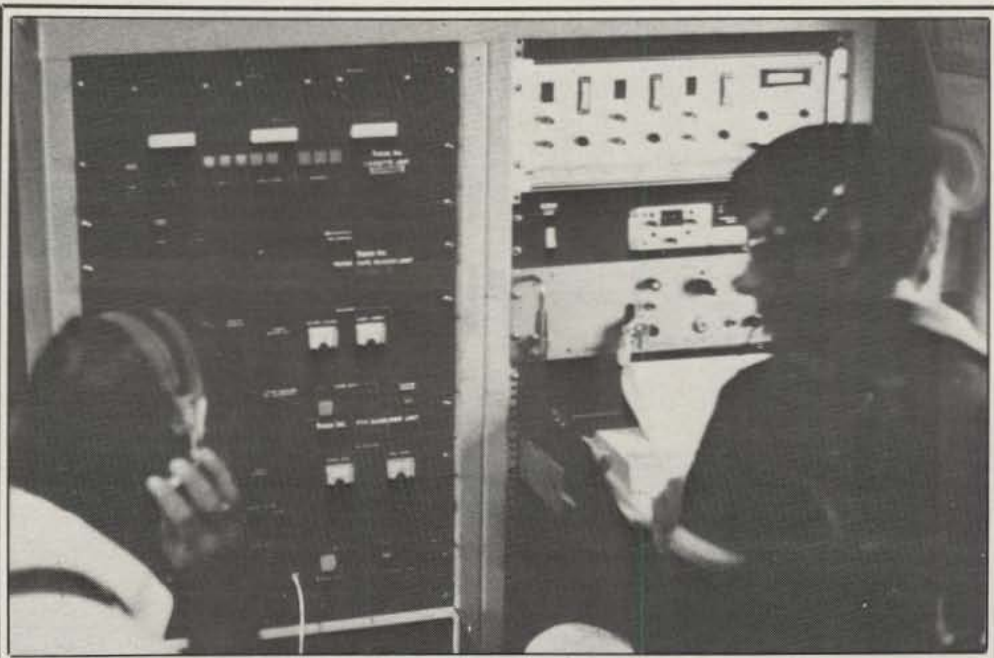
Here's a view of the dropsonde telemetry console with N4MEI, OAO Chief Systems Engineering Division, at the controls. (Photo courtesy of NOAA)
