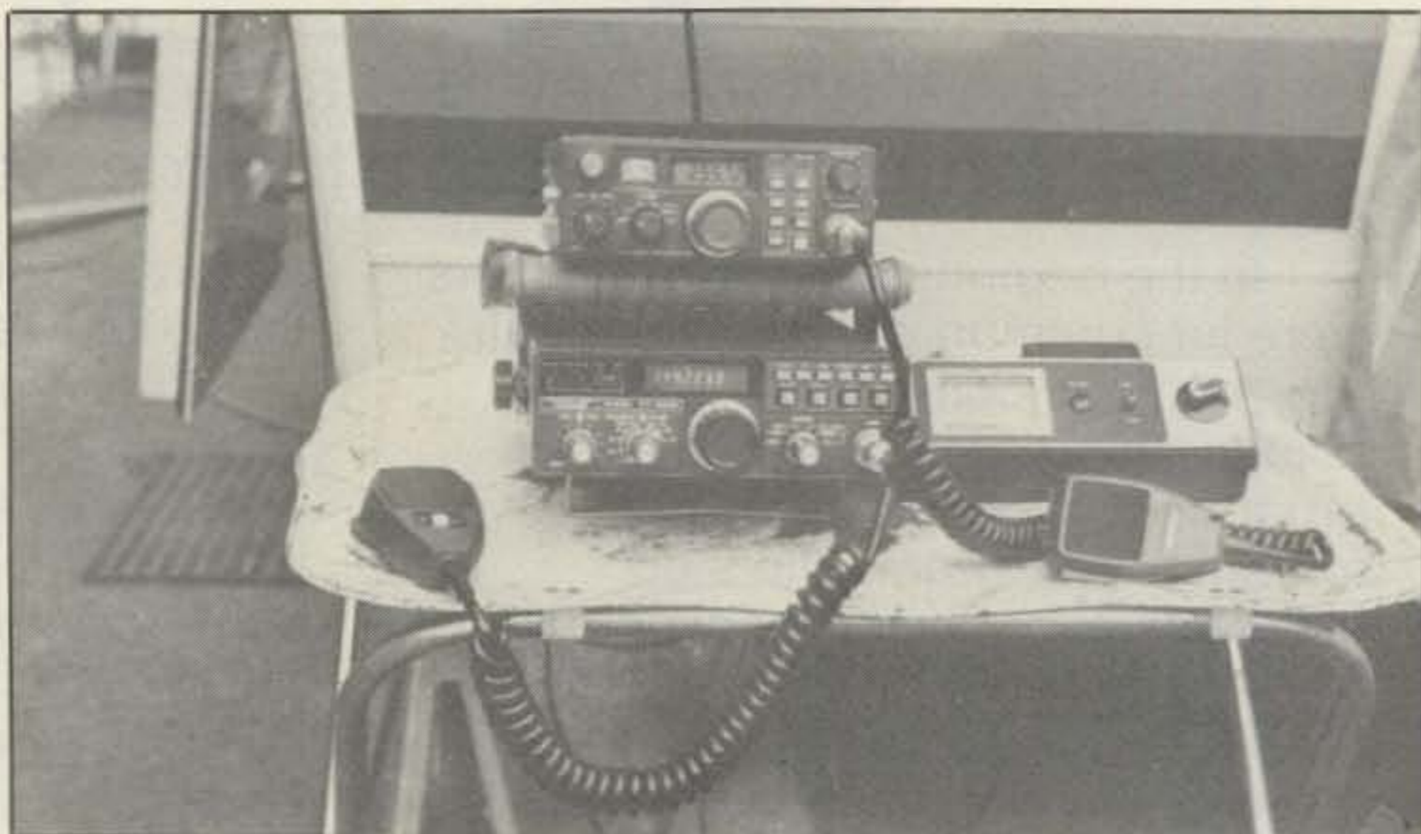
A prime example of mountain-topping or camping fun is exemplified in this TV tray setup situated in front of a camper. The top unit (FT-690R) and SWR bridge are used for 6 meters, while the bottom unit (FT-480R) is used for 2 meters. We'll let you guess which worked the most DX!
