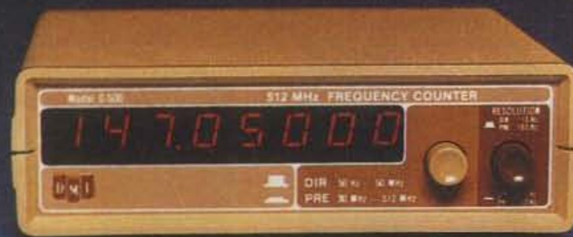
50 Hz to 512 MHz 5 1/4 X 5 X 1 1/2 1 PPM ACCURACY TCXO
