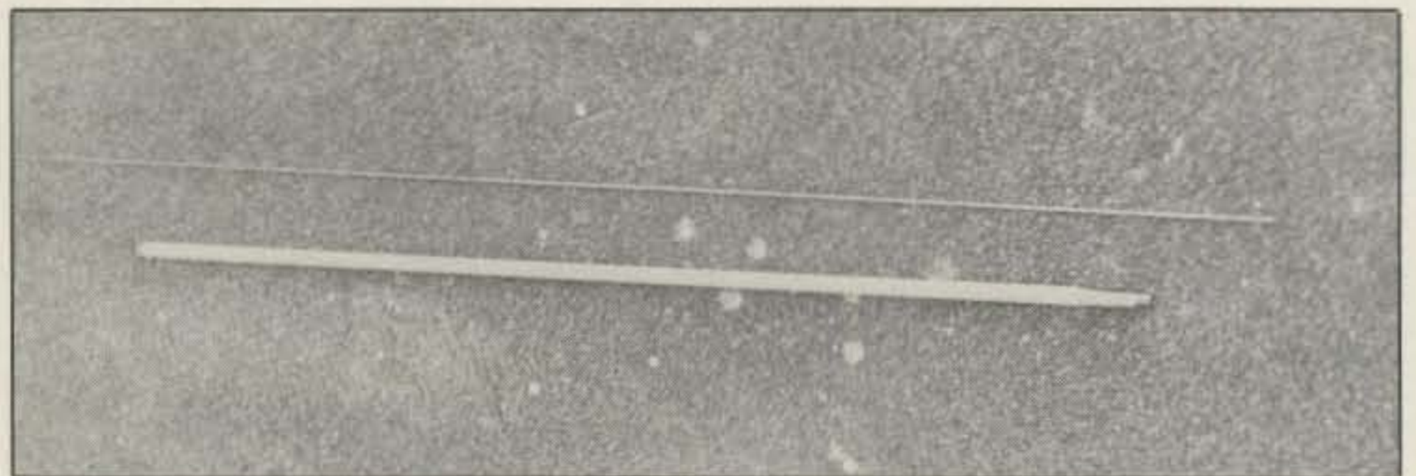
The bottom section of the antennas looks just like a fiberglass rod, while the top section appears to be a VHF-type whip.
