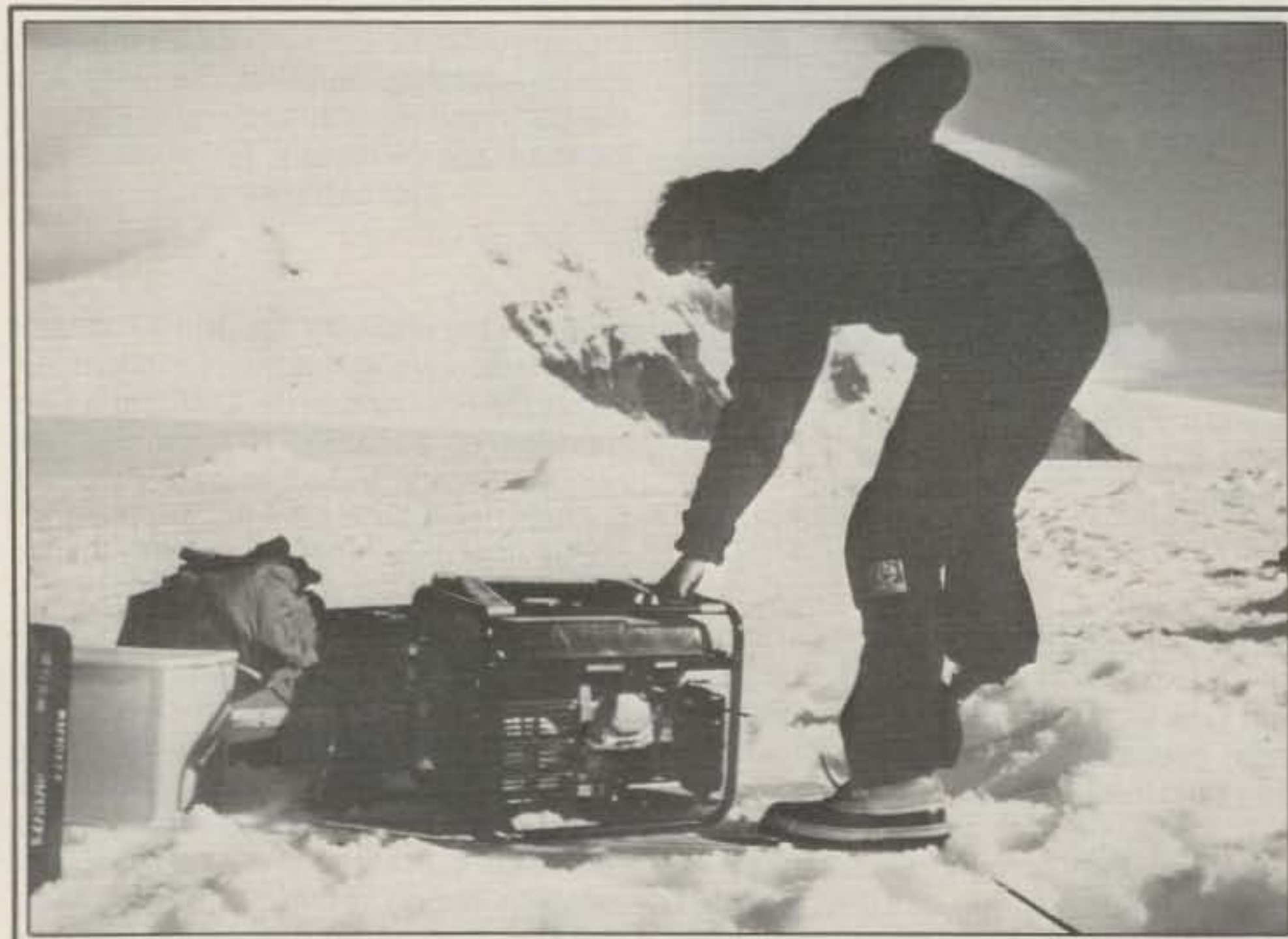
Einar starting the Honda EB2000X. It worked perfectly and only stopped when it ran out of fuel. We had expected icing problems, since temperatures were varying around the freezing point, but no such problems occurred.
