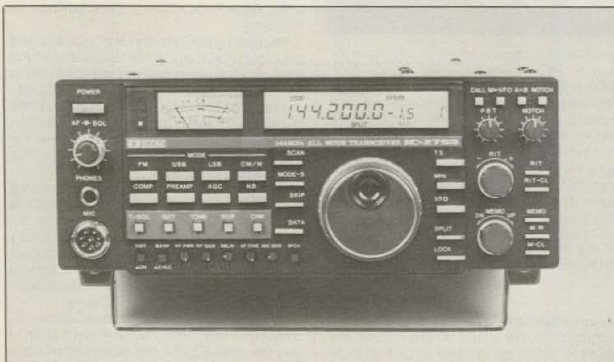
The ICOM IC-275A front panel contains 11 knobs, 35 pushbuttons, 2 LED status indicators, a multipurpose LCD display screen, mic and headphone connectors, and an analog S-meter! Despite all this, the rig is easy to use and becomes an extension of its operator's thoughts after a brief familiarization period.
