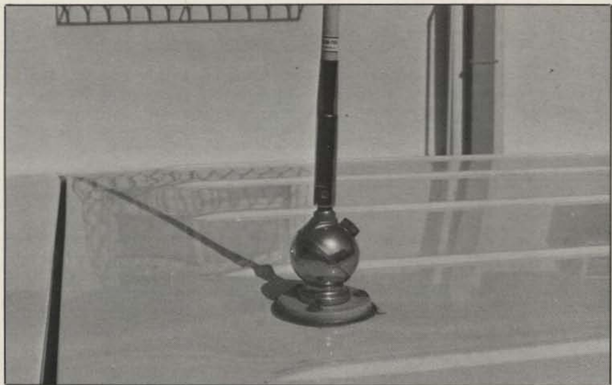
Quick disconnects may be used to rapidly change the "Ultimate" antennas. If you do use them, purchase quality units. Some of the inexpensive imported types can wobble quite a bit.
