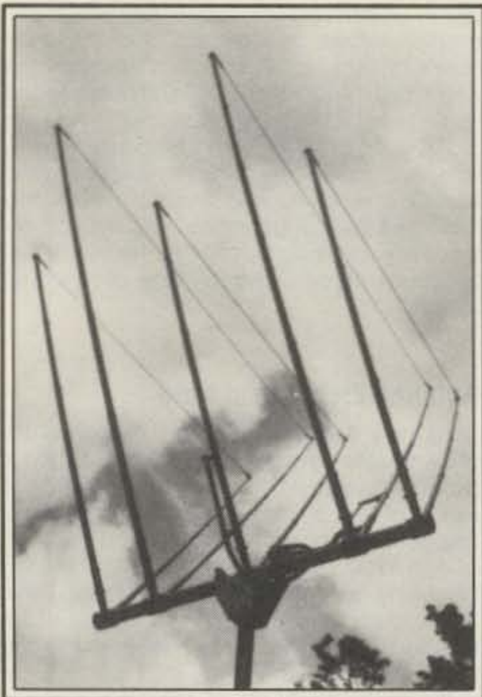
Looking good here is one of the "Big Horn" Delta Loops, this one a duobander covering 10 and 15 meters. Several other models are available with two or three elements for individual band coverage of 10, 12, 15, and 20 meters. (KA1UJ photo)
