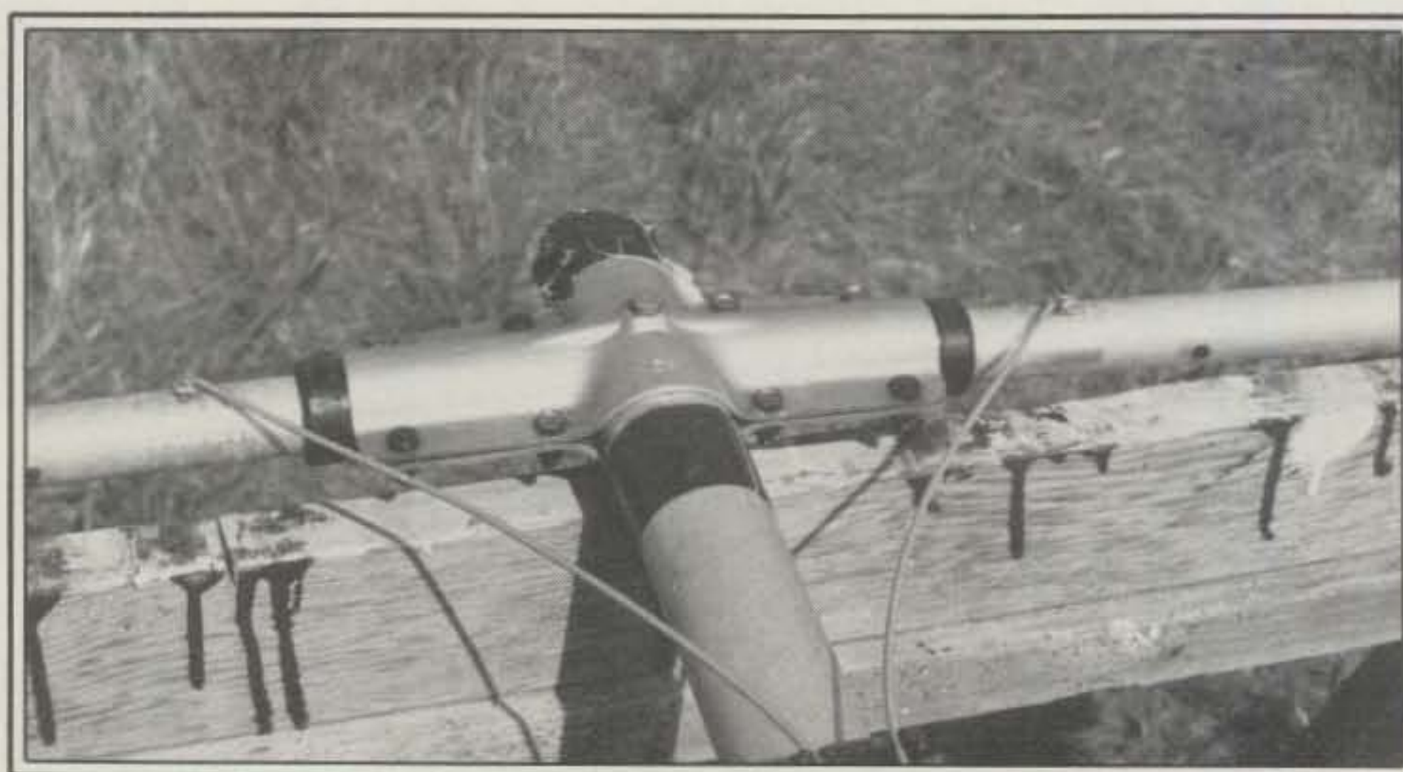
Fig. 2—Attachment of the loading stub to the reflector.
