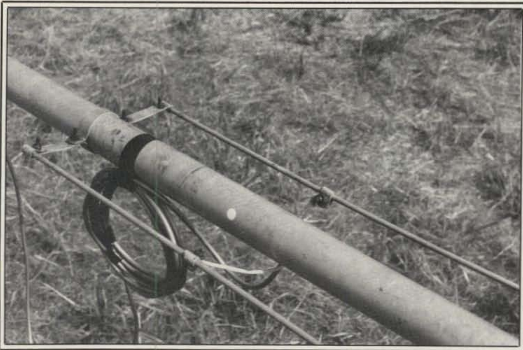
Fig. 4— Shorting bar and feedline attachment to beta match.
