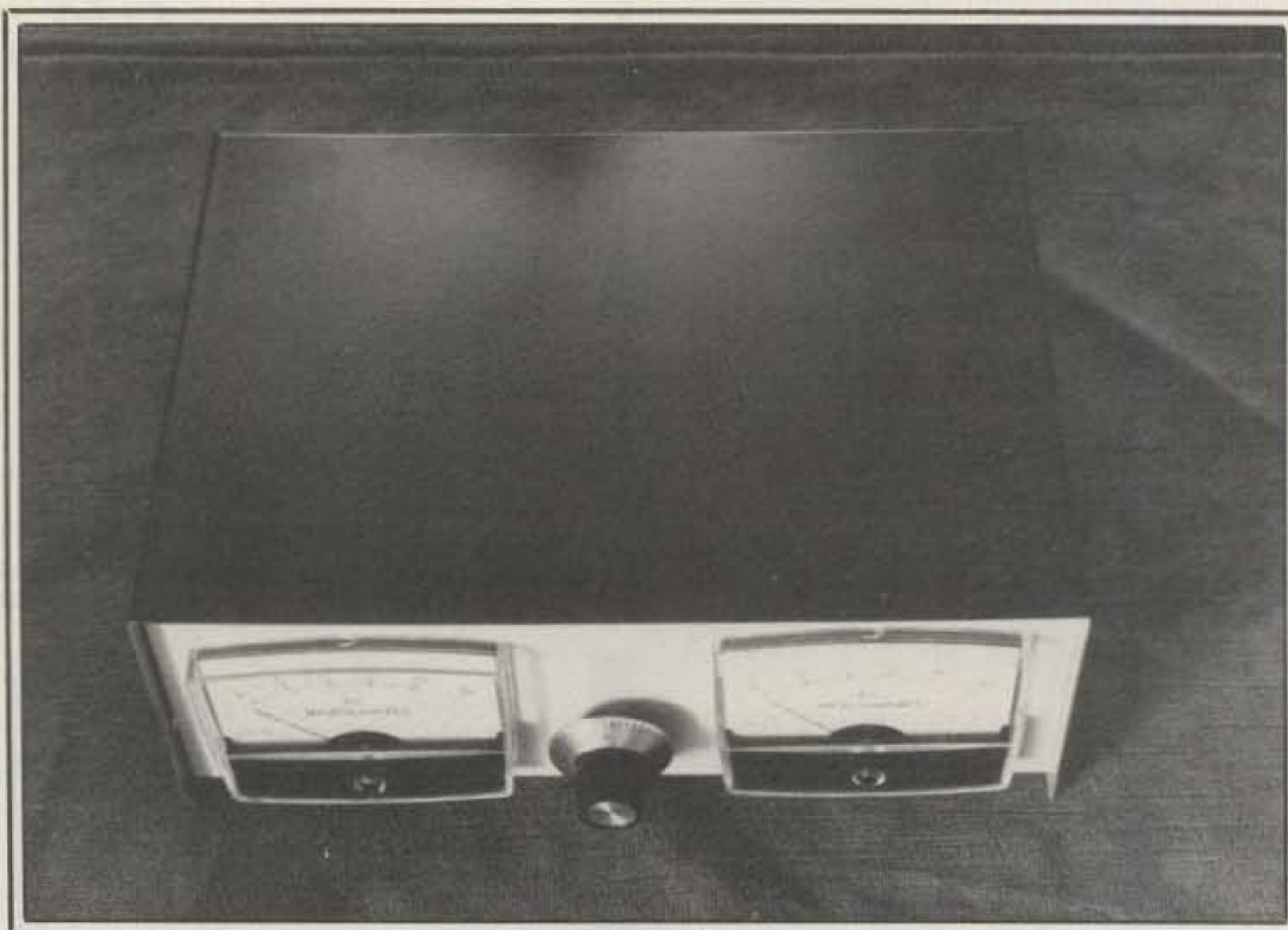
Looking down at the completed SWR bridge. It looks sleek and professional.
