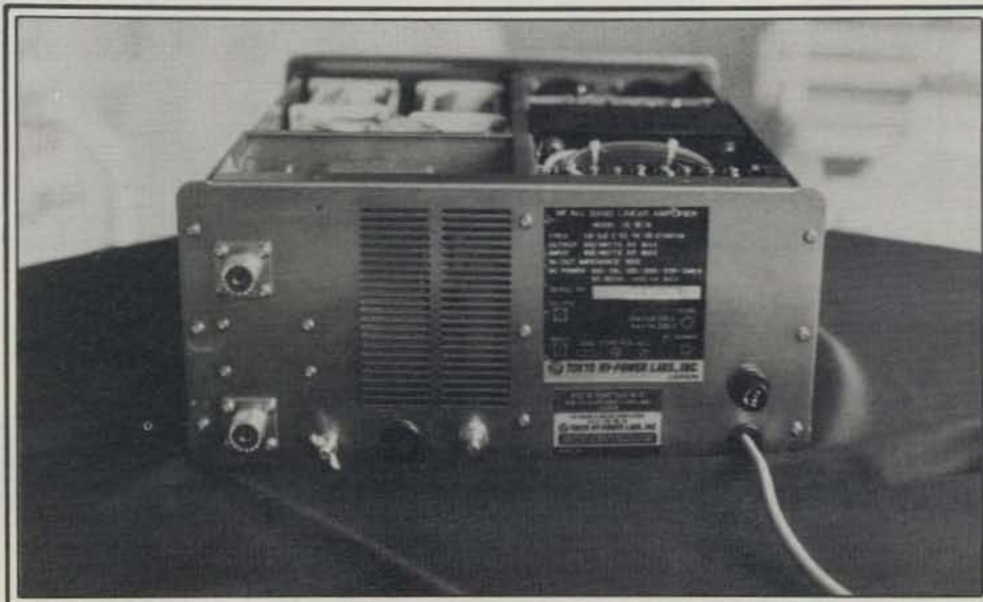
A view of the back panel (the top and bottom covers have been removed). Note the absence of any pop rivets or the like. Everything is secured with solid hardware.
