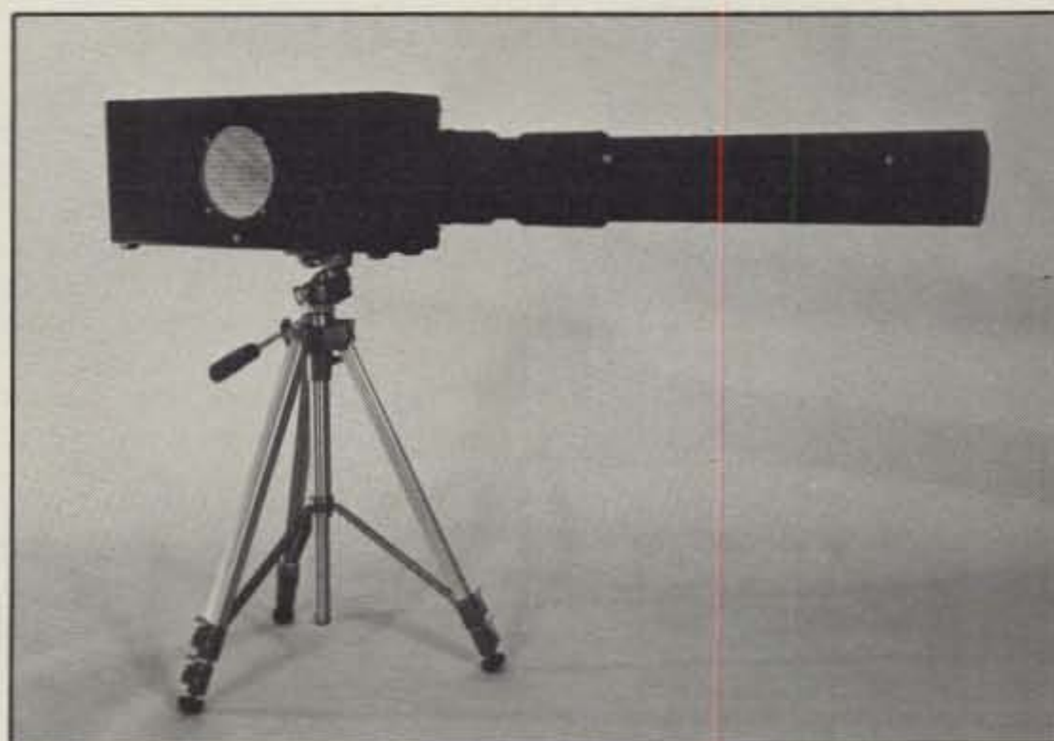
Shown here is a photomultiplier tube lightwave communications receiver. A 3 inch diameter lens is housed inside the long PVC pipe. (Photo copyright 1985 Steve J. Noll.)
