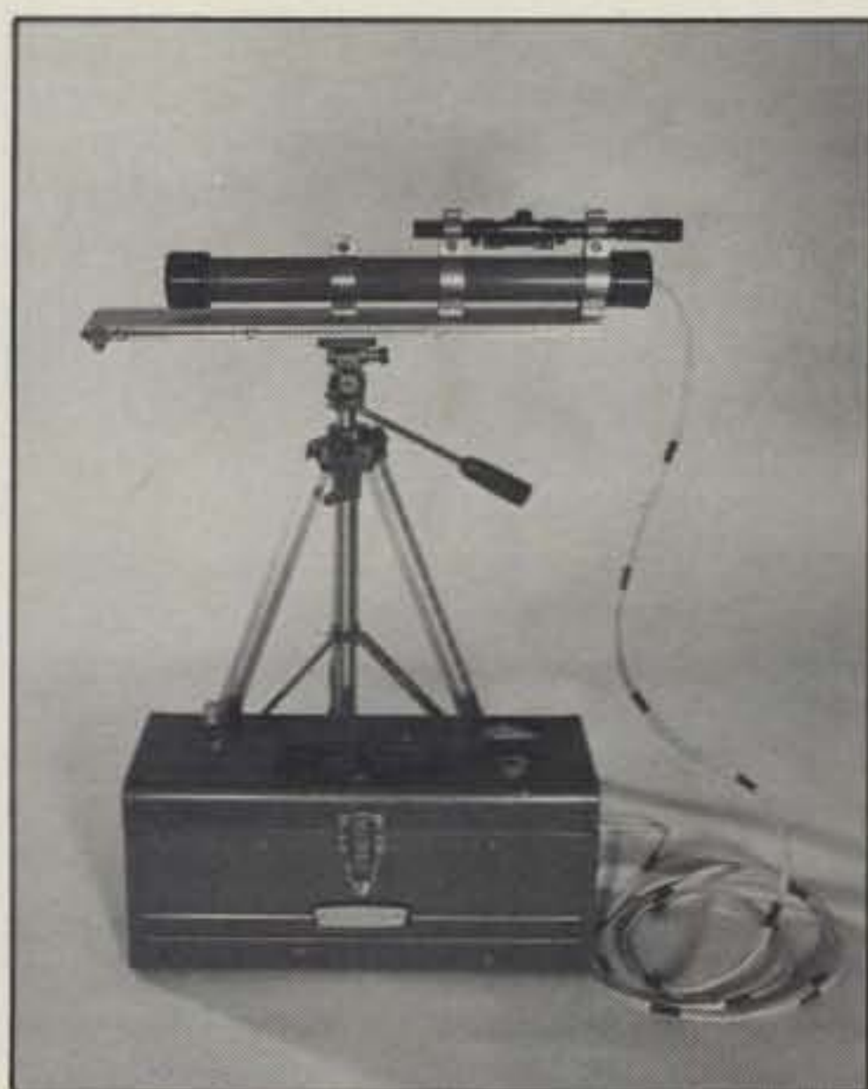
A practical helium neon laser setup. The power supply and battery are housed in the toolbox shown in the photo. (Photo copyright 1985 Steve J. Noll.)
