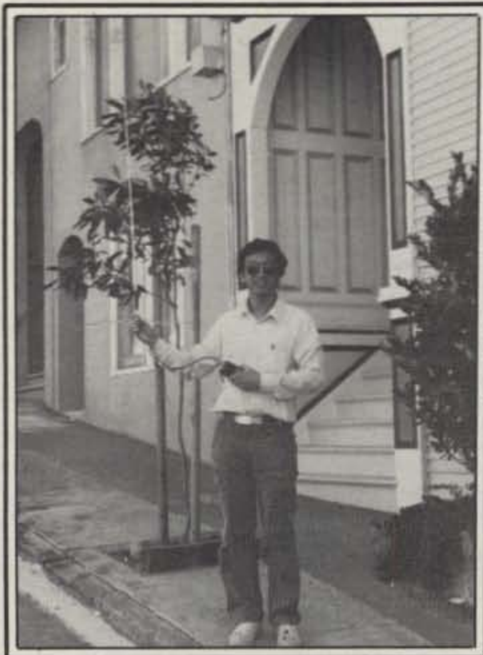
Fig. 3— Fully erected antenna which offers +9.5 dB of gain over a rubber duck.
