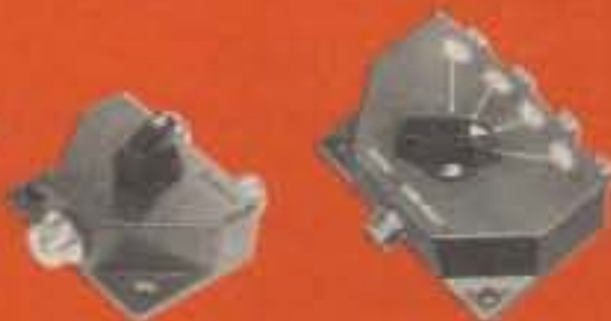
1.8-1500 MHz with SO-239, N-Type and BNC Connectors... VSWR below 1:1.2 ... Insertion loss less than 0.2dB... Unused terminals grounded for your protection... Rated up to 2.5 kW PEP... High dB terminal isolation.
