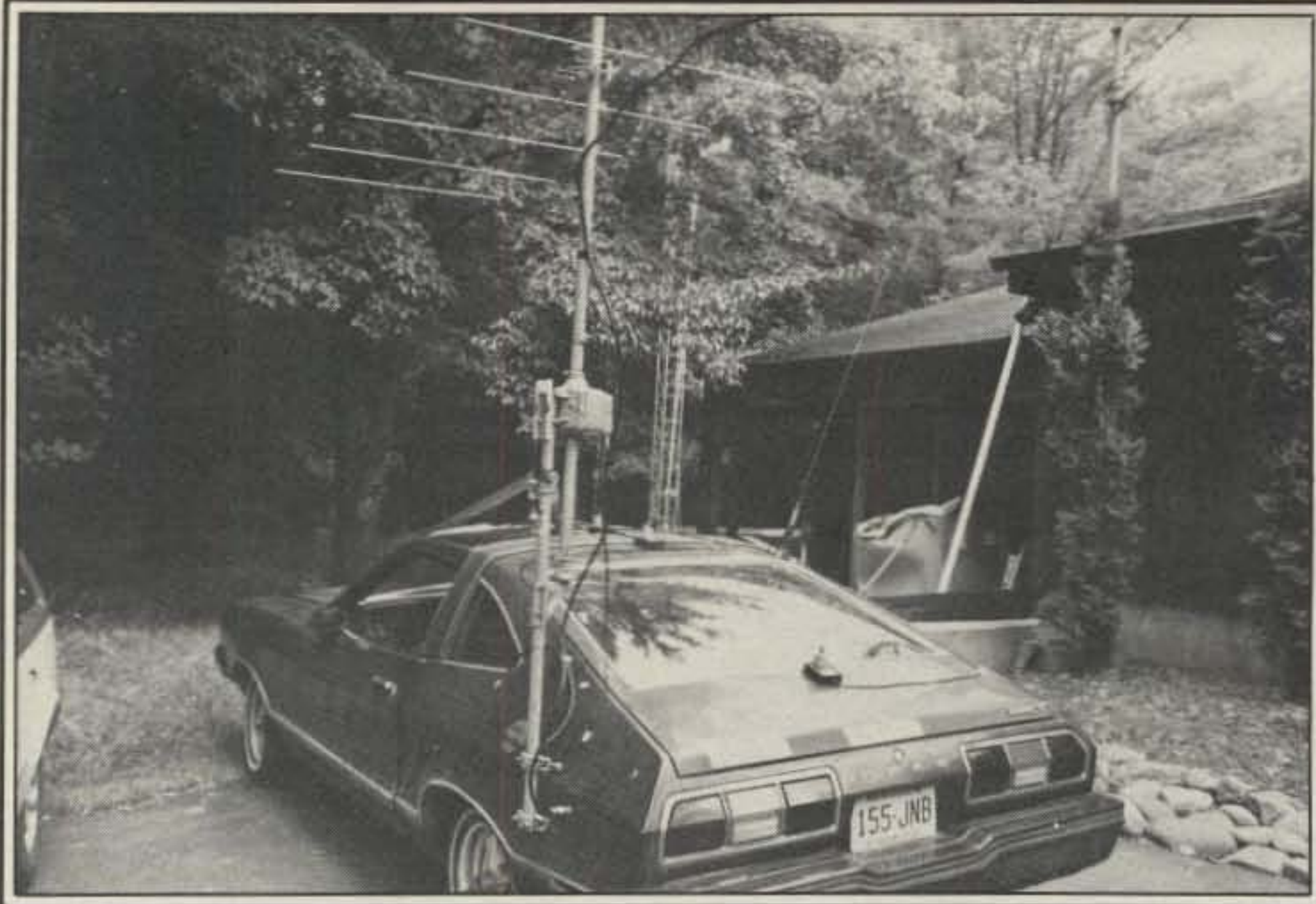
What most people see when K2SMN passes them in his Mustang is the 9-element F9FT "Tonna" beam for 144 MHz, complete with Alliance rotor. The car also sports several whips.
