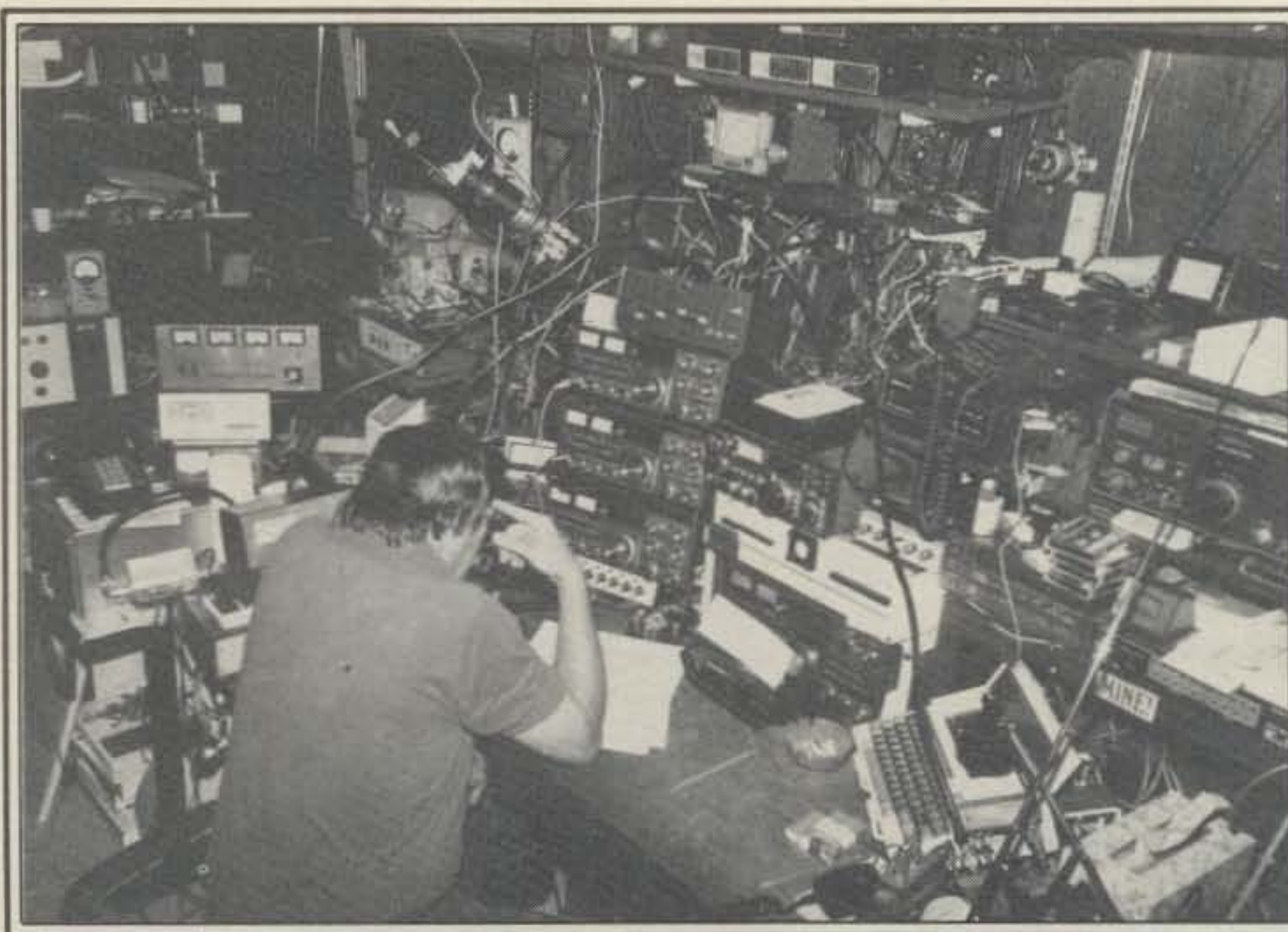
A closer look at K2SMN and some of the gear. Just to Roger's left is his microprocessor-based rotor controller for 144 and 1296 MHz; this allows antenna steering by presets. The audio mixer above that box controls which rig, or combination of rigs, is piped into his headphones. This allows listening on two bands simultaneously while wearing "cans."
