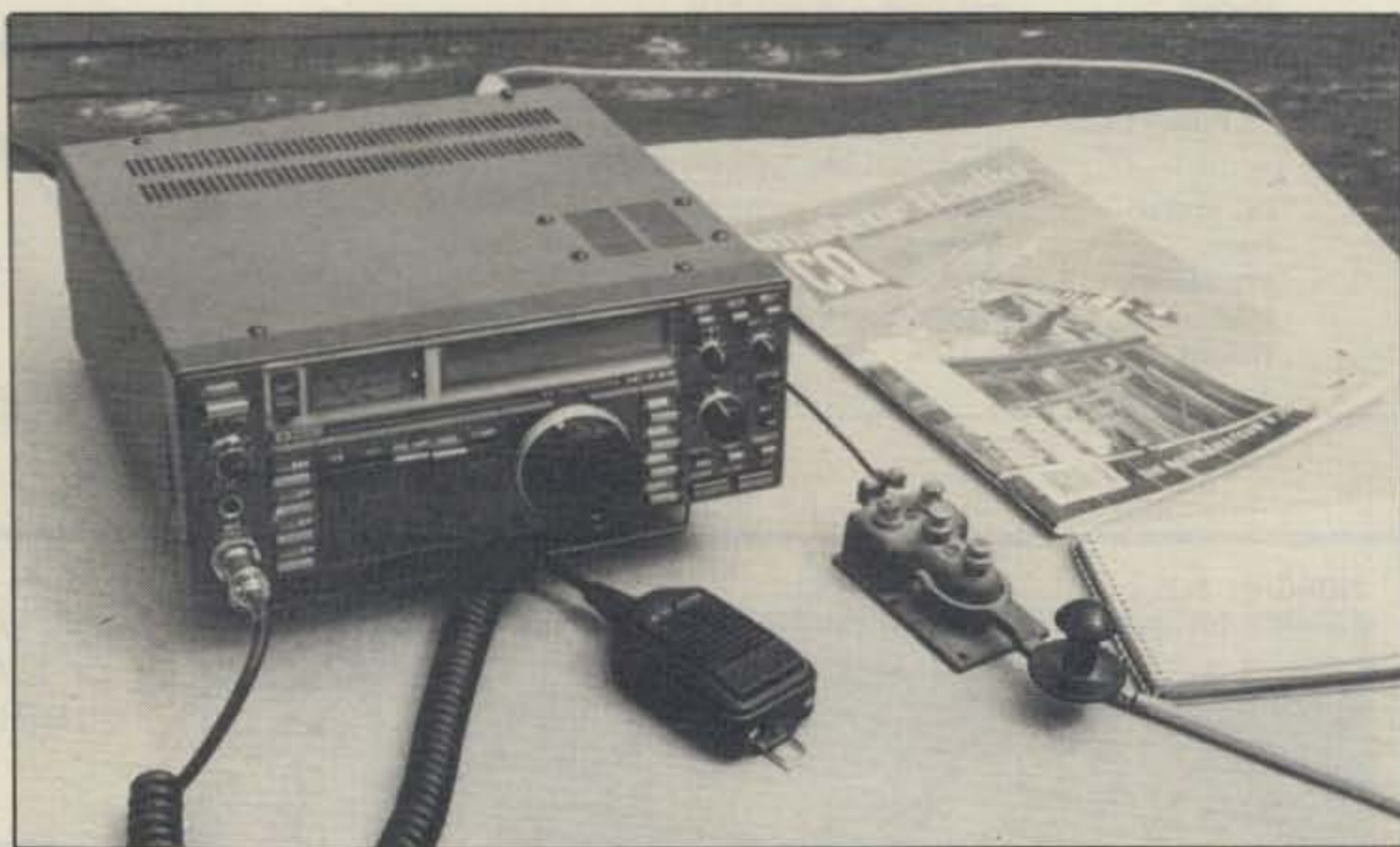
How simple can a station be? Here is the ICOM 735 set up with a mike and a key. The coax lead goes to a simple dipole as shown in Fig. 1.
