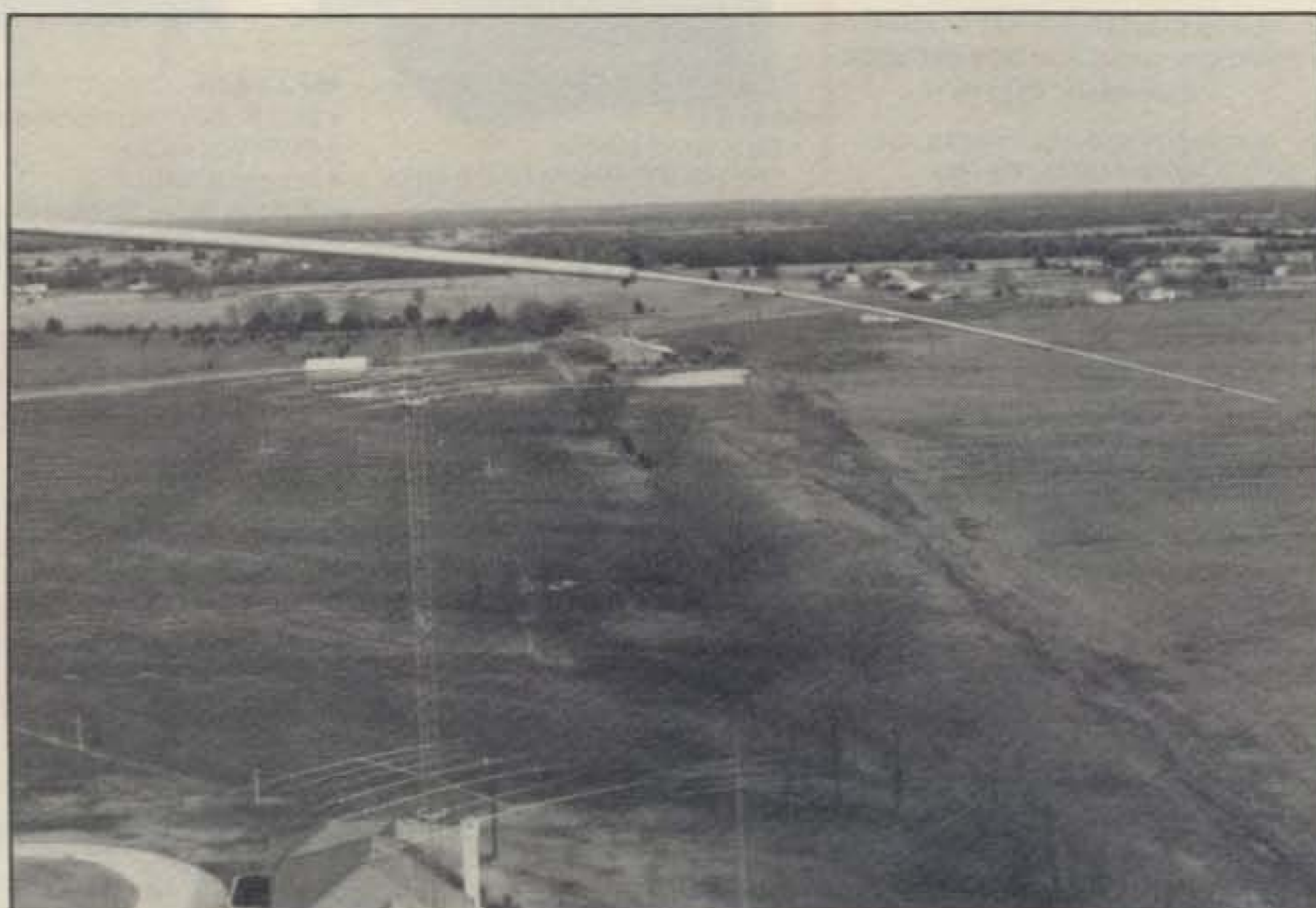
Fig. 1—View from the top of the 40-meter tower, looking east. Foreground-looking down at 145-foot rotating tower for TH28DX, 200 feet away. Right-A4 on 48-foot tower, 400 feet away. Element sag is quite noticeable from the top of the tower.
