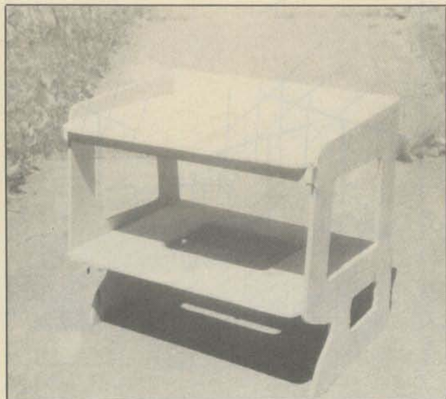
The completed rig rack. This view shows the locations of holes placed in the sides and bottom shelves.
