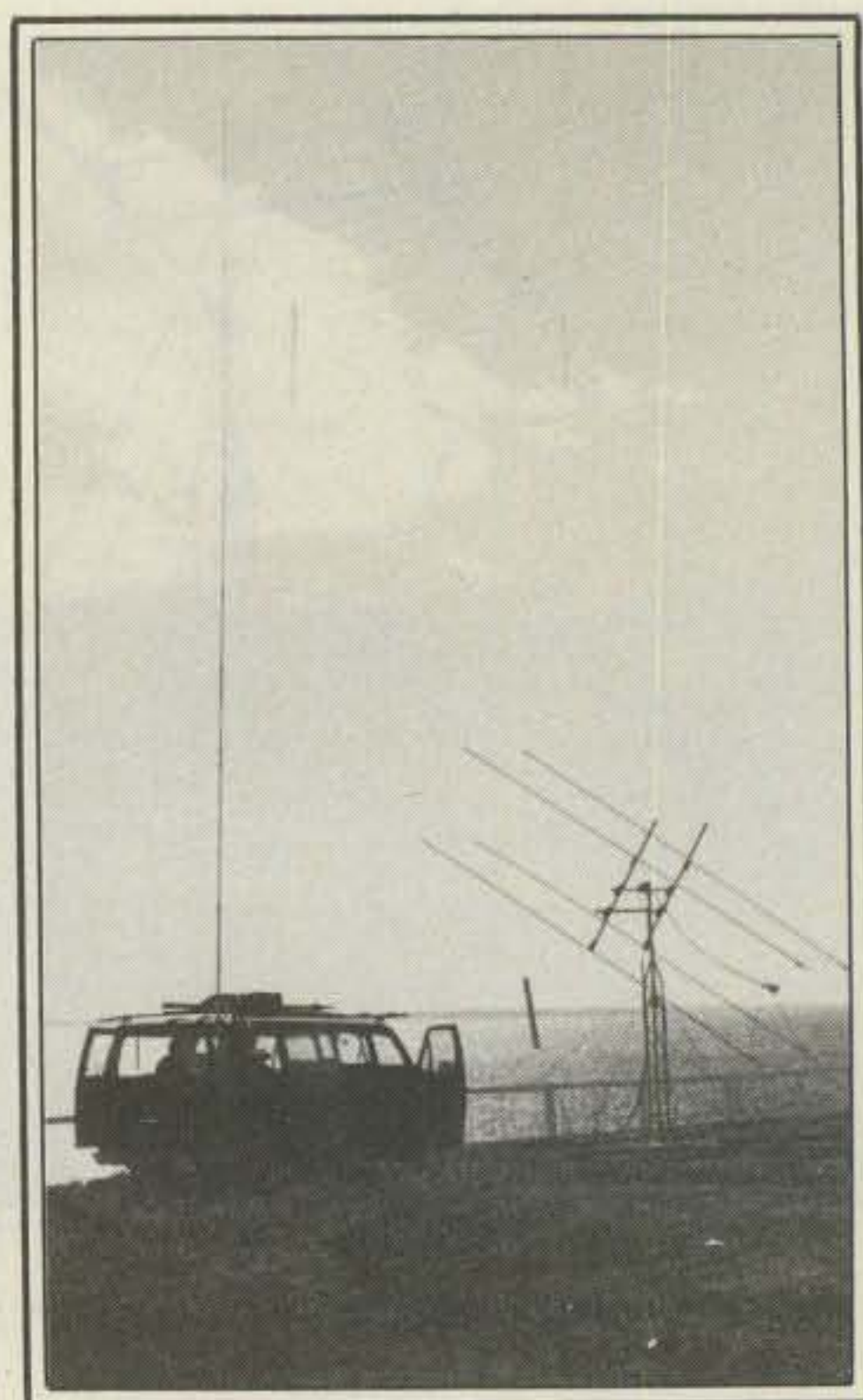
The crew waits for moonrise on the Straight of Belle Isle. The 35 ft. whip on the van was used for 20M liaison with 432 MHz EME net.
