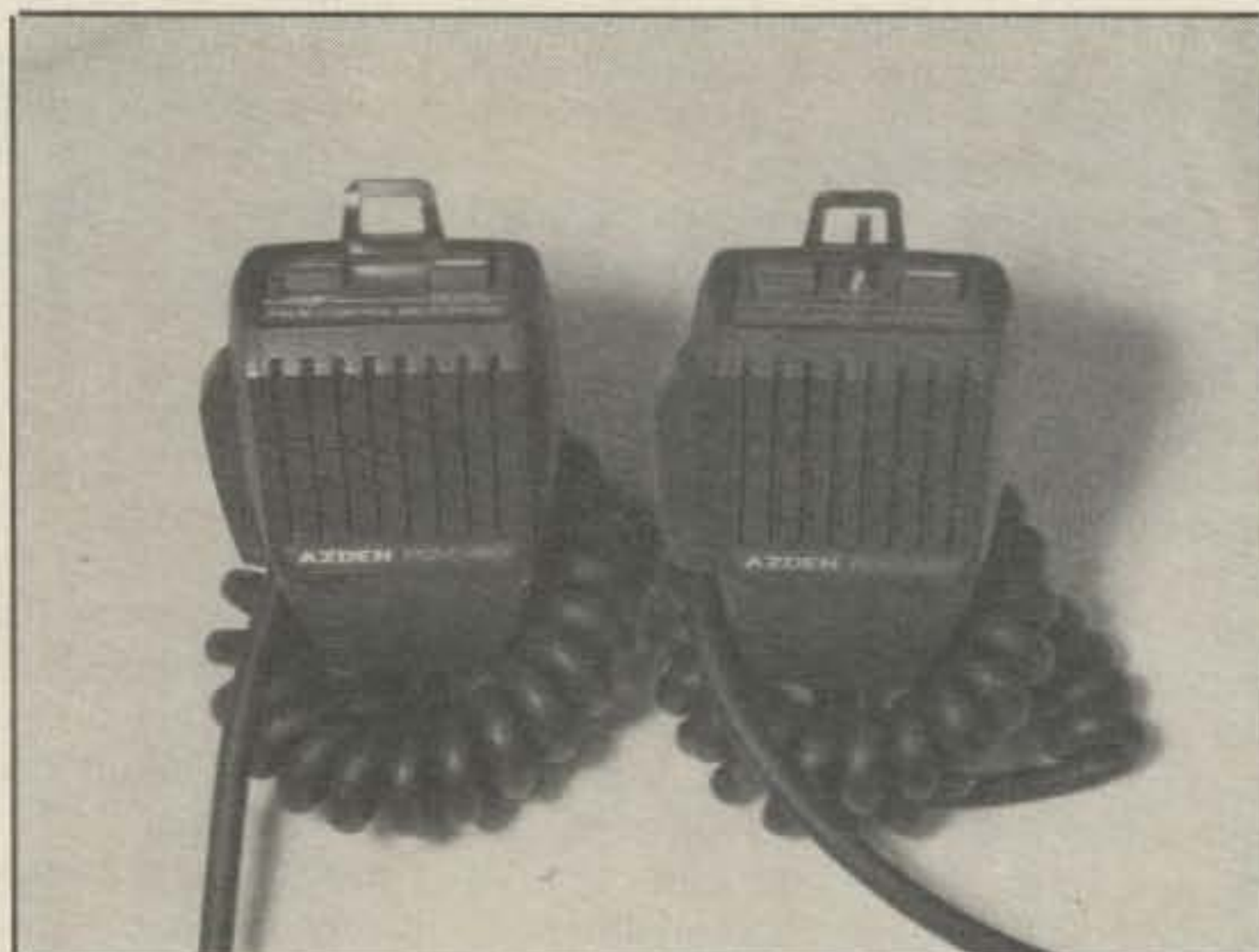
A view of the unmodified and modified microphones. The micro switch is conveniently located and accessible, yet does not interfere with mic usage.
