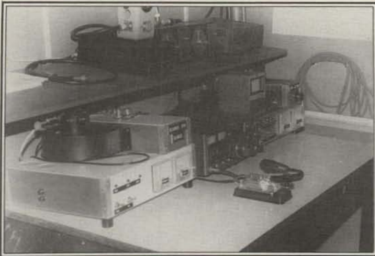
GJ4ICD's neat layout includes 3CX800A7 kilowatt amplifiers for 144 and 432 MHz, FT-726R and assorted accessories. Geoff says the amplifiers have built-in power supplies using toroidal transformers. Are these switched-mode units, Geoff?
