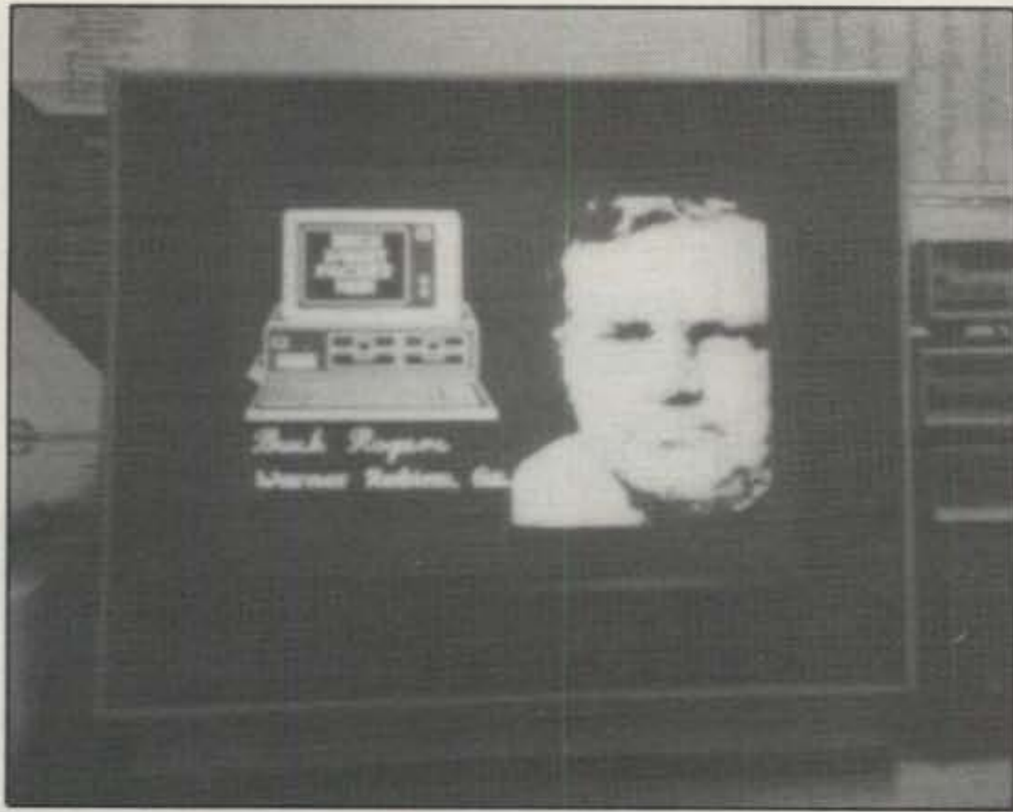
A completed packet picture sent from WD4MNT to K4ABT. Since it can be saved on disk, it can be run again at any time.
