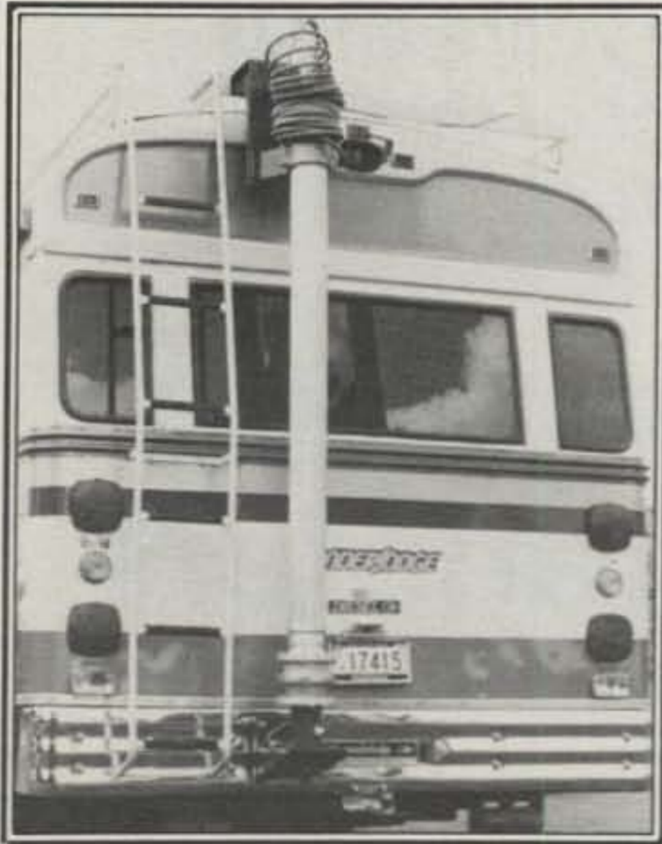
The nested pneumatic mast on the rear of the RV. The coil of cable at the top is the antenna coax. It will spiral up the mast as it is raised.
