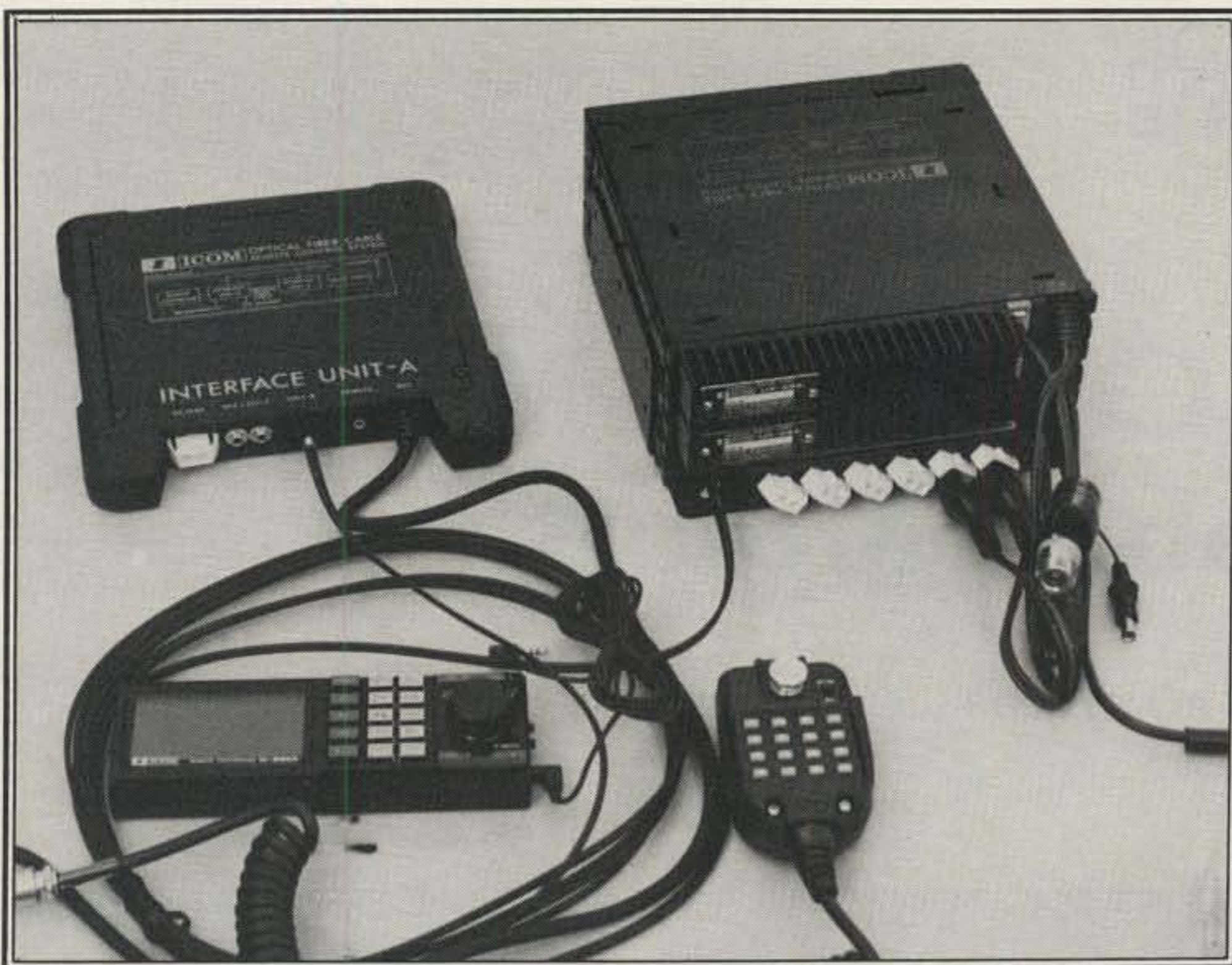
This is the 900 with everything shown except the speaker. The mounting bracket with the two RF modules is at the upper left and Interface A is at the left.
