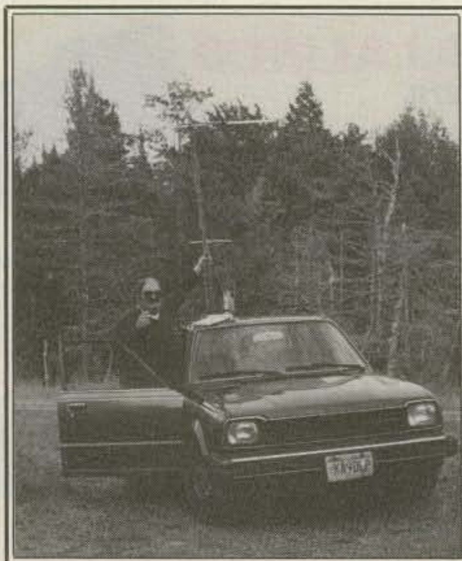
WB9MSV/8, EN56. See the little 3-element 2 meter beam mounted to the end of an oar? With this setup and a 25 watt multimode, Larry made over 120 contacts spanning half the country last July.
