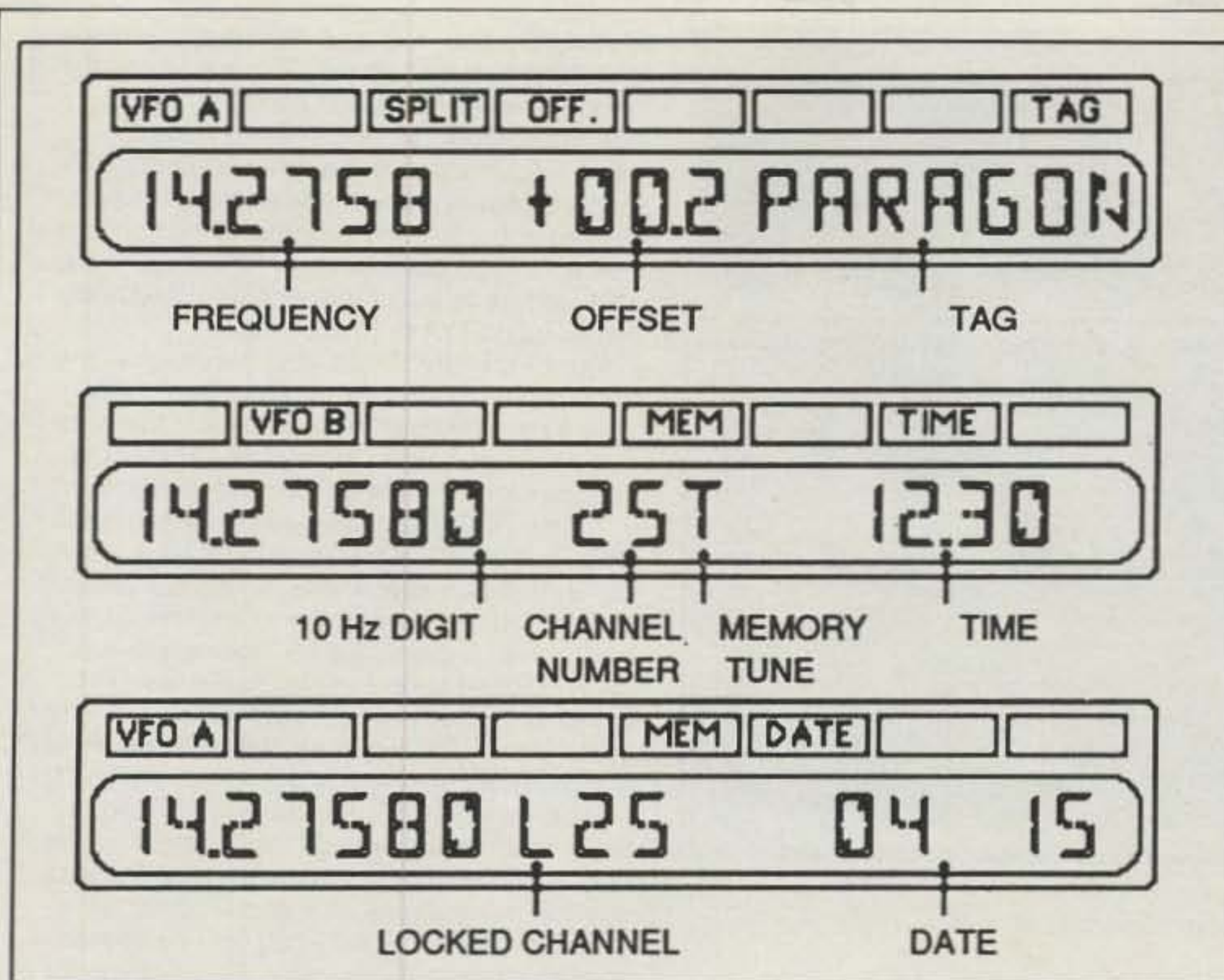
Fig. 1—This diagram illustrates just about all of the displays possible. You have to imagine that the large display is a soft fluorescent green color while the annunciators above are a backlighted yellow. The one display that is not shown is the one that will tell you which software version on an EPROM is installed in a Paragon.
