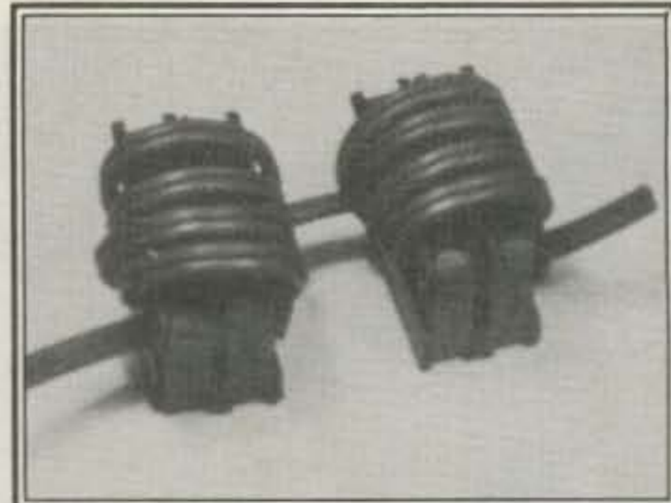
Here we see the AC line wound over four snap-on chokes, in groups of two. This would provide about 30 dB of attenuation from the broadcast band to 300 MHz or so.
