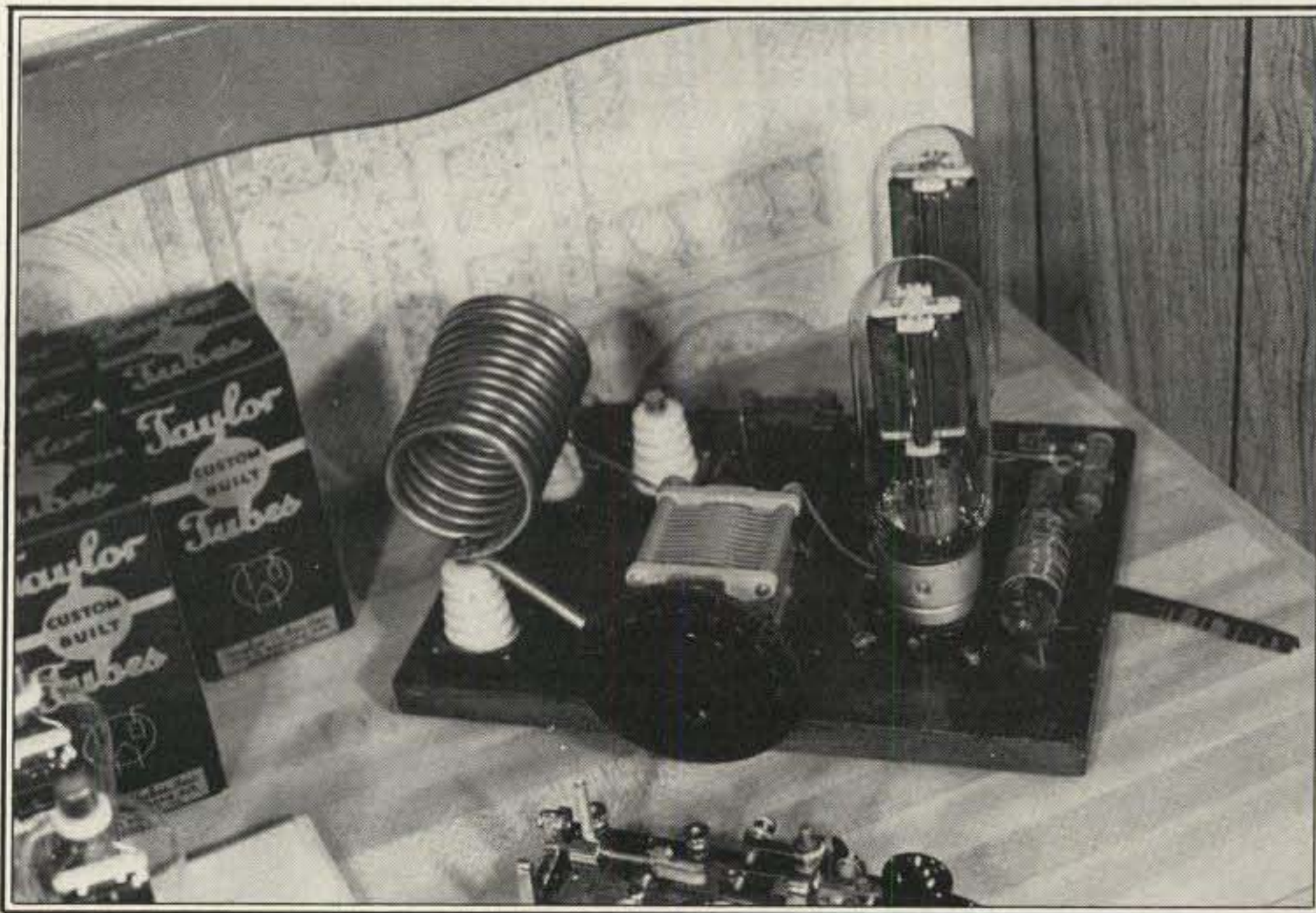
Layout of K4TWJ's big bottled push-pull TNT before addition of antenna coils. The tube's glow is fantastic!
