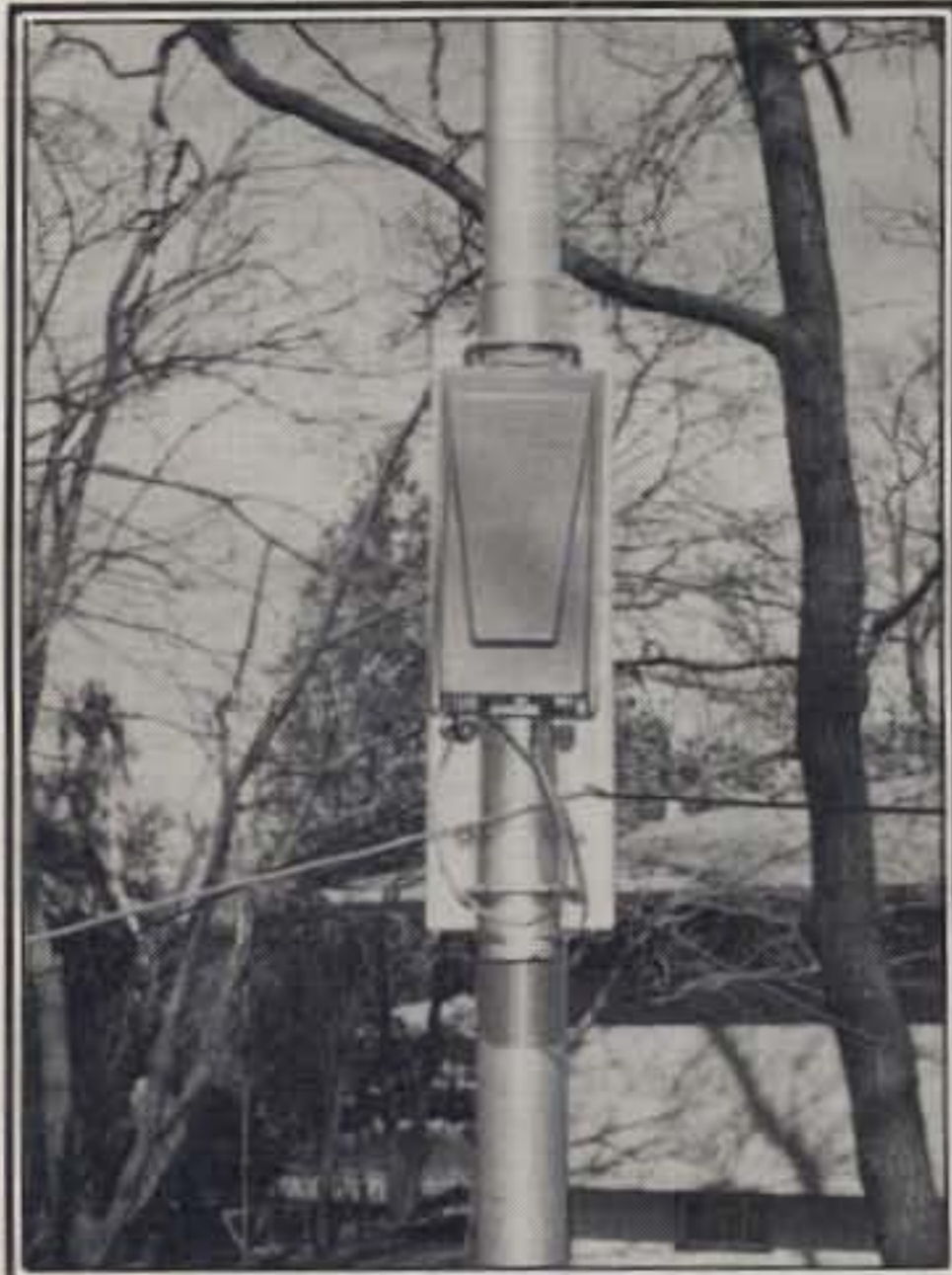
With the weather resistant-cover down, the AD385 protects the relay and CW matching coil from the worst that mother nature has to offer.
