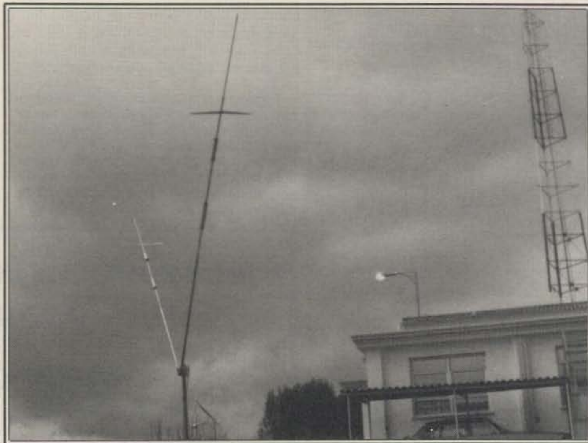
The 730V-1's appearance is accented by the two little "bat-wing" capacitance hats. The 730V-1 won't perform as well as a beam on a tower (that's a 200 foot self-supporting tower on the right), but it is a very good performer for its size.
