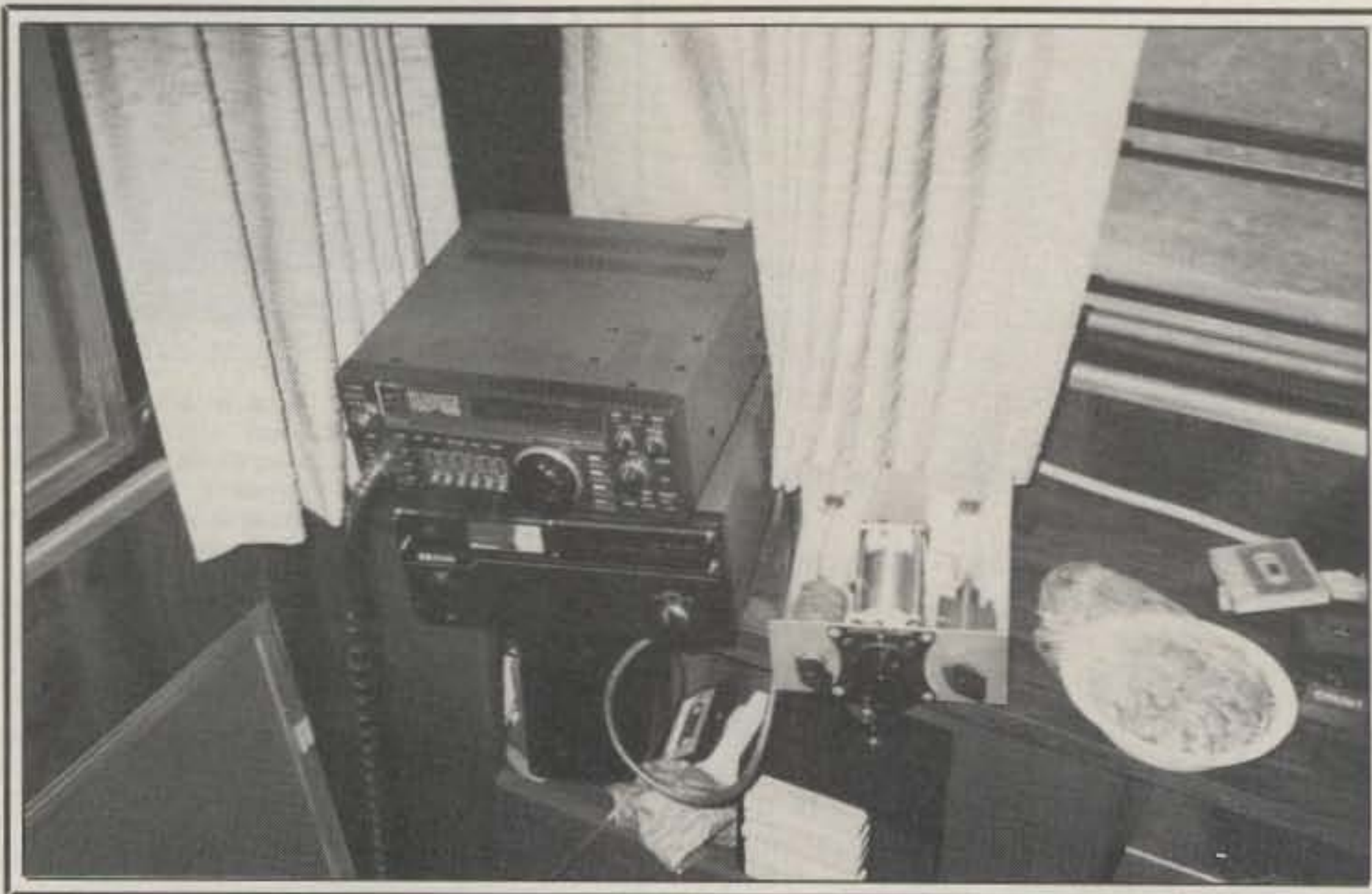
The operating position with the ICOM 735. At the right is a small Transmatch I use, and it easily handles the tuned coax feeder.
