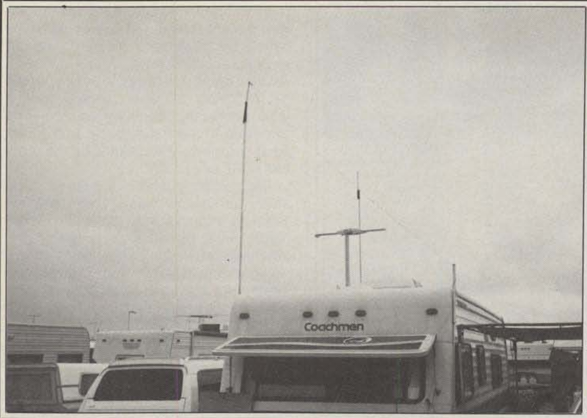
Here is the RV Wonder installed at its full height. The antenna wire terminates just below the front awning of the trailer, at which point the coax is attached. Keep in mind that the coax is used as a tuned feeder.
