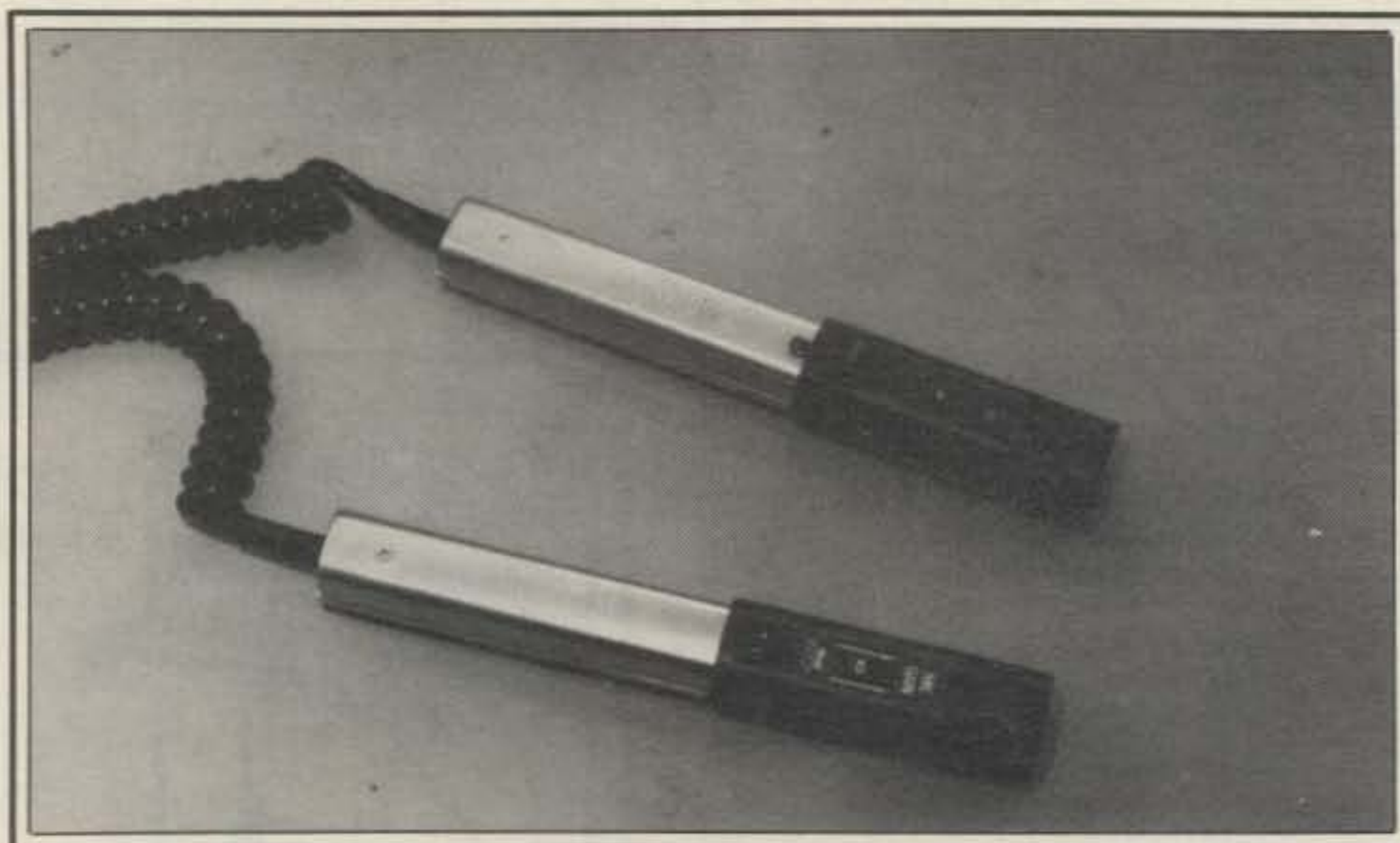
The converted microphone (upper one) looks almost exactly like the original Hy-Gain 617 unit except for a different PTT switch.
