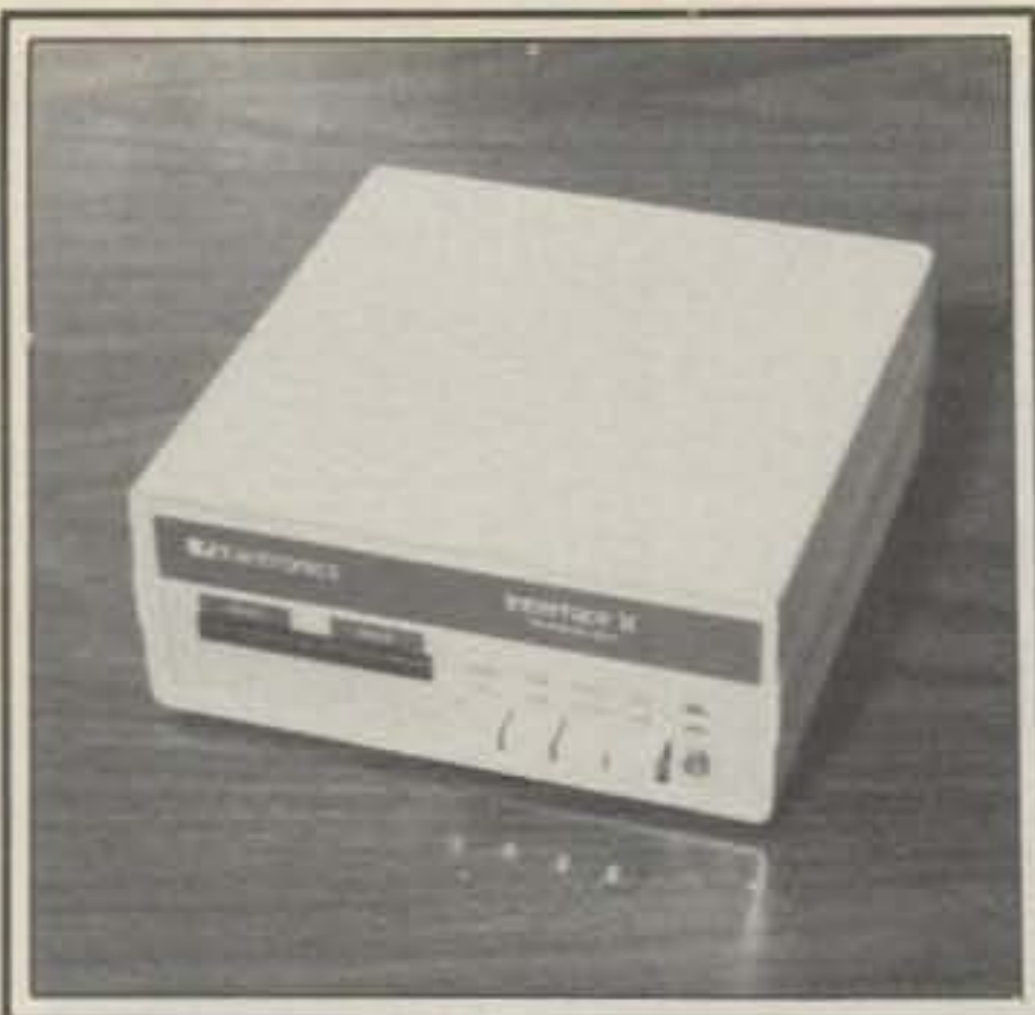
The Kantronics Interface II is representative of the older single-mode RTTY units.
