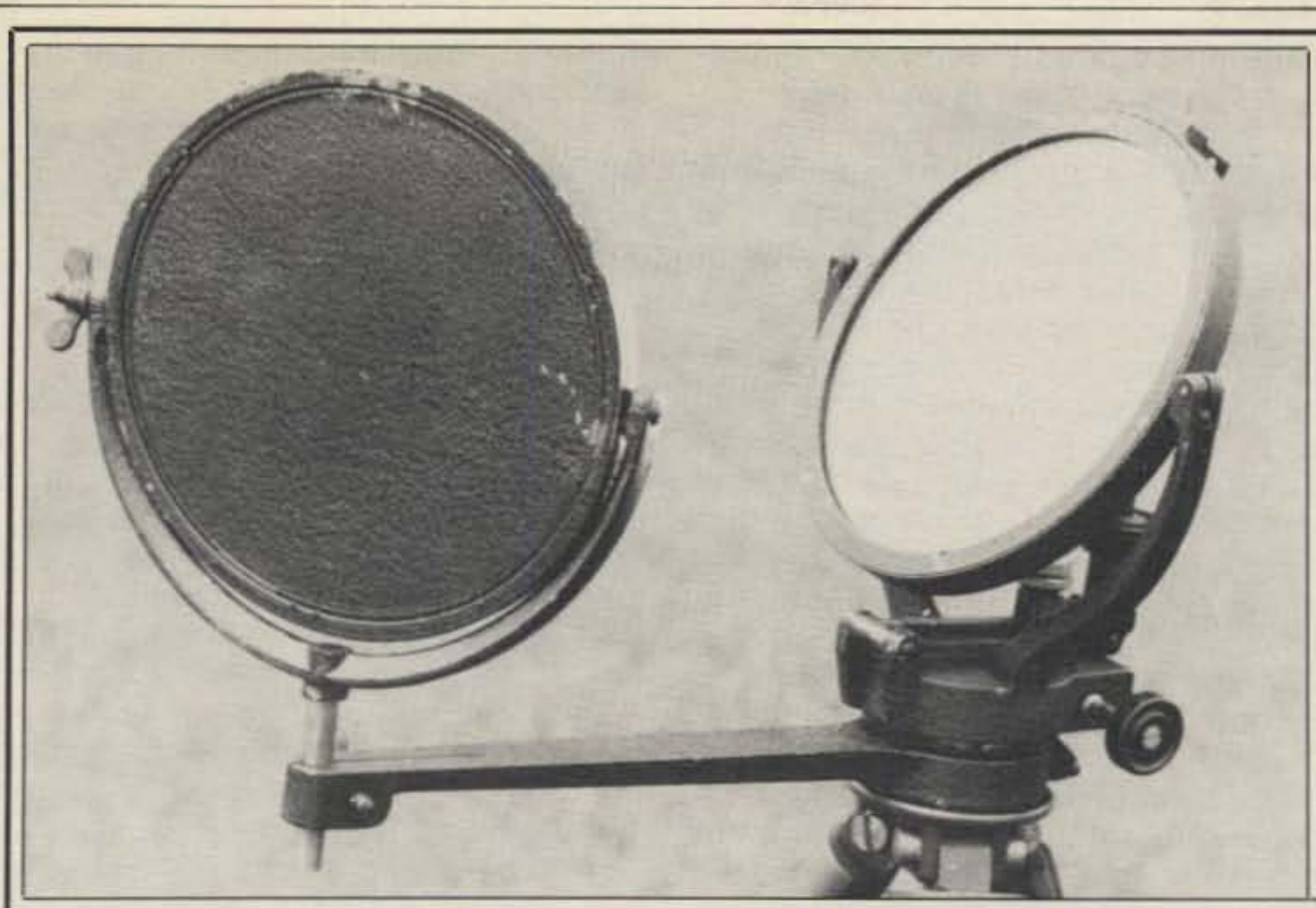
Canadian Mark V heliograph was used in the Canadian army until 1941. It is keyed by mirror deflection and can easily cover ranges of 25 miles in suitable terrain.
