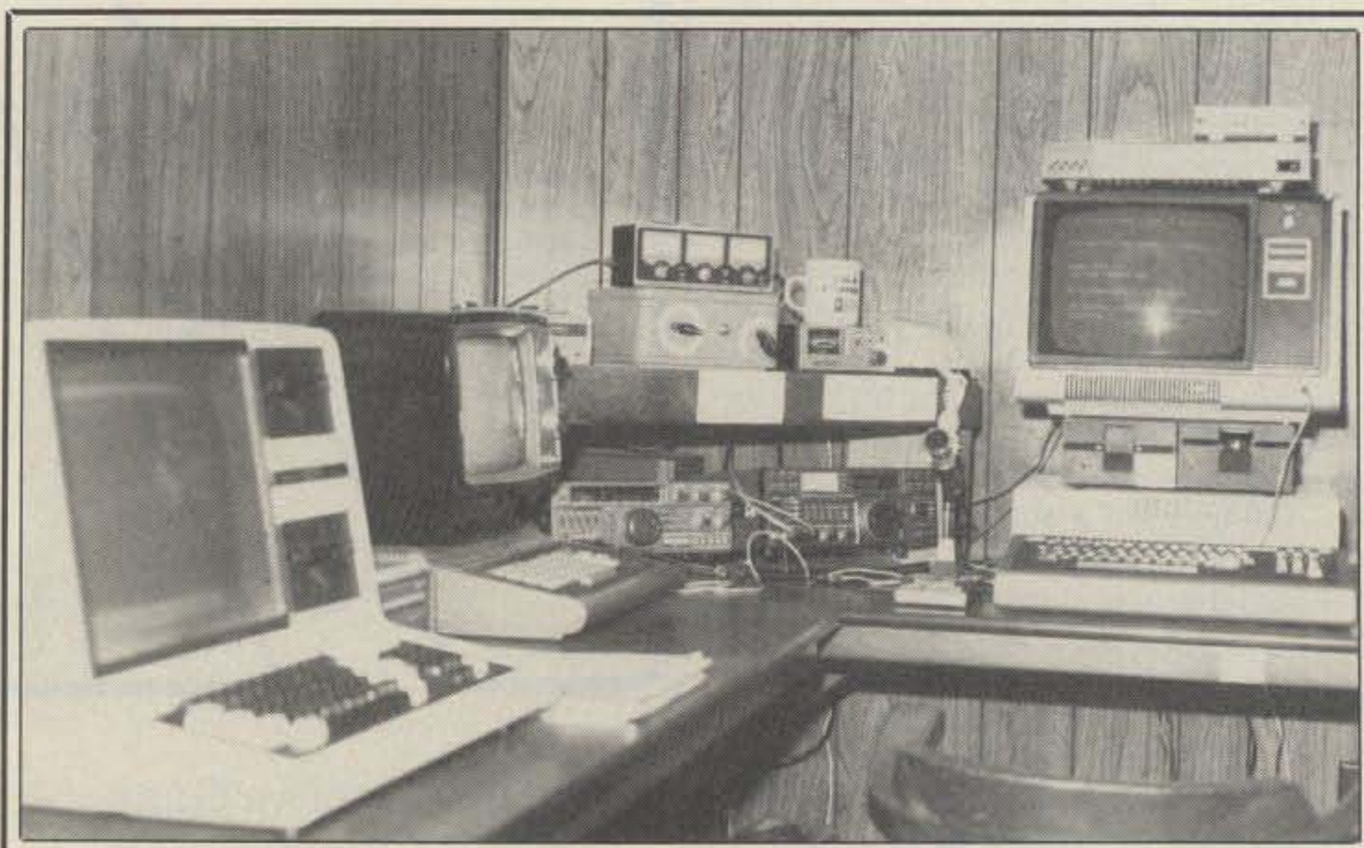
The digital communications station at KR3T. I currently have two separate RTTY stations—a TRS-80 Color Computer with a Kantronics Interface II and a TRS-80 Model IV with a Kantronics KAM.
