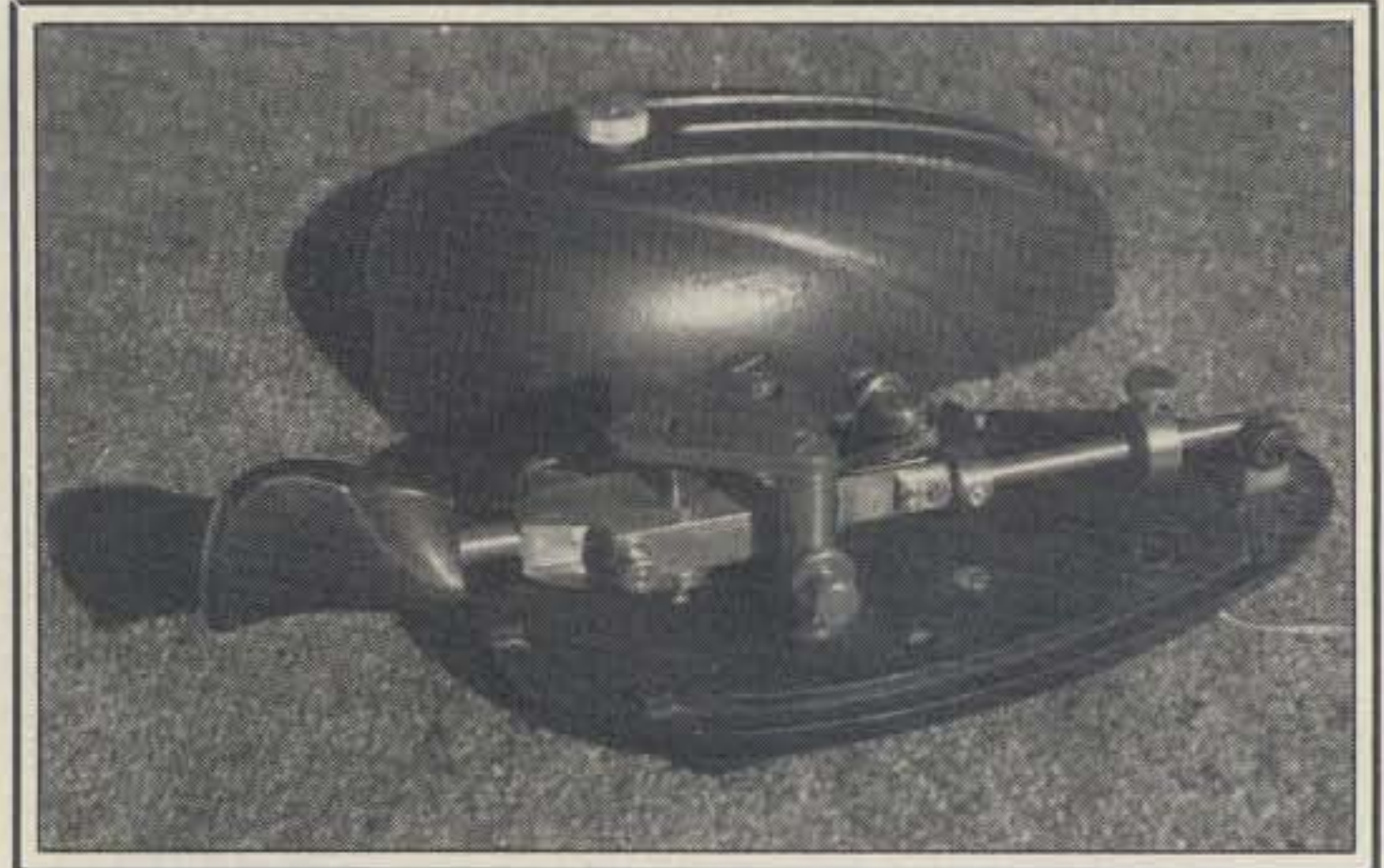
Photo 2— Under-the-cover view of VE7FOU's Eddystone reveals a smooth-working mechanism that handles like a dream. Bug is approximately 8 inches long and is dark gray in color.
