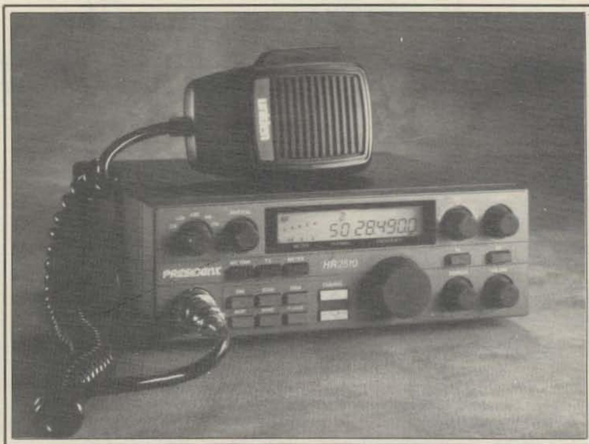
Uniden's new HR-2510 is a compact, all-mode 10 meter transceiver with a sensitive receiver and 25 watt output transmitter.
