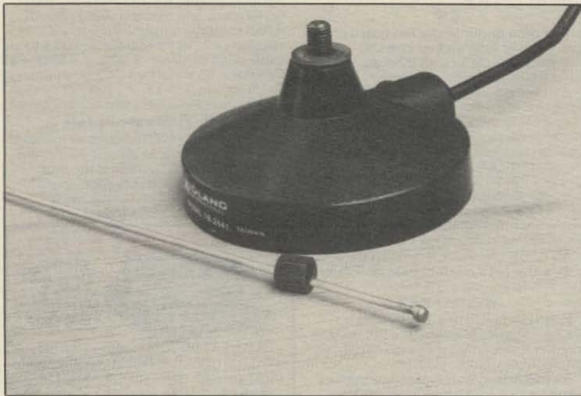
The brass antenna components prior to assembling the whip antenna.
