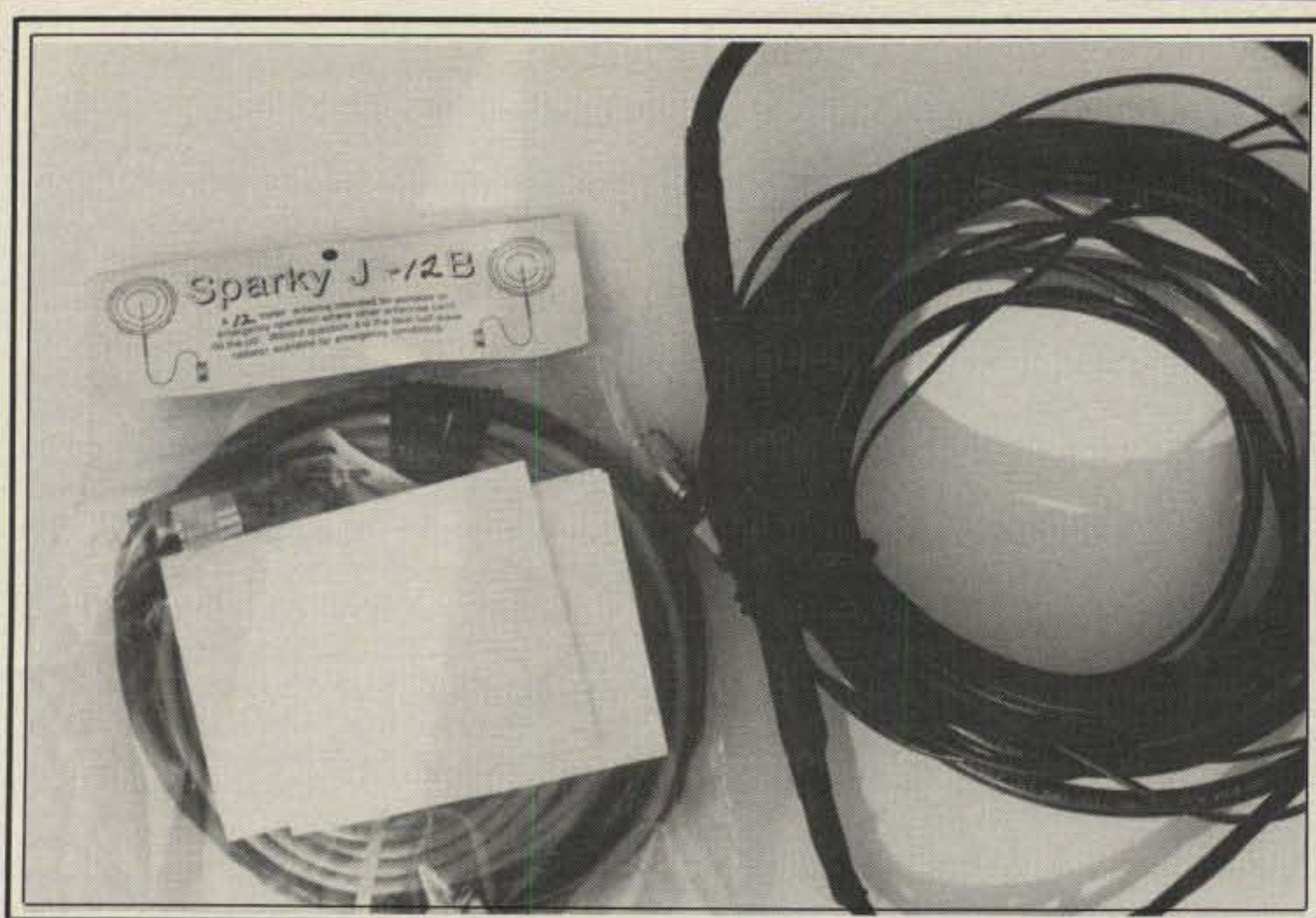
Two Sparky half-wave wire verticals. The 12 meter version on the left was unwrapped and installed immediately after I shot this photo. The 10 meter Sparky on the right was removed from use for this picture. Both antennas work great.
