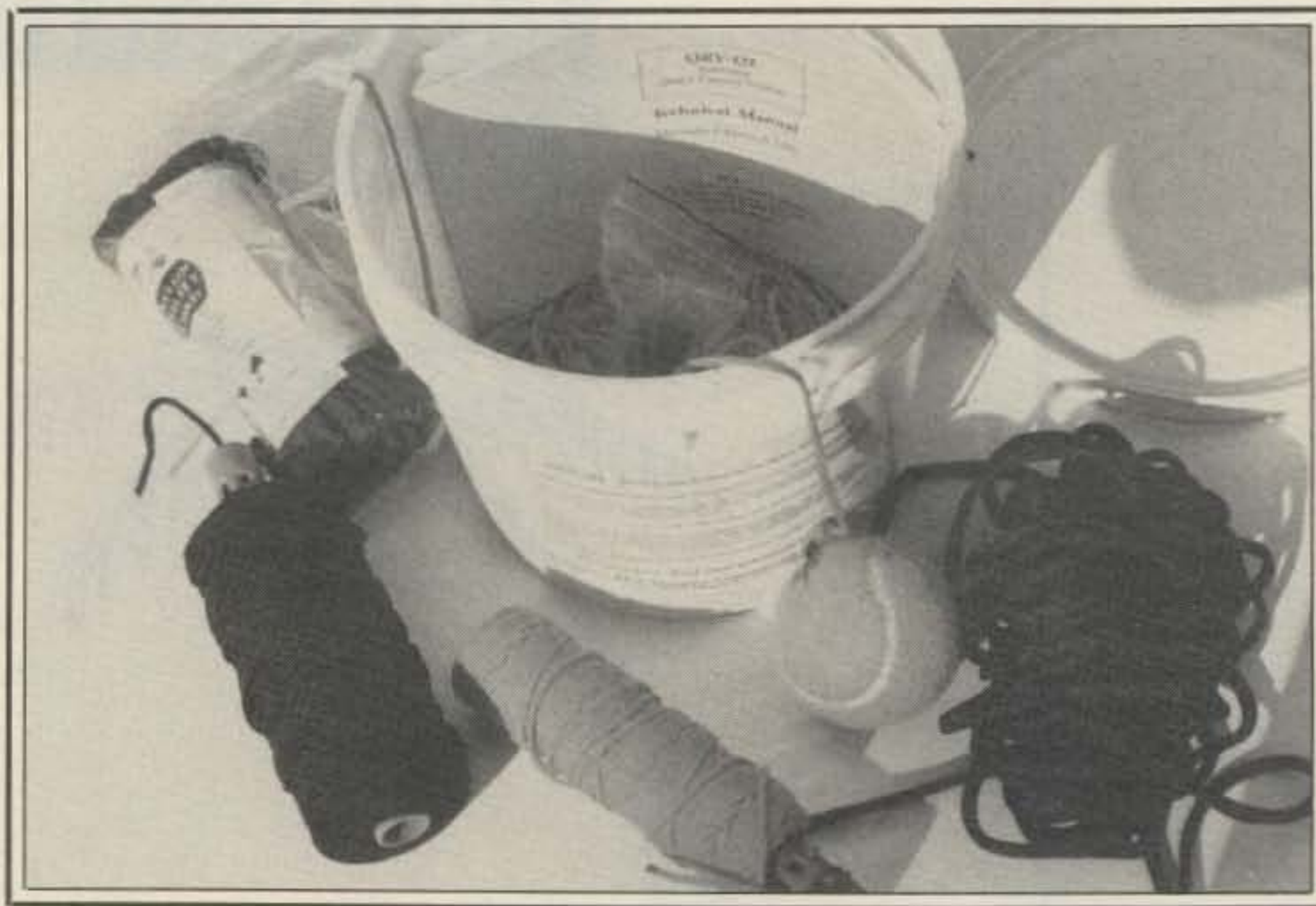
The Antennas West Quick Launch package. Projectile has snap-on safety cover, launch line is very lightweight, and use of the bucket prevents snags. The extra roll of UV-proof double dacron line snuck into the photo during my antenna installation escapes (this is an action photo). Note the manual and spare projectile in the bucket.
