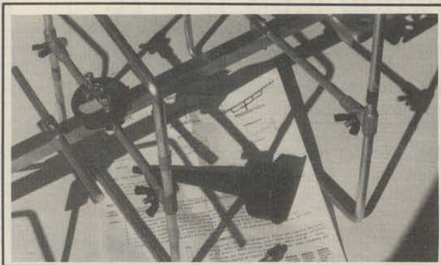
This is a closeup of the loop driven element showing the enclosed balun transformer. The black cone-shaped object is a flexible boot that fits over the balun and feed line to provide weather protection.
