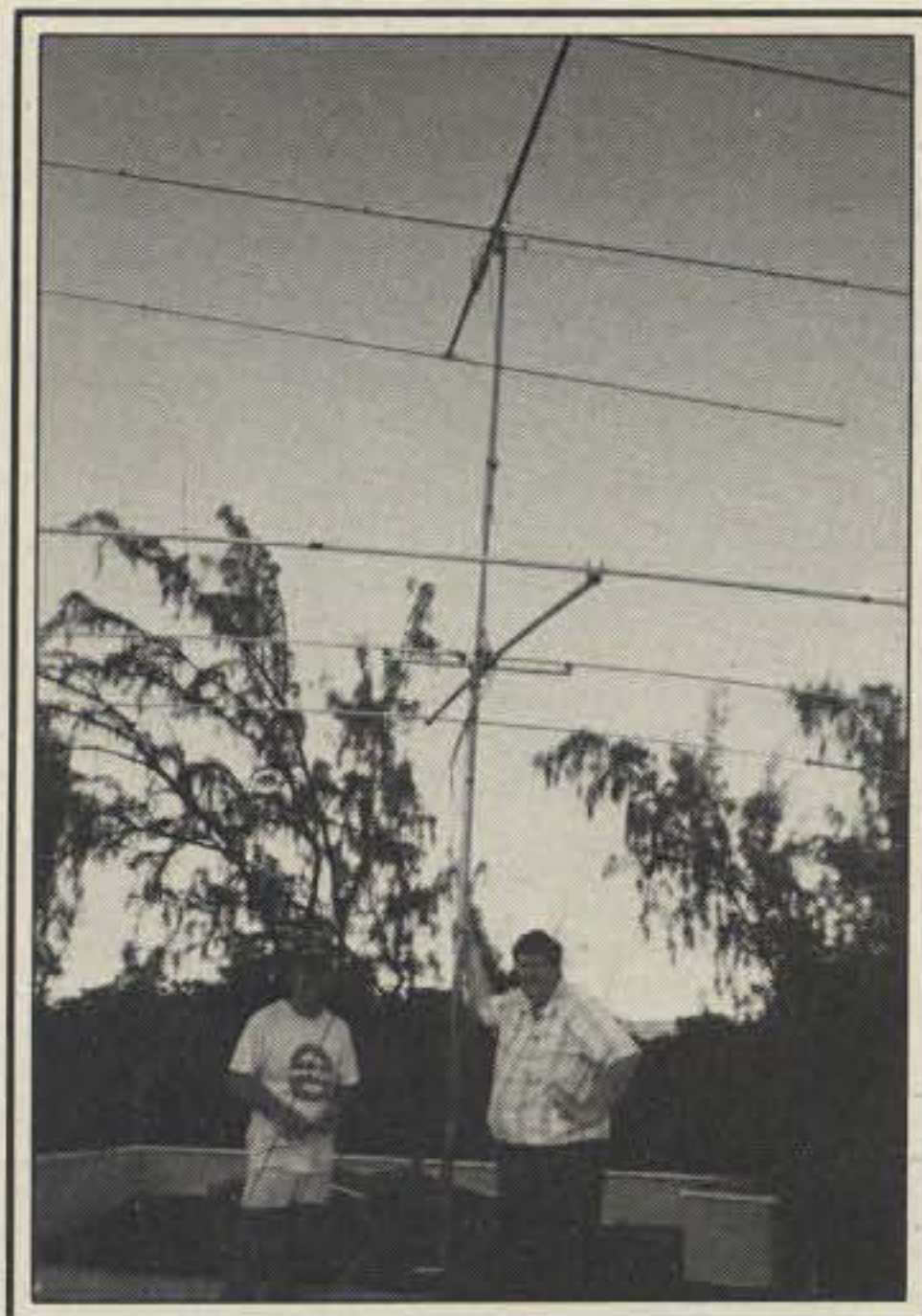
The main antenna system at 8P6BBS. At the top is the Cushcraft 3-element 10 meter beam, with the tribander right underneath. Left to right are Wayne, 8P9FD, and John, 8P9FE.
