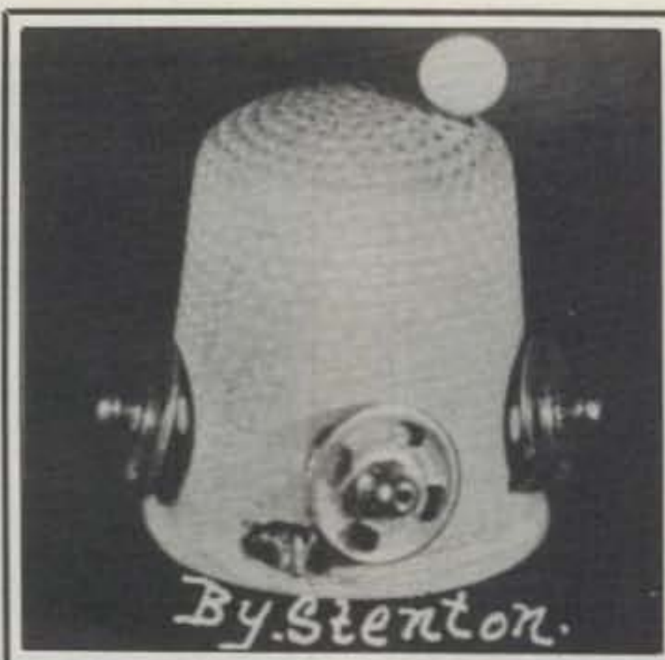
Reg Stofer's thimble radio receiver built in 1925. The white knob on top is a map pin used for tuning the coil inside. Snap fasteners on the sides were used as connectors for earphones, antenna, and ground wire.
