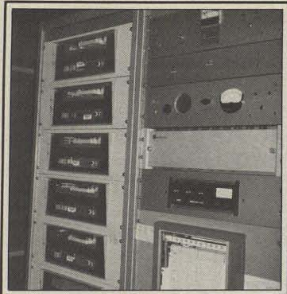
This tape deck at the end of the control panels is used for weather and Pacific storm-warning announcements.
