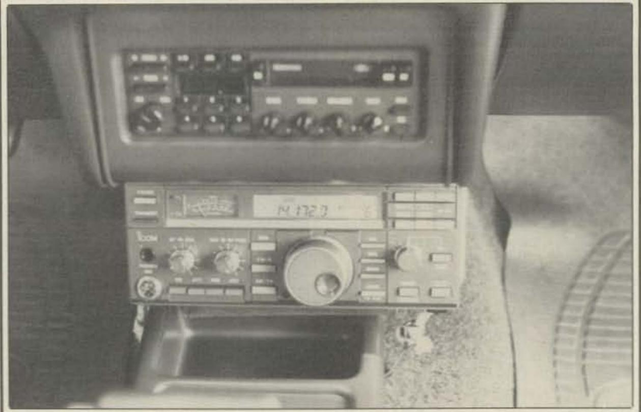
Fig. 4- A compact HF transceiver fits perfectly in the new space. Rear sits on carpet hump, front is cushioned by foam, and bungee cord hooks around rig to secure it in place. A small pad was also taped under the dash center to prevent rig scratches during installation and removal. A light coat is laid over the rig front to divert evil eyes when the car is left unattended.
