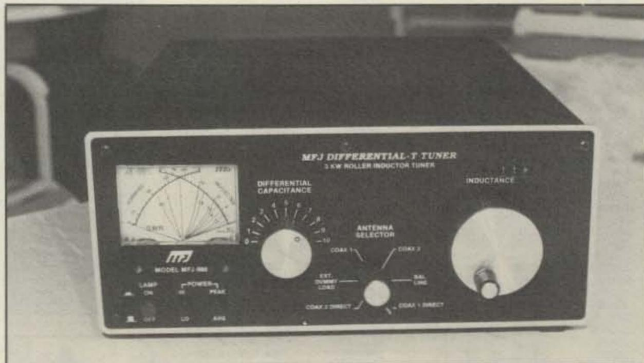
The front panel controls are grouped very logically for ease of operation. A turns counter permits quick resetability of the variable inductor.
