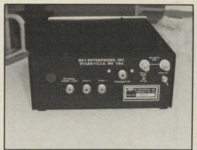
The rear of the tuner contains the various in/out coaxial line connectors and two hefty feedthrough insulators for connection of a balanced line.
