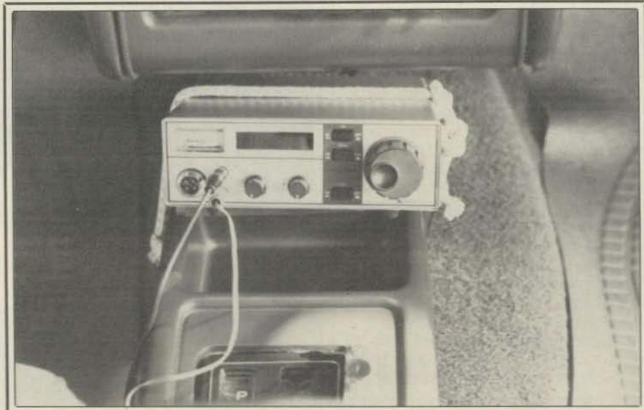
Fig. 5- Tie two knots in the bungee cord to reduce its length, add a DC plug adapter, and a super-small Kantronics KT-130 transceiver fits in the same spot. Two rig mounts in one!
