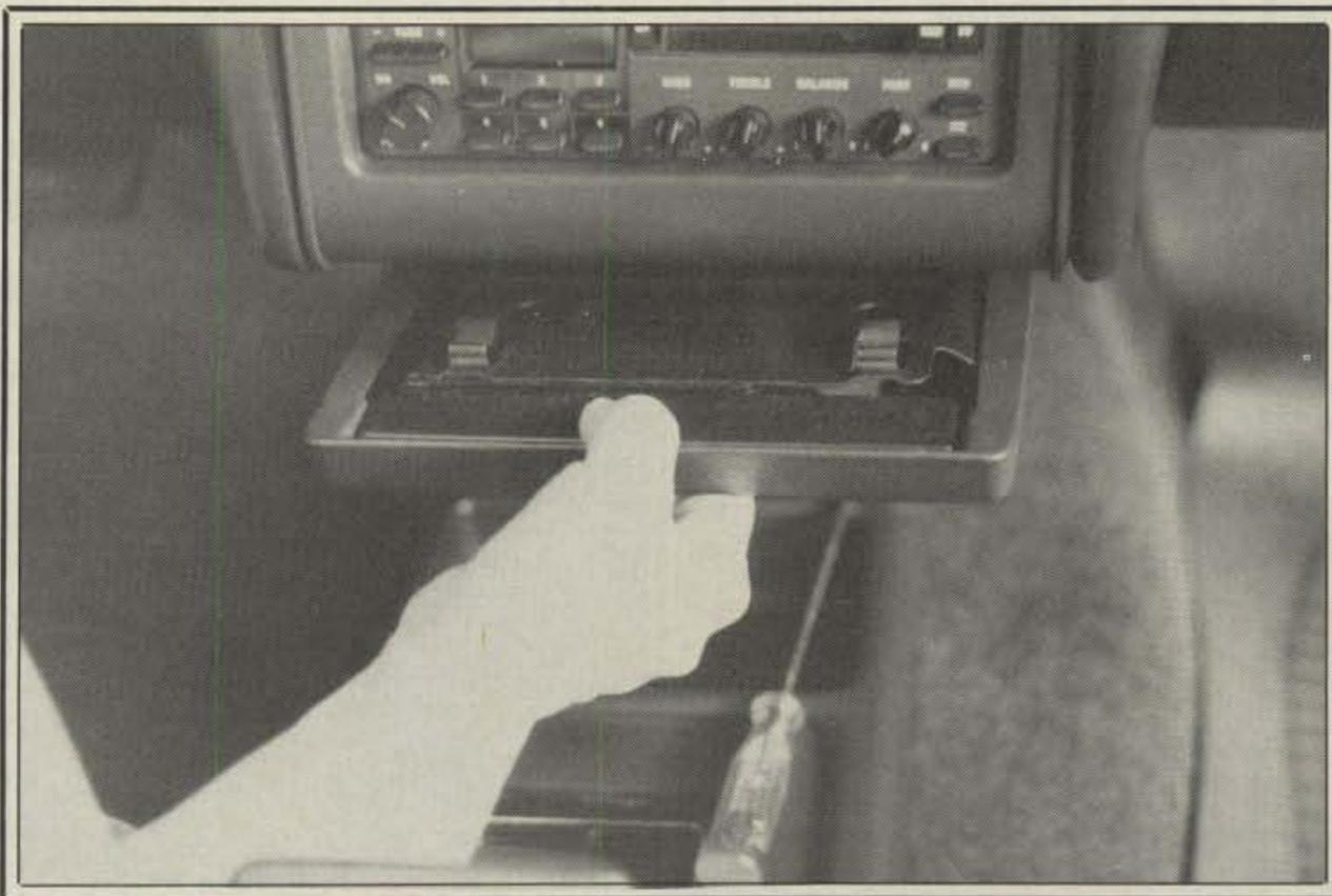
Fig. 3- Our 30 minute installation begins with removal of this compact car's ashtray. Extracting four screws and disconnecting two wires only takes 5 minutes. Similar room-expanding ideas for other car styles are discussed in the text.
