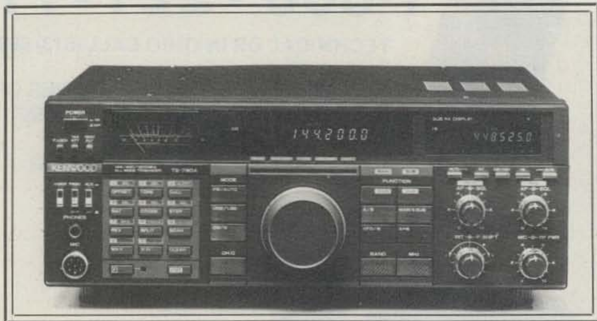
Kenwood's new TS-790A is an impressive-performance, all-mode, and full-duplex transceiver ready for FM, mountaintopping, and OSCAR satellite action.
