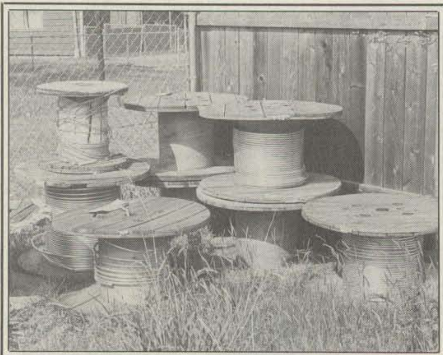
Many partial reels of cable go to waste around CATV companies because they are too short to be strung on poles.
