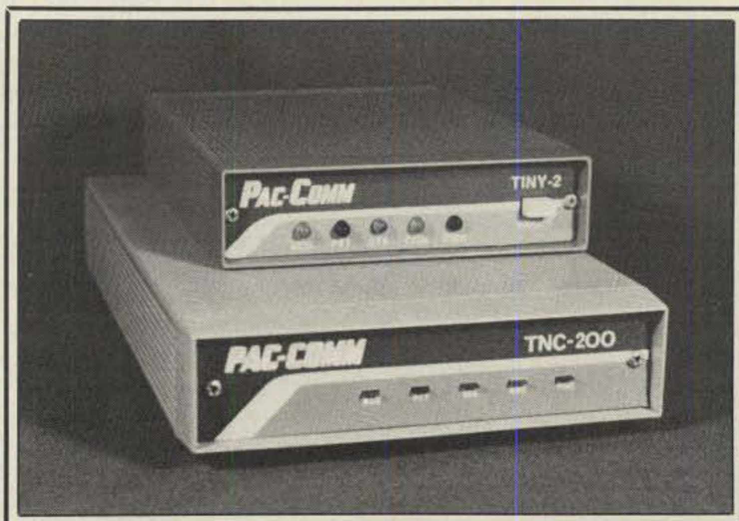
The Pac-Comm TNC-200 and Tiny-2 are both modified TAPR TNC clones.
