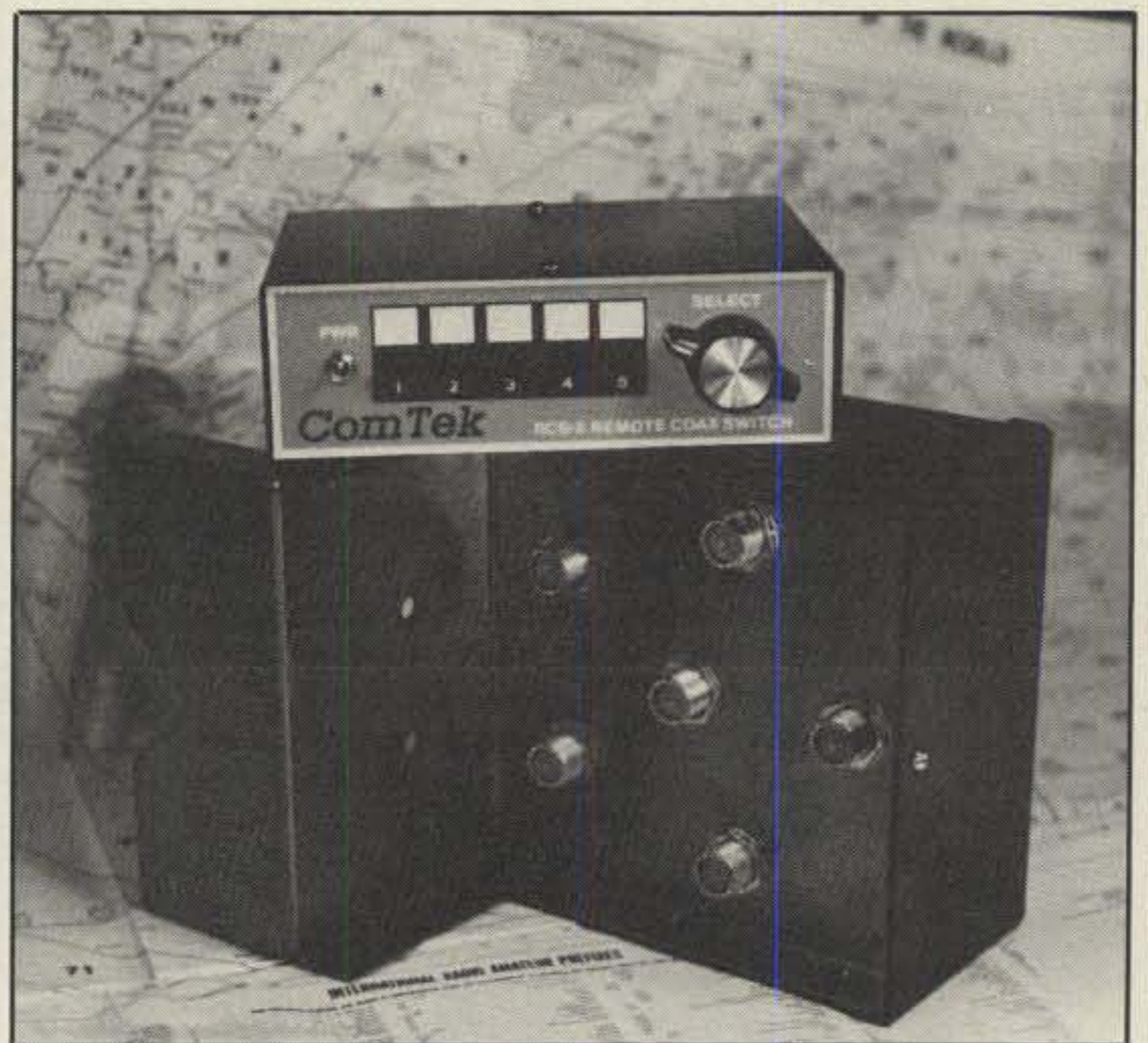
The ComTek RCB-5 Remote Coaxial Control Box switches up to five different antennas from one coax line; you can connect to one or all five antennas at once. The device handles up to 5 KW. (Photo courtesy ComTek)
