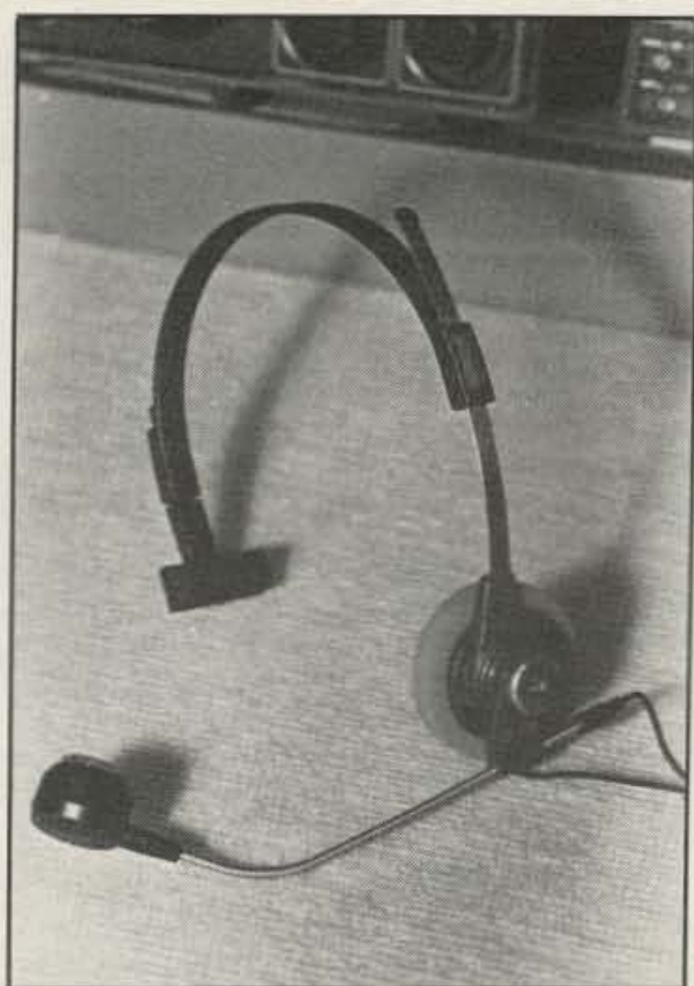
Fig. 2- Heil's new BM-5 single ear headset and boom mic is a fantastic contesting and mobiling aid, especially when combined with VOX operation. Check your state's laws to ensure a one-ear 'phone is acceptable.
