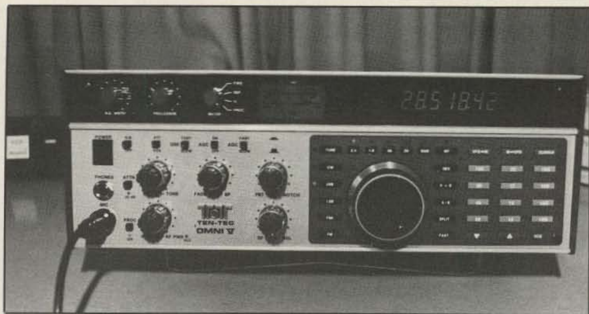
The front-panel layout of the Omni V is very well balanced with an easy-on-the-eyes frequency display, the analog controls on the left, and the large keypad around the main tuning control.
