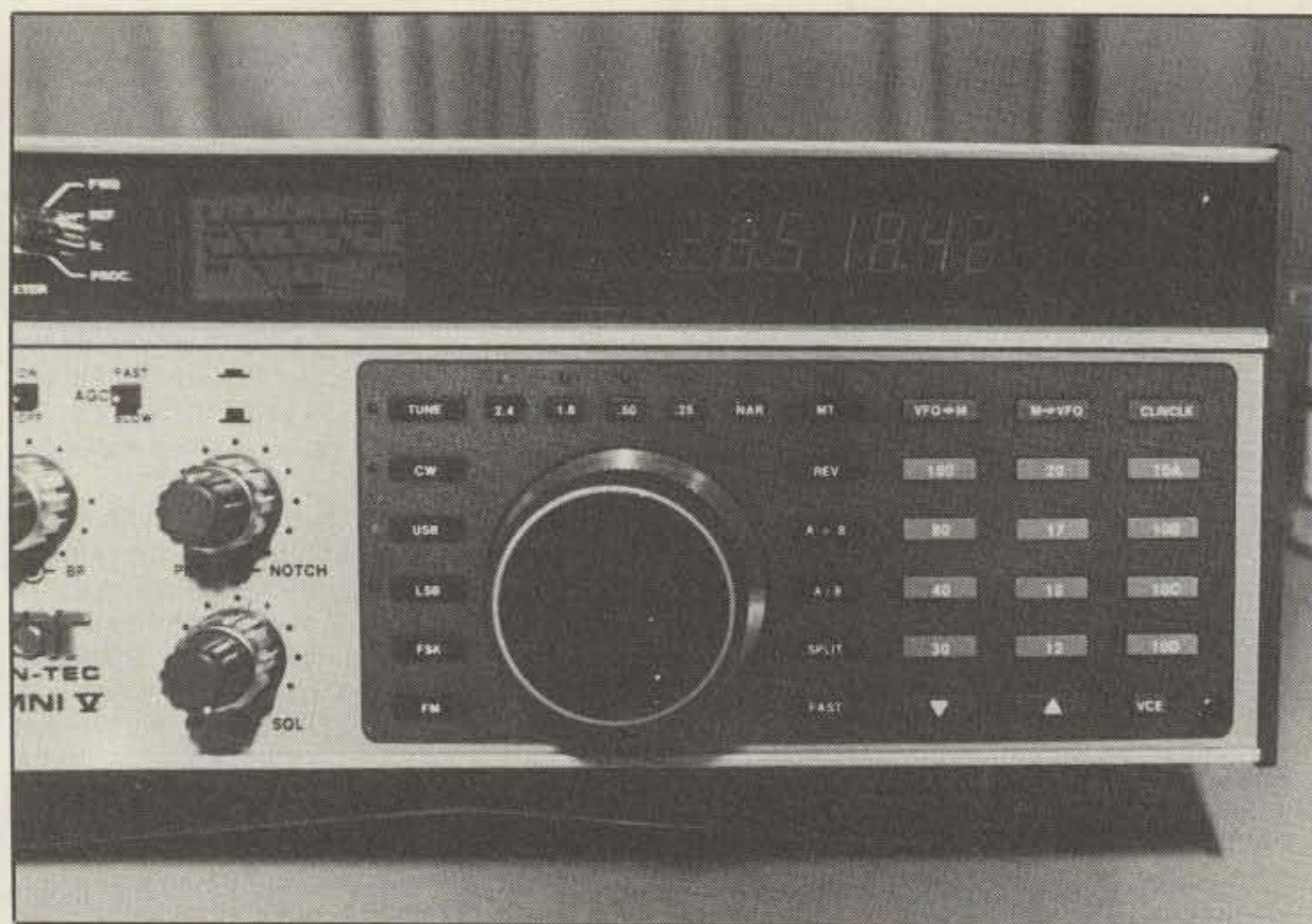
A closer look at the keypad. Except for two keys, each key has a single dedicated function to avoid confusion in operation. It's a very user-friendly arrangement.
