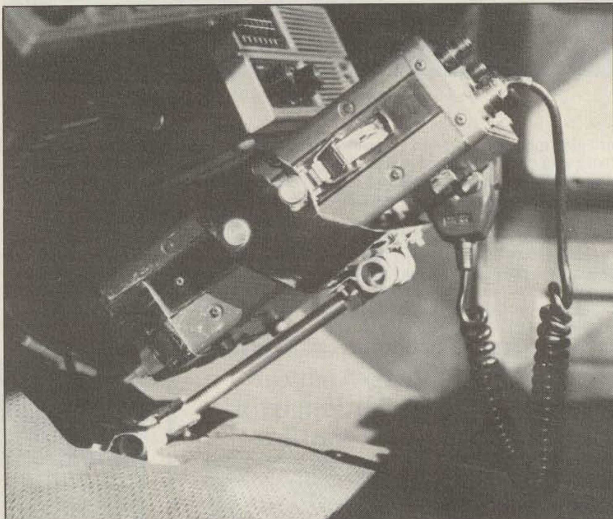
As installed in my pickup, the gimbal mount holds the rig in a convenient position and out of the way at the same time.
