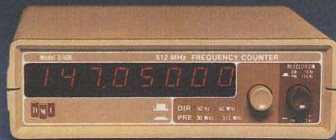
50 Hz to 512 MHz 5¼ X 5 X 1½ 1 PPM ACCURACY TCXO
