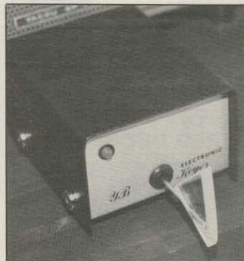
The completed key is housed in a metal cabinet with the keyer circuitry. Operating controls are on the rear.
