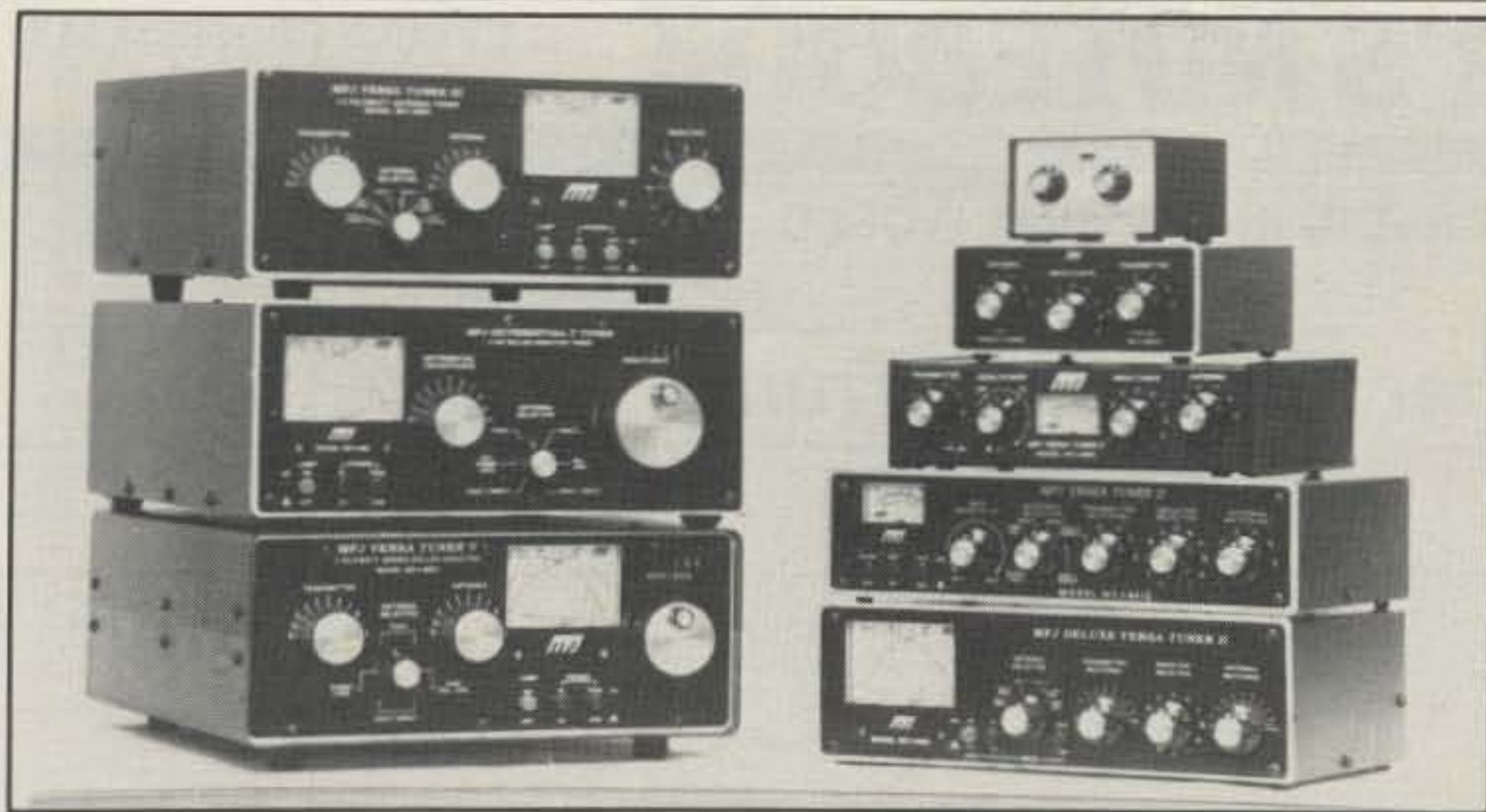
Included in this photo are several of the MFJ tuners which incorporate the new MFJ peak-and-average-reading cross-needle SWR/wattmeter. MFJ tuners with the new peak reading include the MFJ-949D, MFJ-962C, MFJ-986, and MFJ-989C. (Photo courtesy MFJ Enterprises)
