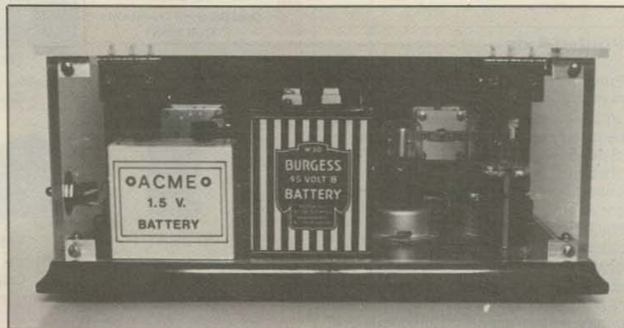
Fig. 2 - Rear view of W8WVM's Globe Trotter. Batteries are homebrew covers with replaceable "innards." Coil forms were on-hand items, and tube sockets are raised above the base with aluminum shells. Rig is enclosed in a clear plastic case with hinged top. Little portable works quite well after big-band music clears from its nostalgia-filled grids.
