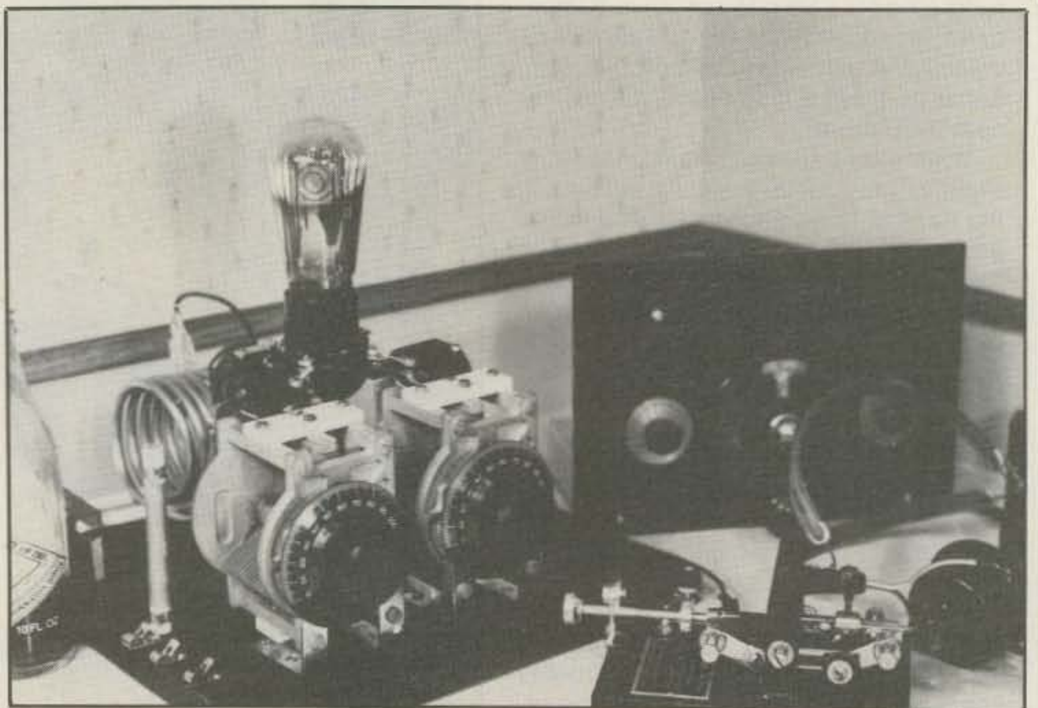
Fig. 7- My home re-creation of the Gil Classic transmitter beside its mating two-tube regenerative receiver. Note bug, Baldwin earphones, and pocket frequency counter for checking and zeroing frequencies. Now this is the way to work 30 meters in style! The operator, not the rig, makes the difference.
