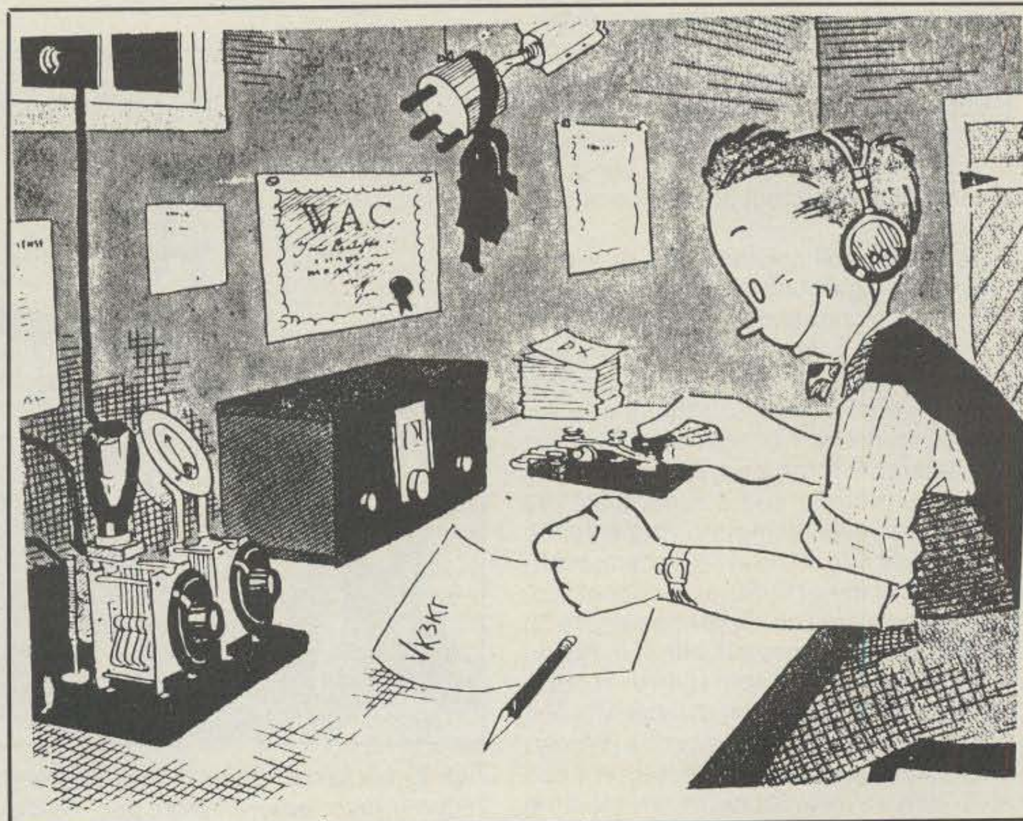
Fig. 5- Famous Gil cartoon that inspired construction of its 1929-style transmitter. Look at that black board, top-mounted tube, upright RF choke, and flanking condensers with twin velvet vernier dials. A genuine classic for sure!
