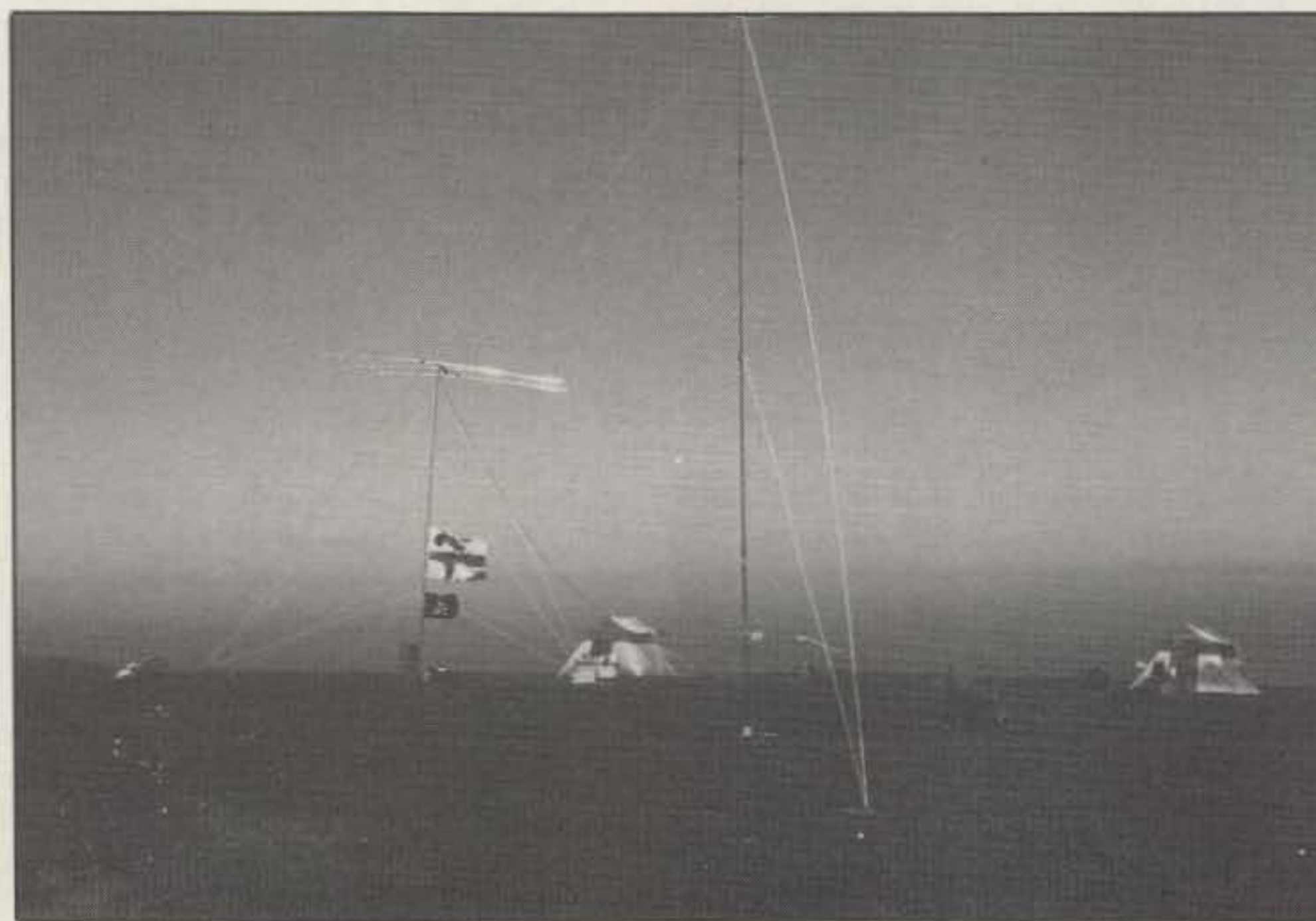
Consisting of two tents, the SSB and low-band site was located at the northern end of the island and featured a Cushcraft A3, a Butternut HF6V, and a special 80/160 meter ground plane. It was like a lunar landscape with the suffering EUs booming in from over the horizon.
