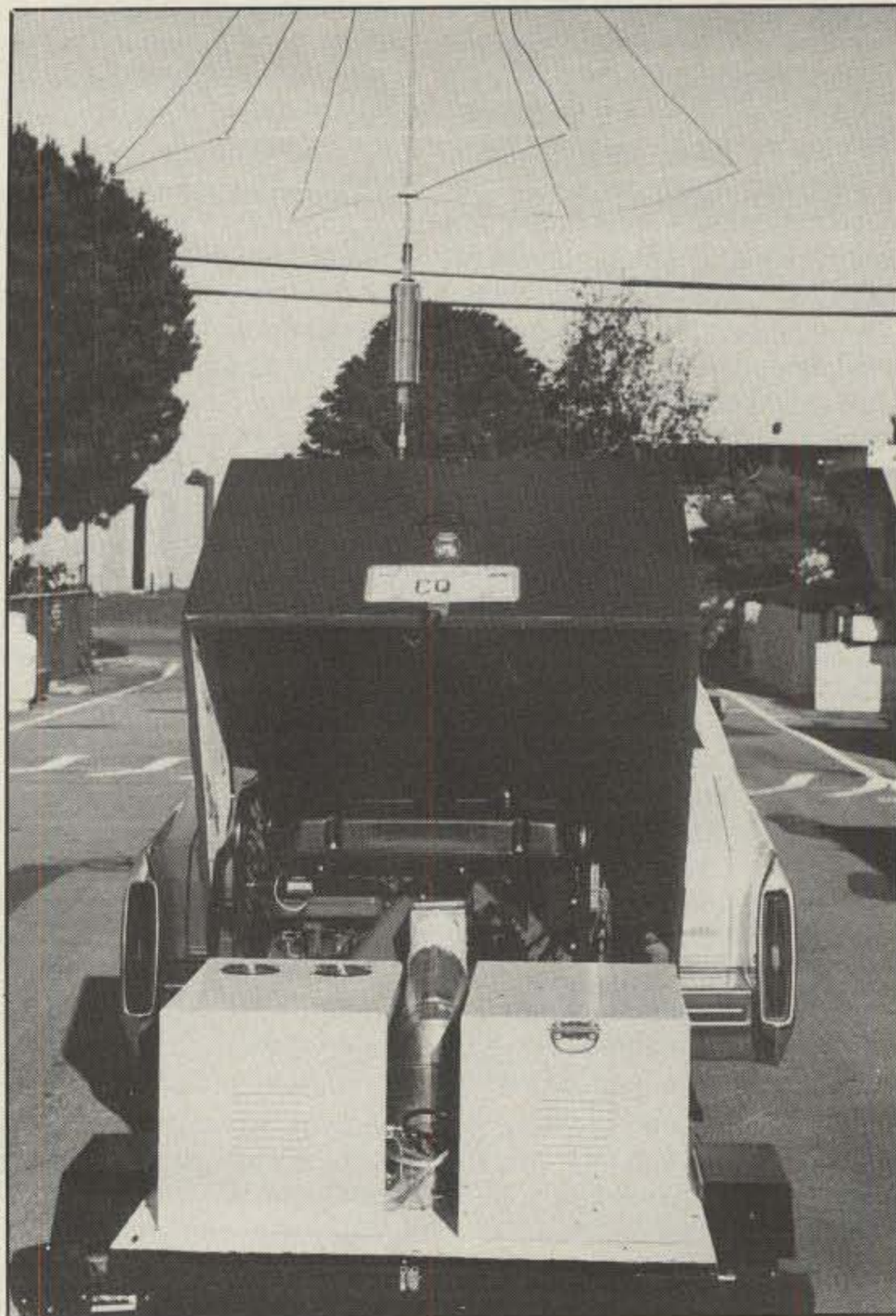
Fig. 2— Once the trailer hood is lifted, the reason behind the big signal becomes evident. No, it's not our spare clothes. It's the reason receivers cringe in fear—a multi-band KW-plus mobile amplifier able to move anywhere, even park in front of your house.
