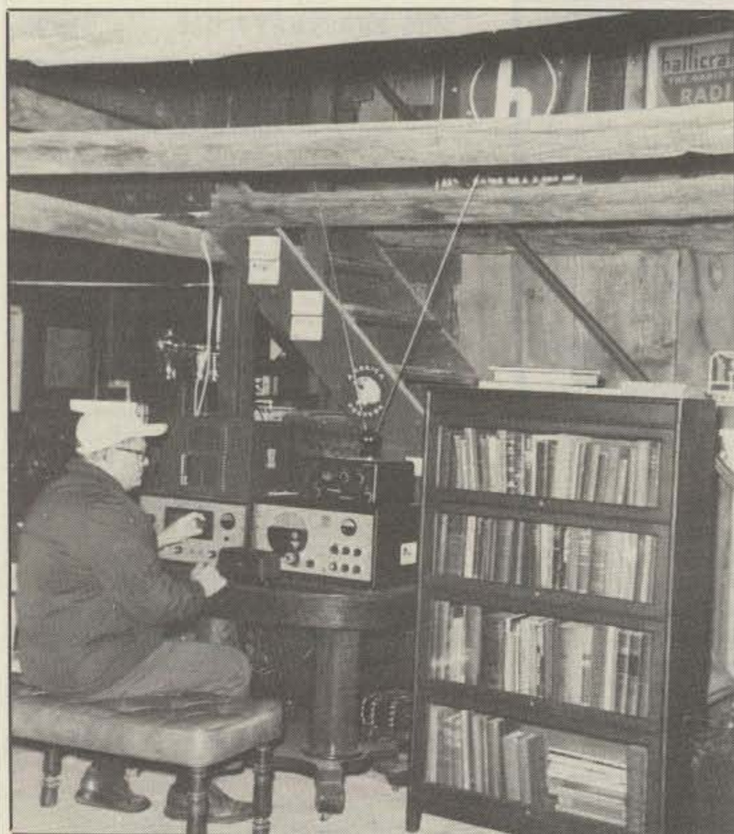
Clarence Smith, KA8PJN, is a farmer in Spring Lake, Michigan. He has this 1940s-era Hallicrafters amateur radio station set up in his barn. It includes an HT-19 transmitter, SX-42 receiver, SP-44 panadapter, and a PM-23 loudspeaker.
