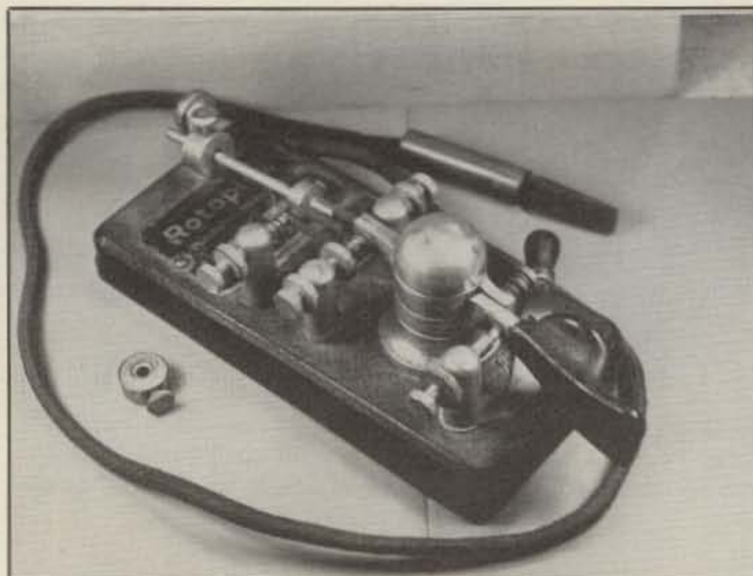
Photo 12- A rare Martin Rotoplex. Complete yoke turns on an enclosed ball-bearing assembly to make dits and dahs. (Owned by W2GDV)
