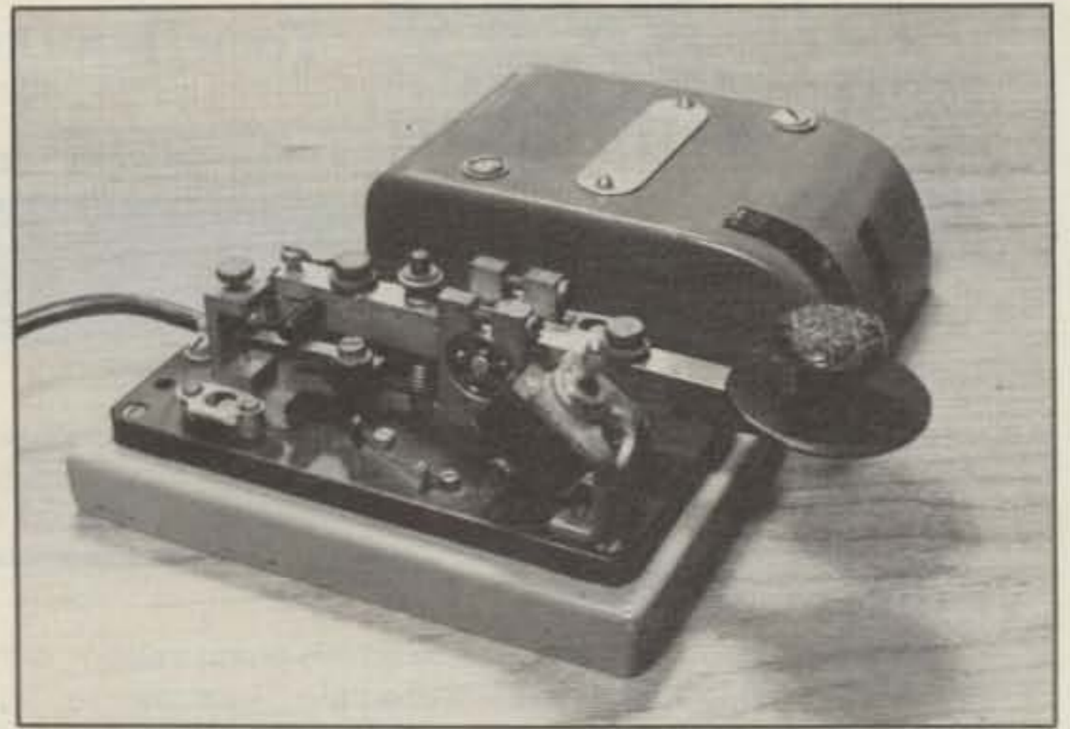
Photo 6- English key with heavy marble base, ball-bearing fulcrum, and rugged cover. This item even has a built-in T/R switch! (Photo via JN1GAD)
