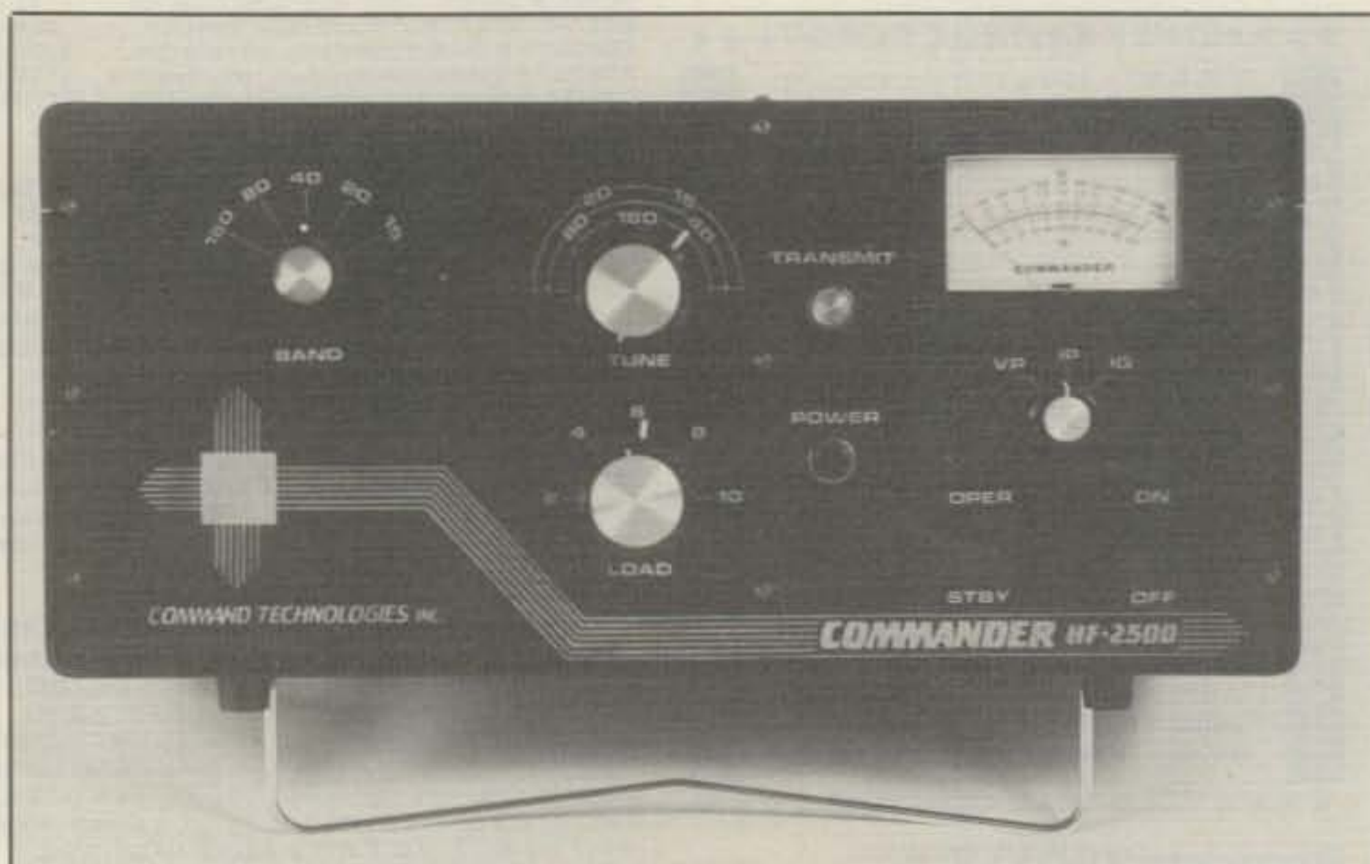
This is the front-panel view of the HF-2500. At the upper left is the band switch. To the right are the TUNE and LOAD controls. There are two lights, one indicating AC power is on (green) and another showing you are in the transmit mode (red). The OPERATE-STANDBY switch is also an exciter-only switch. In the standby position the exciter is connected straight through to the antenna.
