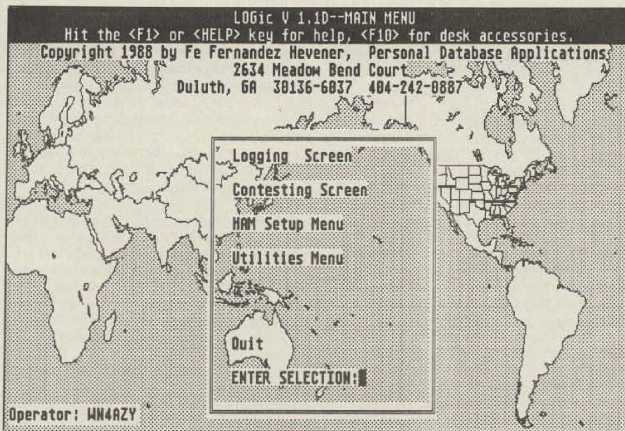
Fig. 1—Shown here is the LOGic Main Menu, which provides access to the four major areas of the program—logging, contesting, setup, and utilities. The graphic screen shown here is actually from the Atari ST version; the IBM version does not have the world map.
