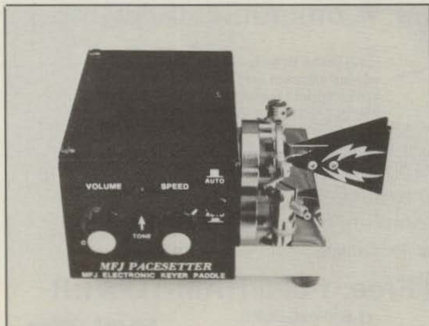
Photo 1- Check out the custom fingerpieces on this keyer. VE7FOU made them by inlaying mother-of-pearl lightning bolts in polished plexiglas. (K4TWJ keyer and photo)
