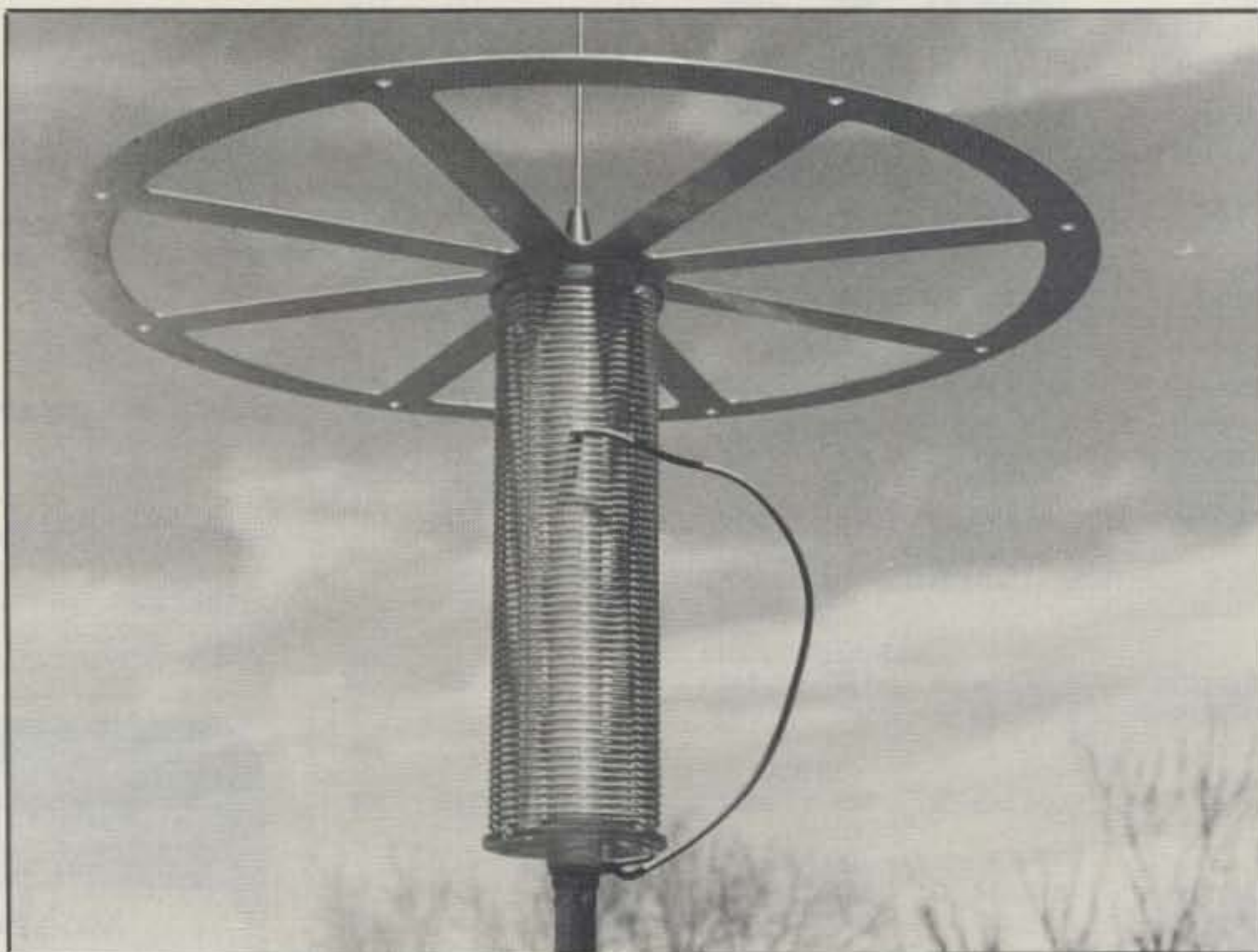
Here is a close-up of the center, or loading, coil and the capacitive hat. Note the excellent construction. The adjustable tap is visible in this shot.
