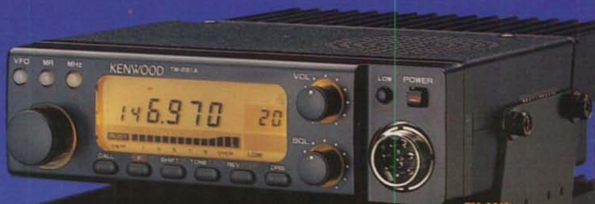
TM-231A 136-174 MHz receive, TX on Amateur bands only. Modifiable for MARS/CAP. Permit required.
