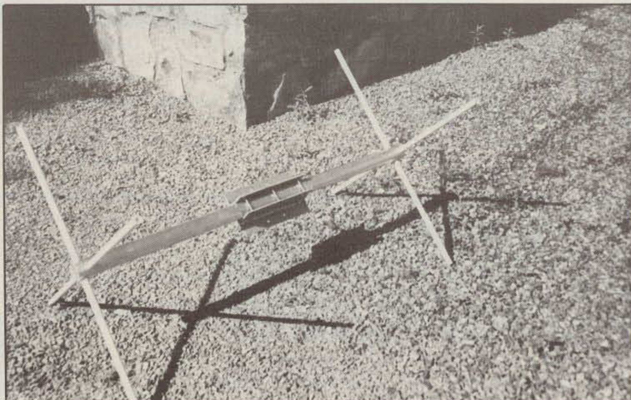
Here are the boom and element supports. The fiberglass supports are "locked" into the boom with nuts and bolts.
