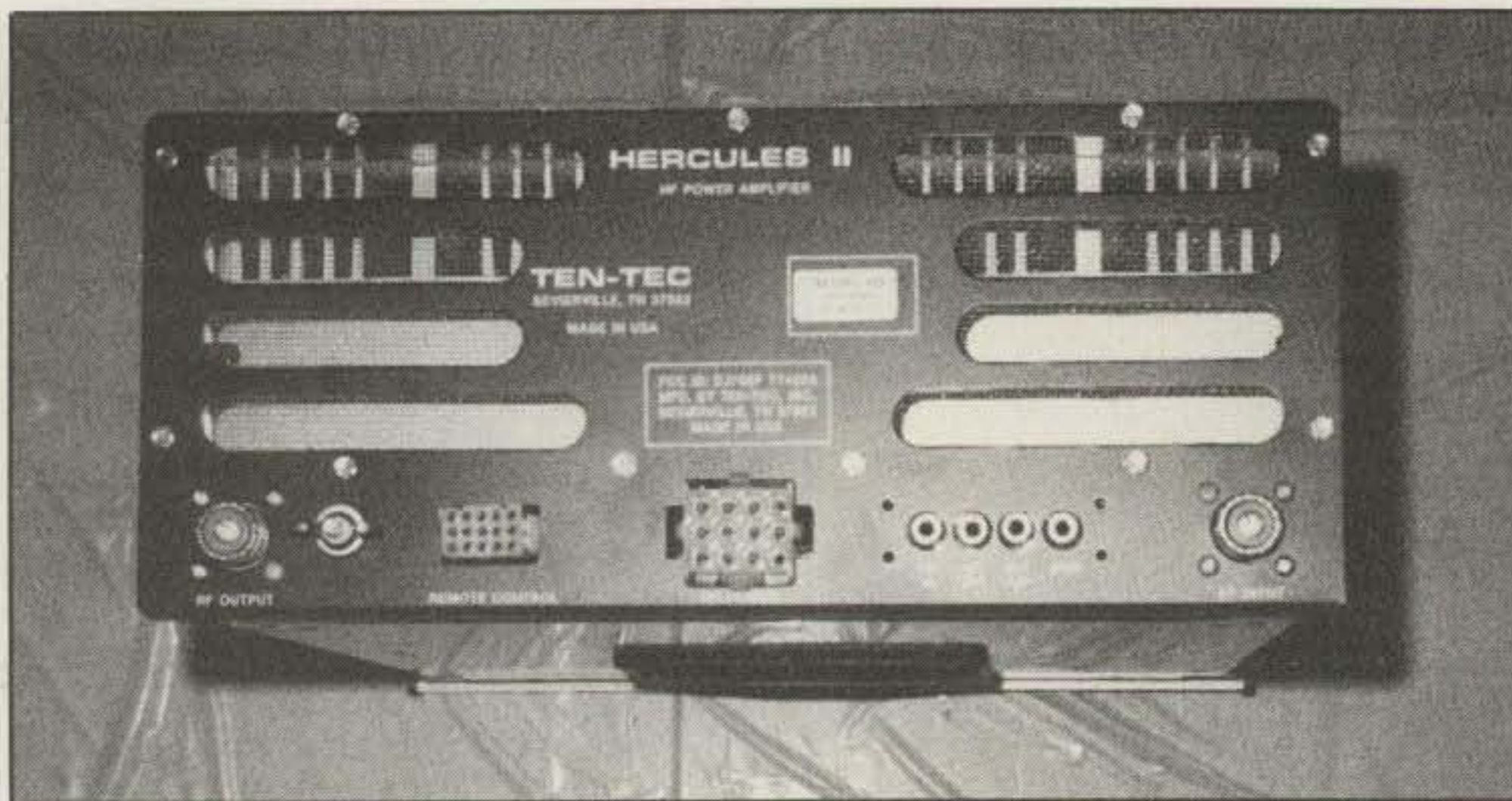
The rear-panel connections are quite simple with the usual RF in/out connections and keying connections for simple PTT, semi-QSK, or full QSK operation. The large Molex-type connector (center) is for a power source connection, while the smaller connector to the left of it is for a remote-control connection. The two SO-239 RF connectors are each fastened with four sets of hardware, a touch rarely found any longer!
