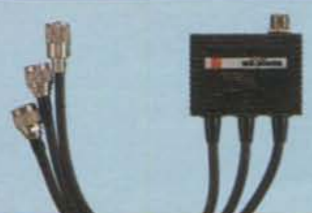
MX-3000N Triplexer with N connectors and UHF connector for HF, 2m, 70cm and 23cm bands ●Coaxial cable : 5D2VS 35cm
