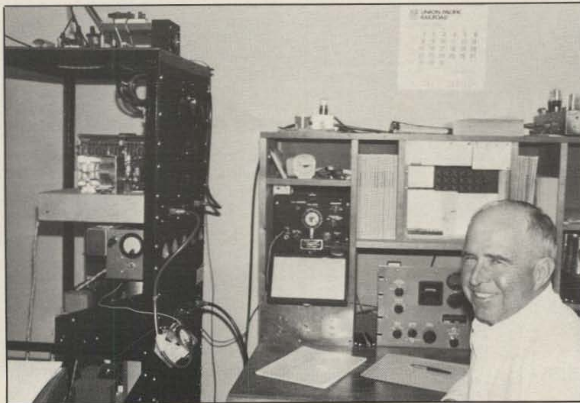
You don't need modern, state-of-the-art equipment to work all zones on 40 meter CW, as Dan Knipe, W7IGE, proves. Dan runs a pair of 35TGs at about 150 watts output from his home-brew amp, feeding a two-section W8JK dipole.
