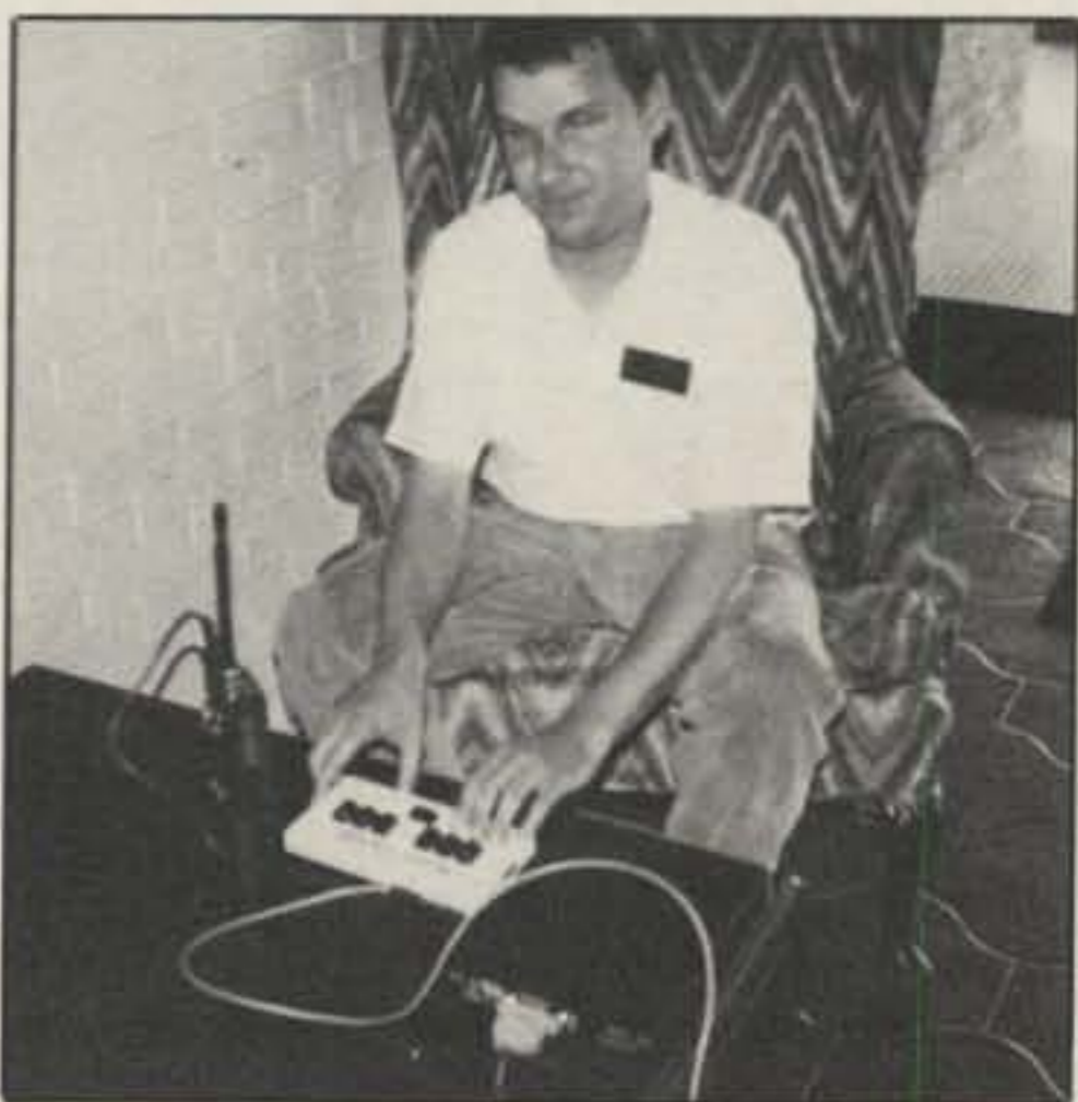
Dana, N4PGE, demonstrates the "Braille 'N Speak" for us. The "Braille 'N Speak" is connected to the RS-232 port of the MFJ-1274 in much the same manner as a terminal would be. The incoming data from the MFJ-1274 is fed to the "Braille 'N Speak," where the voice synthesizer converts the data to words.
