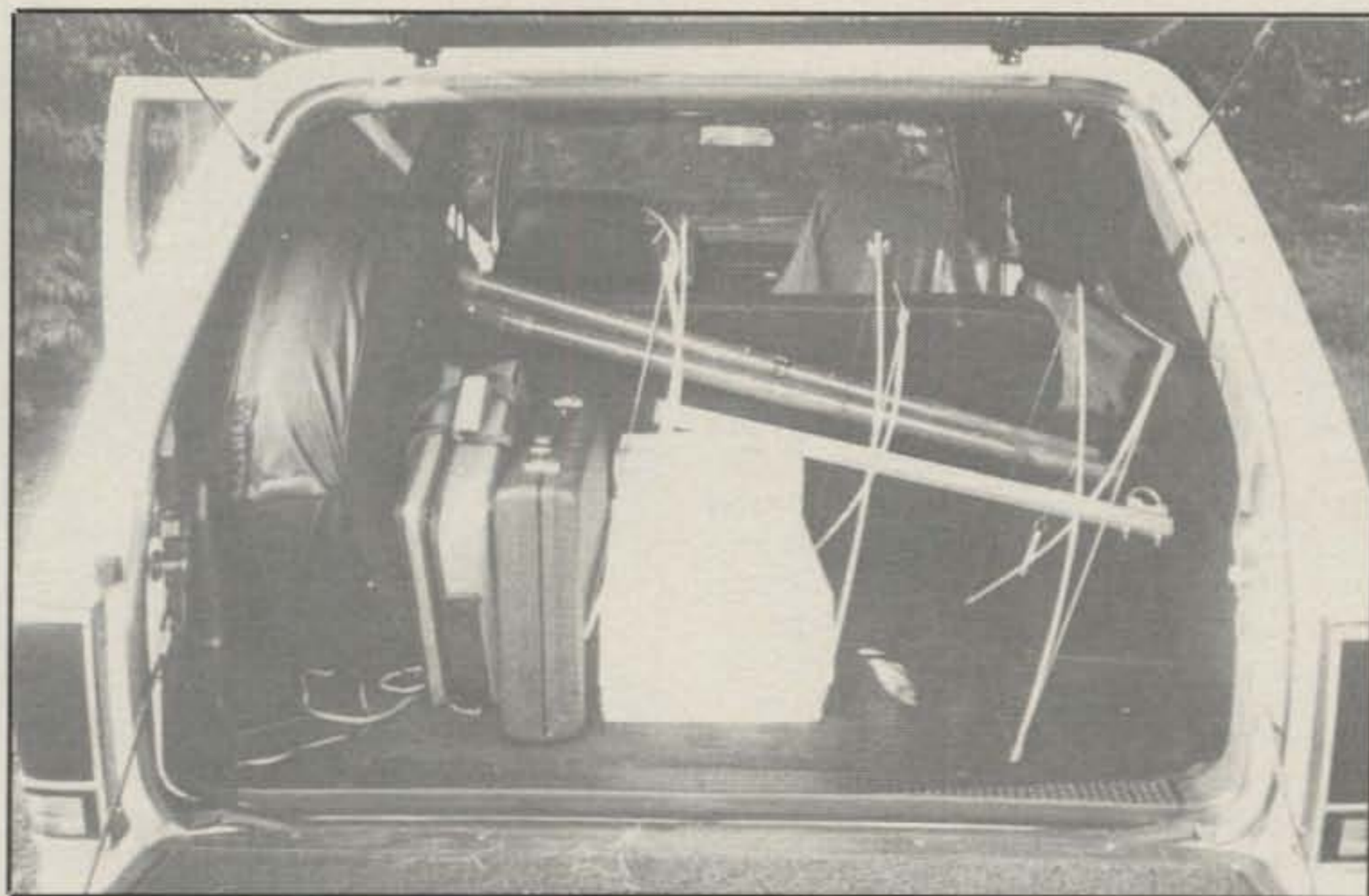
For field-day purposes I ran a special line (fused) to the rear of the Blazer from the vehicle's heavy-duty electrical system (the cable visible beneath the spare tire). For added protection a separate switch at the battery controls the power to the line.
