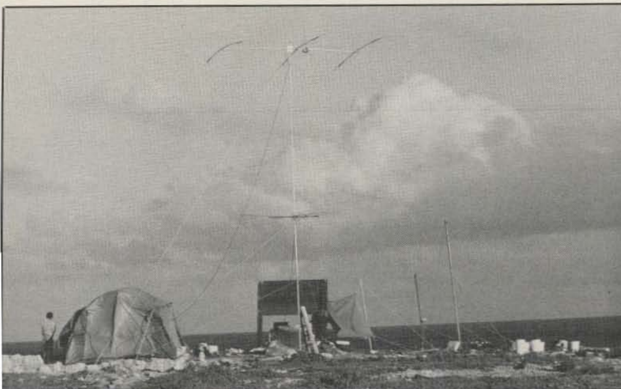
Site 1—The Cushcraft A3 tribander is about 60 feet above the water. Most of our phone contacts were made from here.
