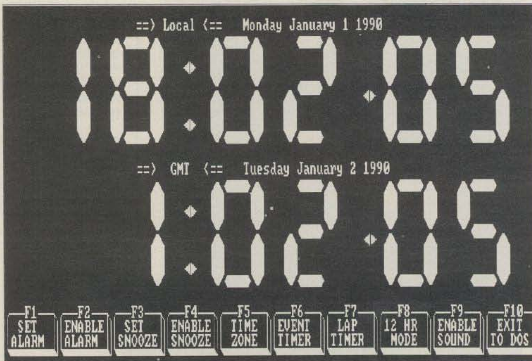
Fig. 2- Shown here is the HAM-TIME Main Clock Menu. It displays the local and GMT time, along with the correct date for each. The major function keys are shown at the bottom of the screen. You also can access three additional menus from this menu: the Event Timer, Lap Timer, and Time Zones Menus. (Screen display courtesy ECode Systems, Inc.)
