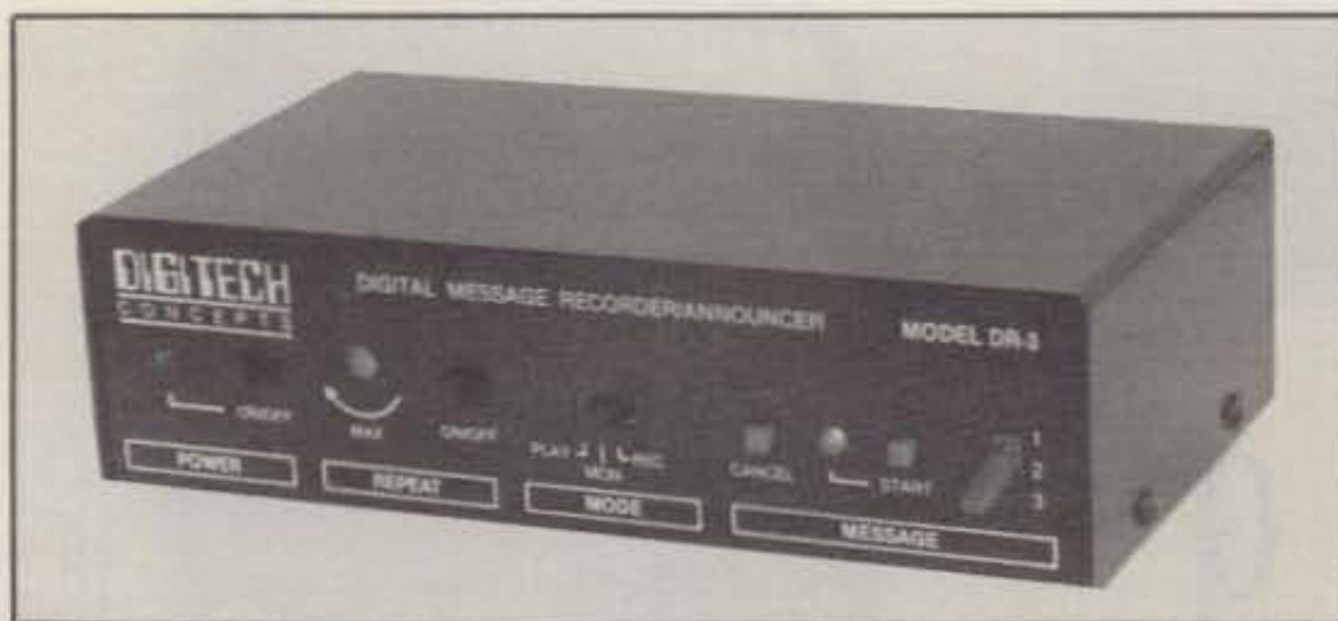
Photo 6- This new digital voice recorder/player is the SSB equivalent of a CW memory keyer. Press one button and it makes those DX calls for you.
