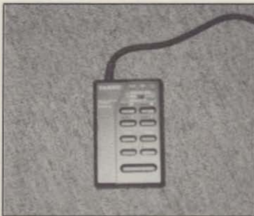
The DSV-2 is a small (2½ x 4 x 1 inch) solid-state digital voice recorder/playback unit. It interfaces with the FT-1000 via a single cable/connector and provides off-air recording, recording from the microphone used with the FT-1000, and the on-air playback or recorded messages.
