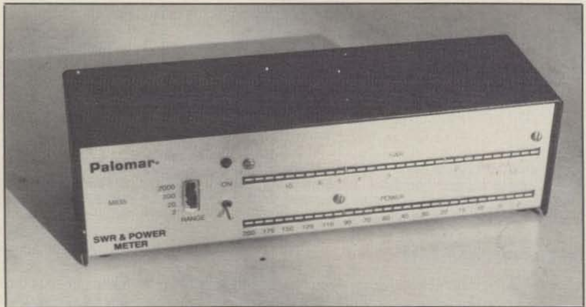
Front-panel view. On the left is the switch for changing the various power levels. The upper line of LEDs is for SWR, and the lower is for power.
