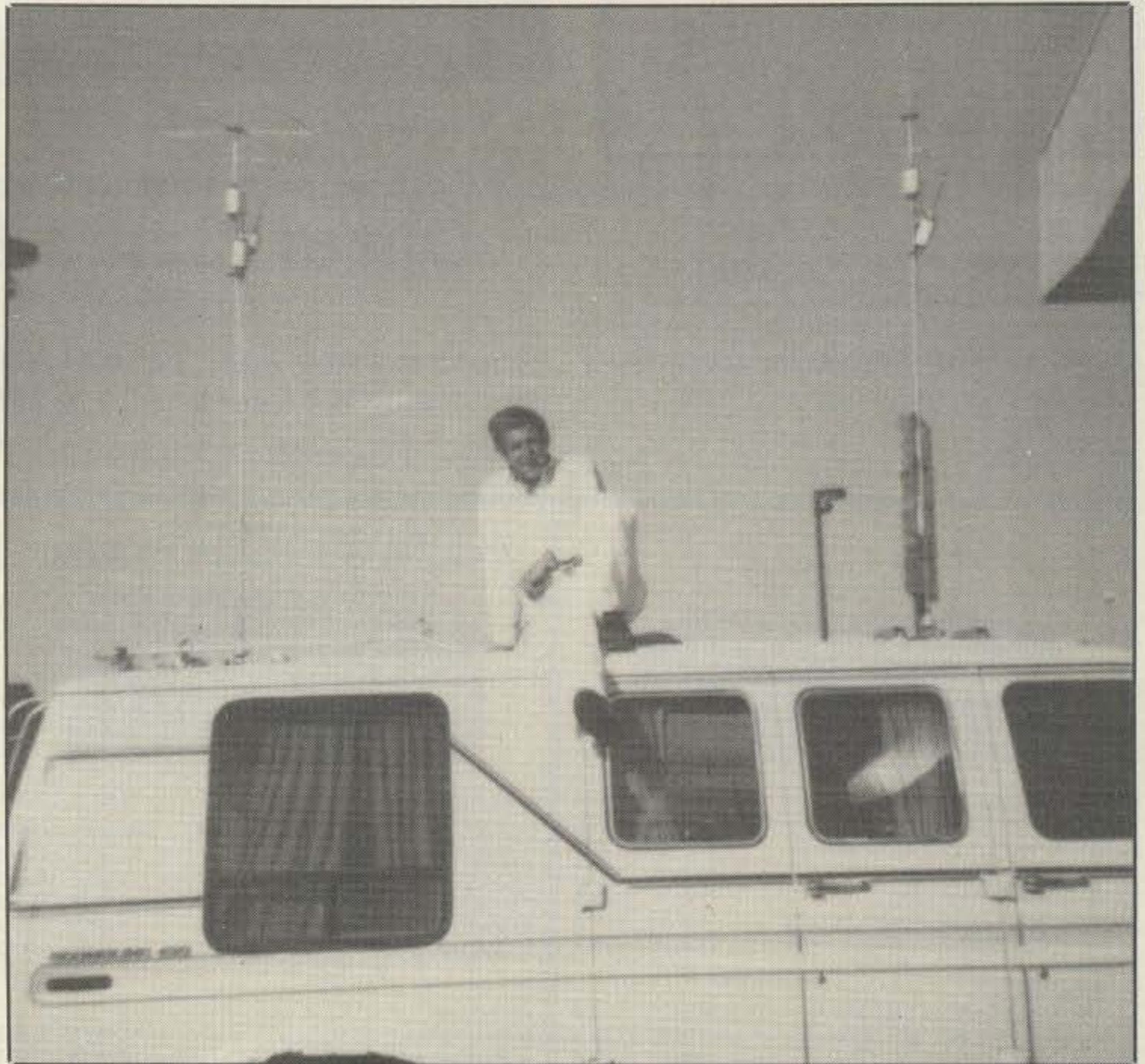
Photo 1— Sy, N4KEL, with his big-signal mobile. Setup runs a KW to phased verticals, and it is stiff competition for most home stations.
