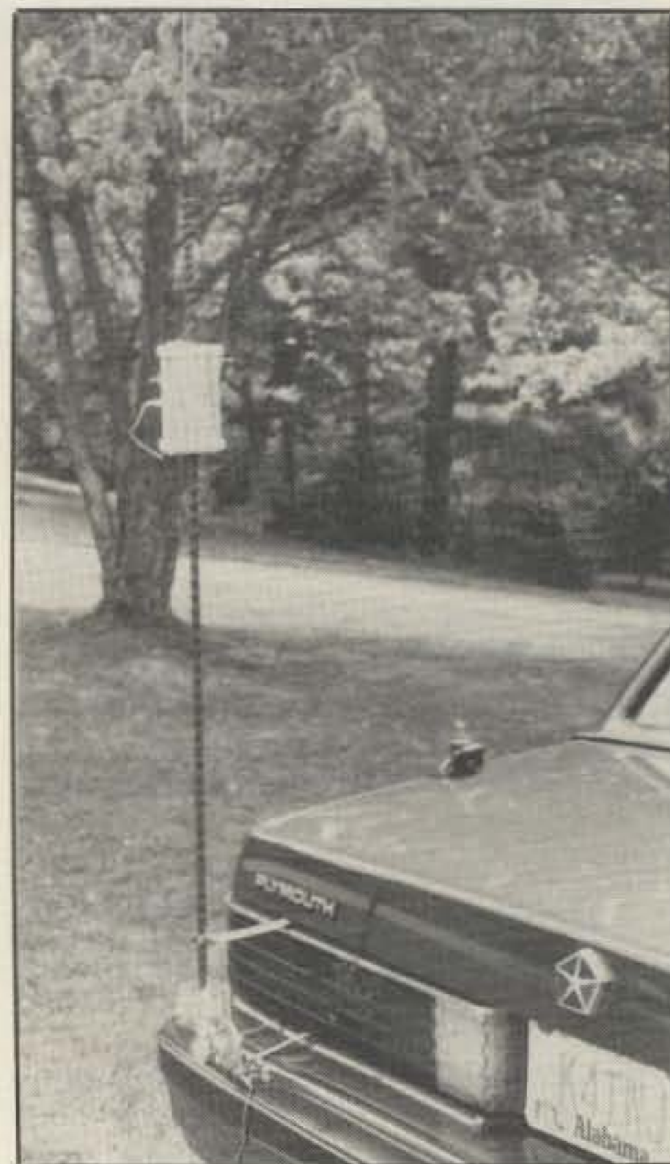
Photo 2- The brand-new Carolina Bug Katcher. Antenna works like a champ, and you can set its taps to favor frequencies on each band. Coil is 3½ inches in diameter and 5½ inches tall. (See text.)
