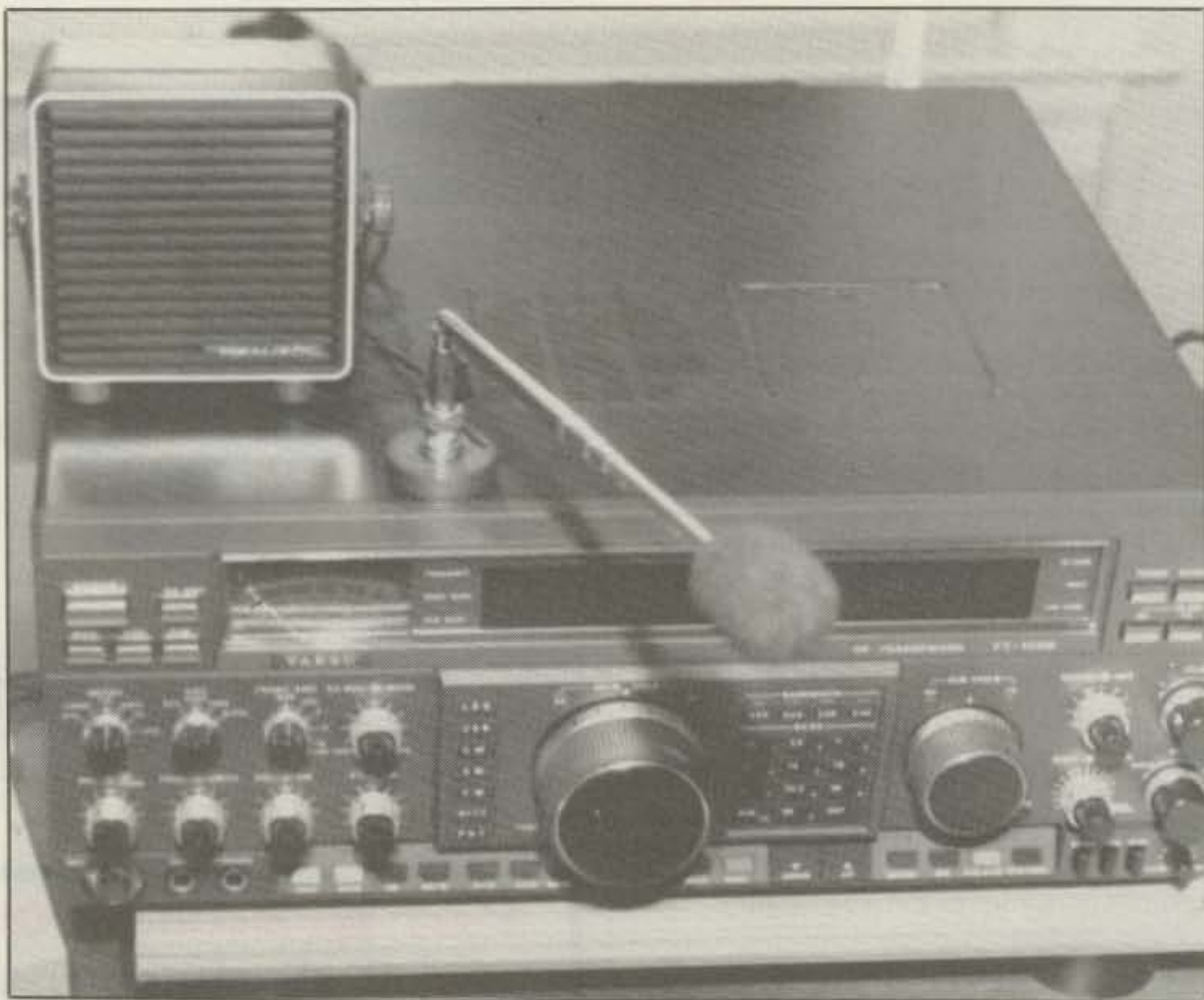
Here's the microphone sitting quite comfortably on top of a transceiver. If the top over on a transceiver were not made of steel, a small steel plate could be mounted on the cover by double-sided tape.
