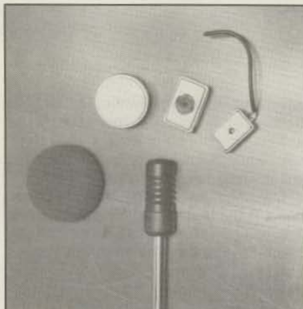
A variety of microphone cartridges can be used to "roll your own" microphone assembly. The only requirement is that the cartridge be held firmly in place and that some form of windscreen be used in front of the cartridge. The round cartridge is a Shure MC-11 and the two cartridges to the right of it are Heil Sound elements.
