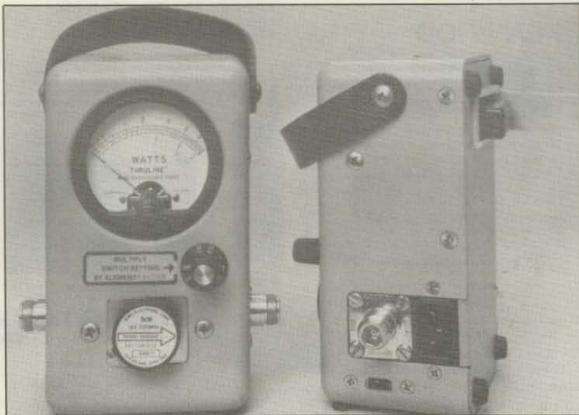
A front and side view of the 4410A. The compartment at the upper rear is for a 9 volt battery. The multiplying factor switch is to the right, between the meter and element.
