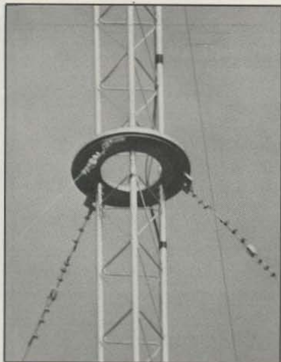
Shown here is the Rotating Tower Systems guy-wire bearing for Rohn 25G towers, installed here at 90 feet. The guy-wire bearing is a three-part assembly that installs as a complete unit and affords a high degree of immunity from ice and snow.
