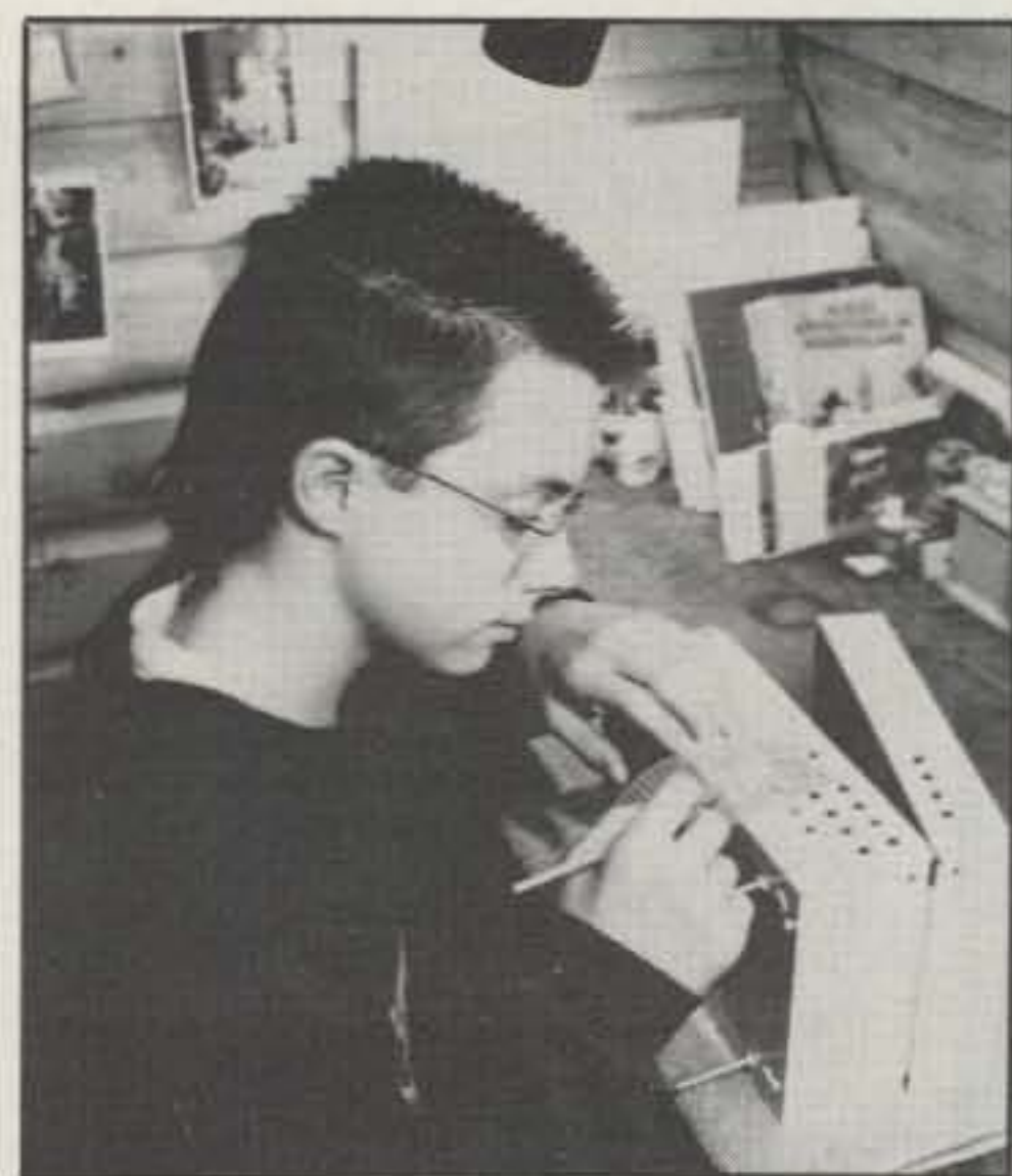
Dan applies rear-panel markings to the 4 x 6 file box "chassis" of the transceiver unit with rub-on lettering.
