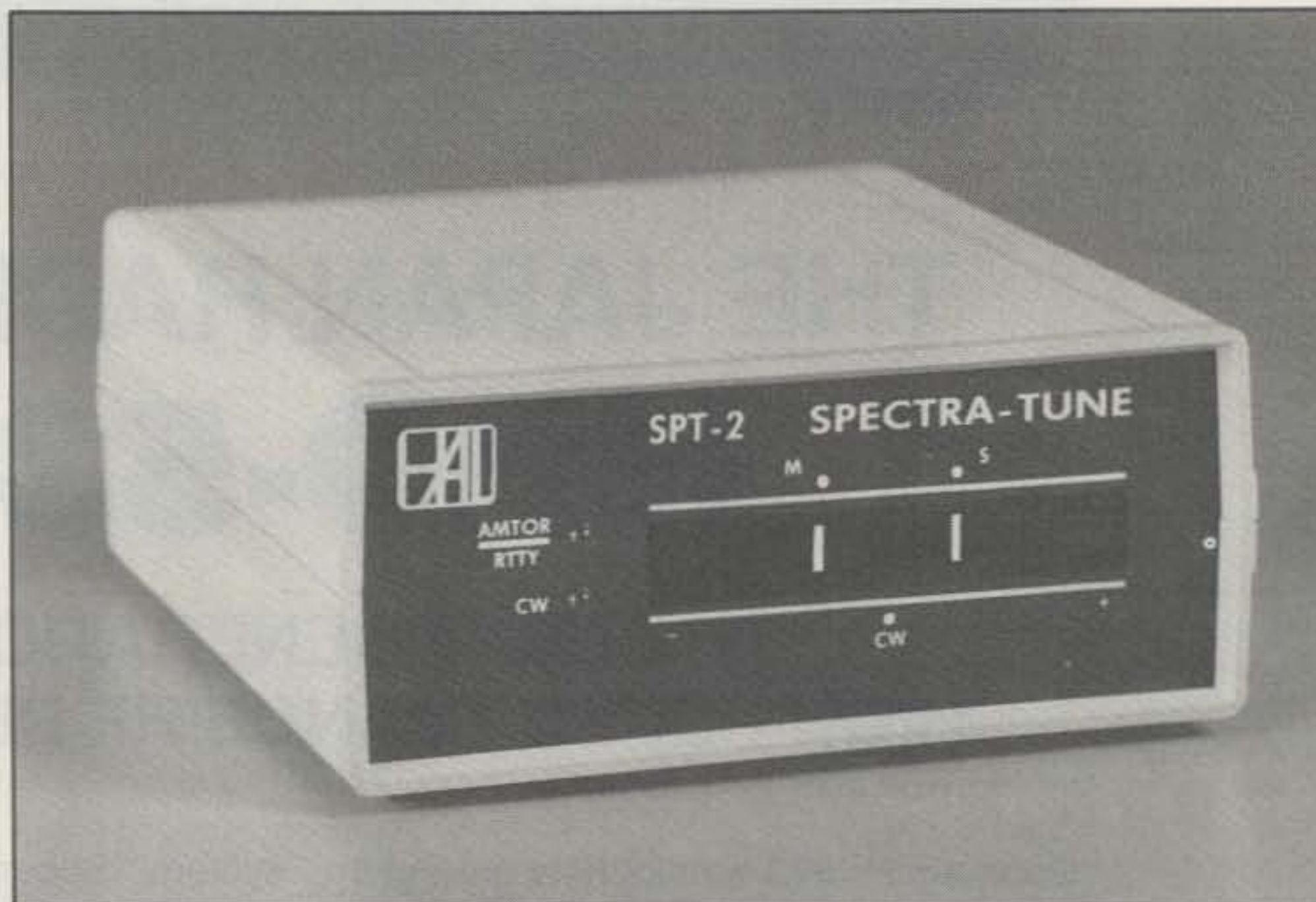
Here is a shot of the bar LED tuning unit.
