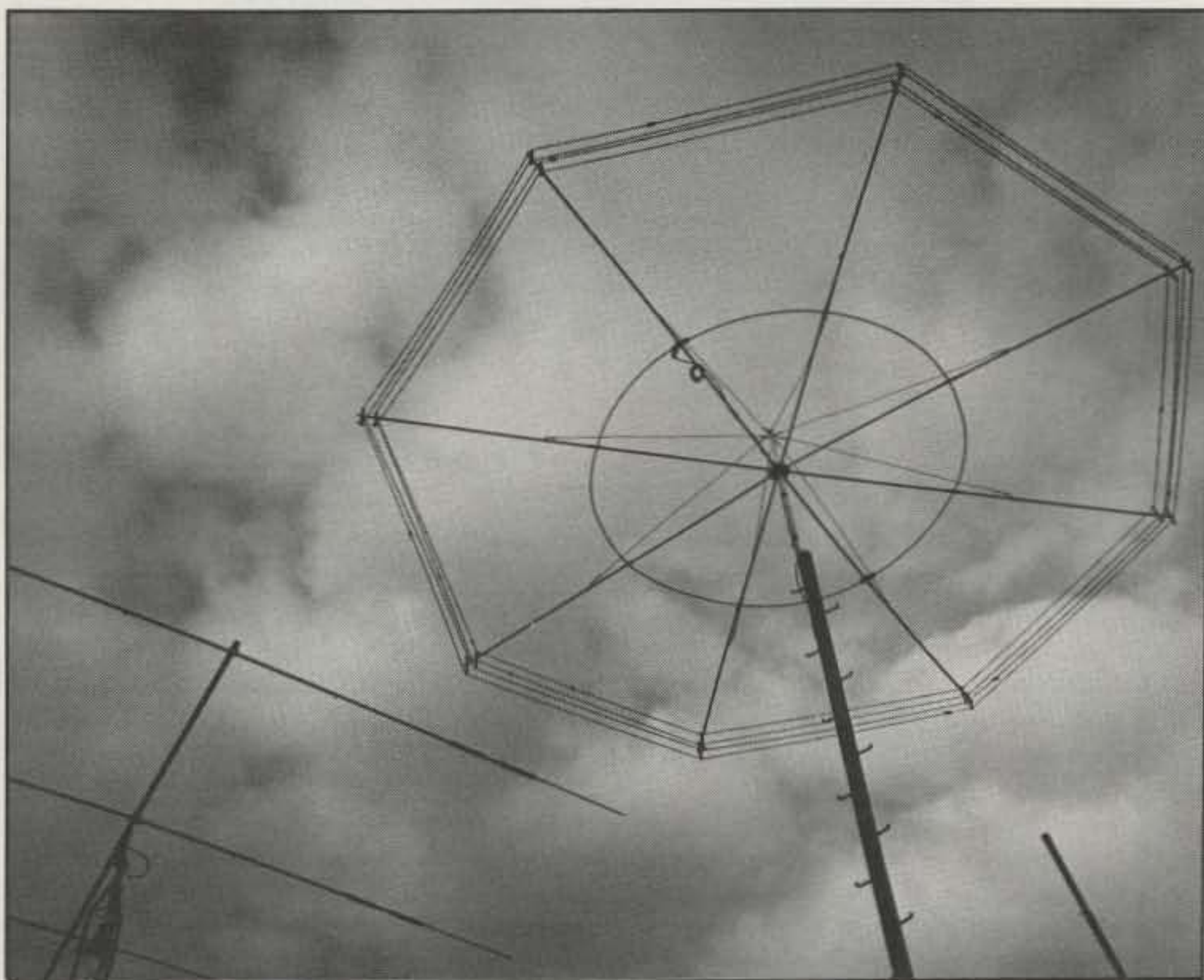
The overall size may tend to put some amateurs off the idea of trying a concentric Yagi, especially multi-element arrays. Here we see the original version installed near a conventional tribander.
