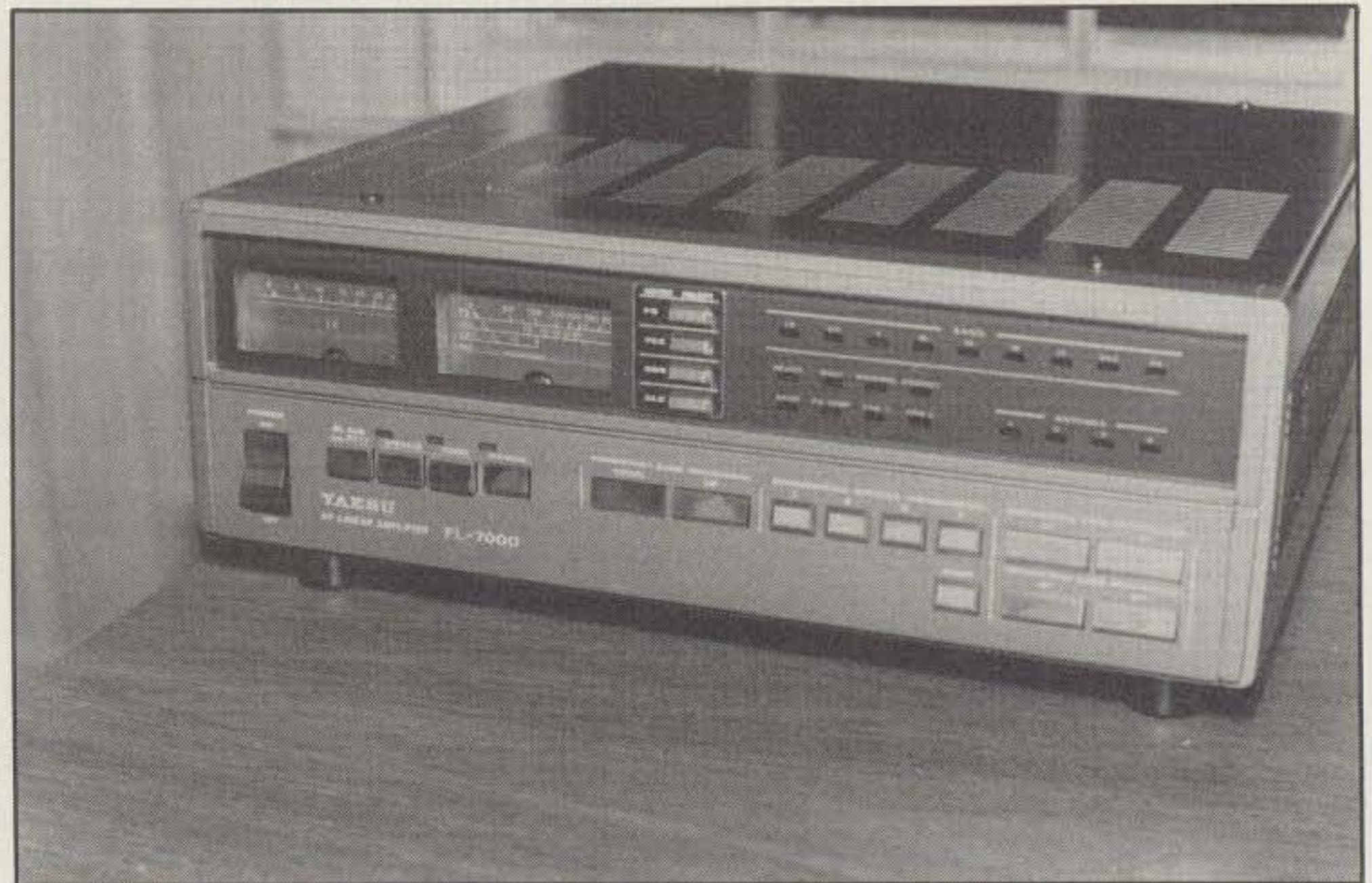
The FL-7000's front panel consists only of various fields of pushbutton controls, LEDs, and two analog meters. If the amplifier is fully set up for automatic operation, only the power on/off switch and the operate/standby switch have to be used.
