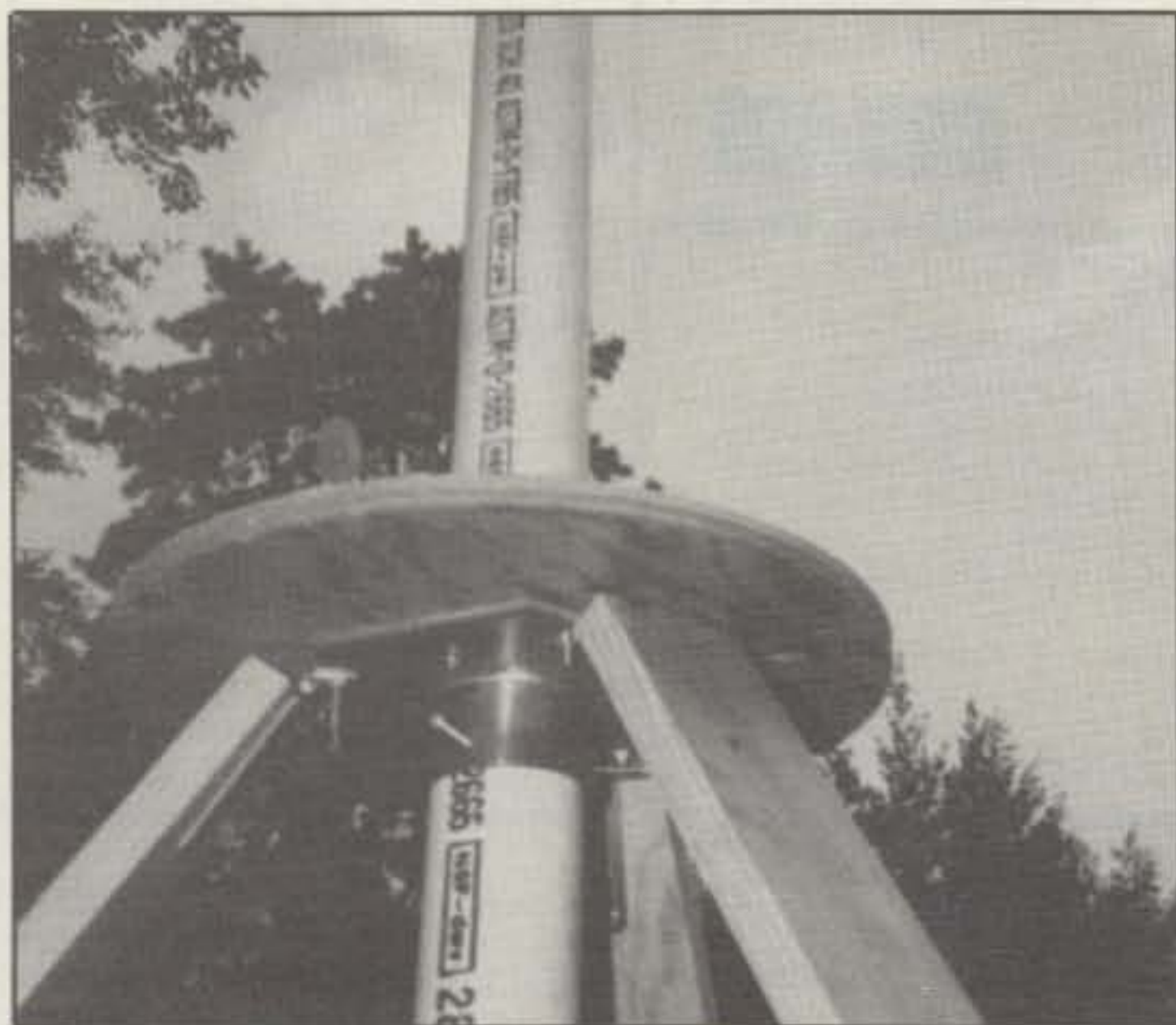
A plywood disc of any convenient dimension makes the top portion of the stand.
